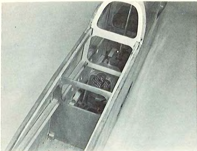
Drive installation as it appears from the cockpit.
