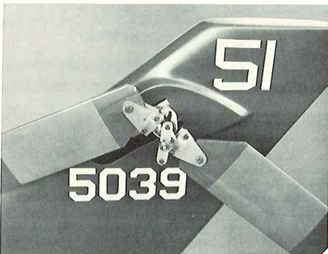
Tail rotor blades must be fitted into the blade holders correctly, allowing the blades to pivot if they should strike the ground.
