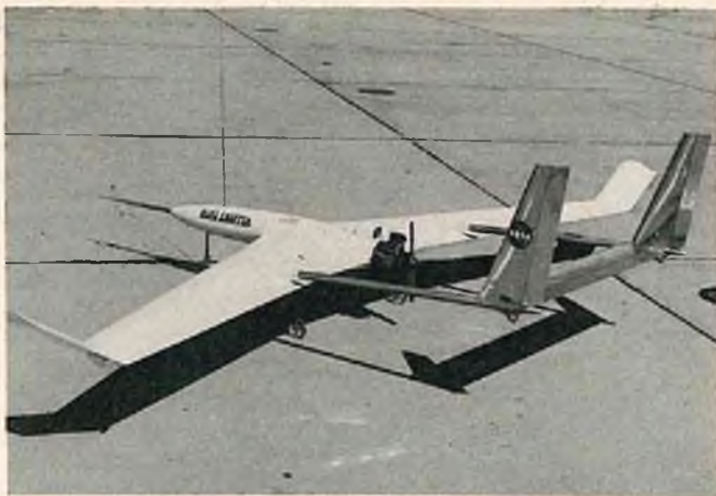
FIGURE 9: Mini-Sniffer aircraft will perform atmospheric pollution sensing up to 100,000 feet altitude.
