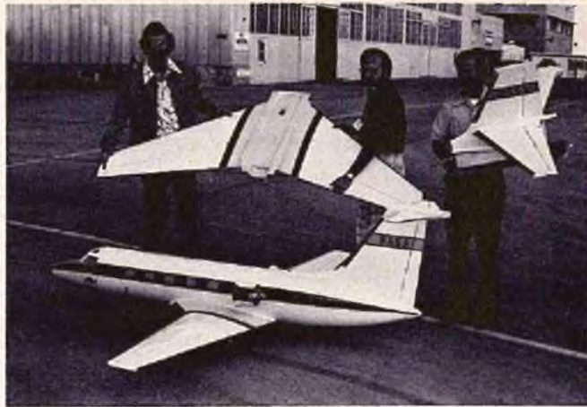
Lockheed Jetstar model is equipped with more efficient NASA designed active control surfaces. Interchangeable scale surfaces are being held.
