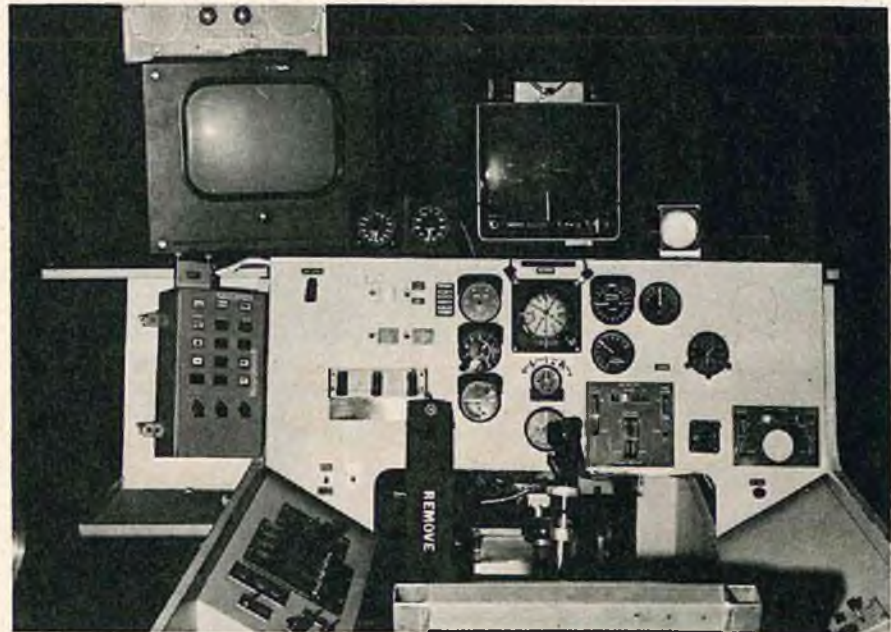
FIGURE 3: Ground cockpit, located inside a building, from which the more sophisticated models are flown!
