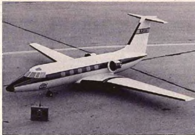
FIGURE 6: ACT-configured Jetstar model has same wing area with ten foot span.
