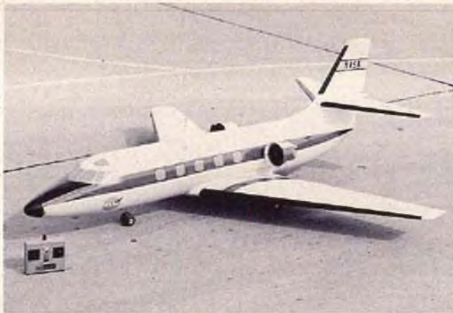
FIGURE 5: Scale Jetstar model with eight foot wingspan weighs 33 pounds.
