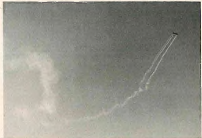
FIGURE 12: Vortex cancelling 30 feet behind model.
