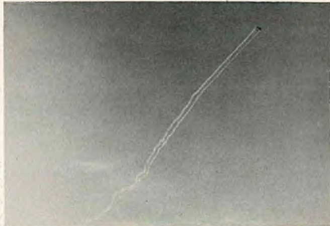
FIGURE 11: Trailing vortex, approximately 2500 feet long.
