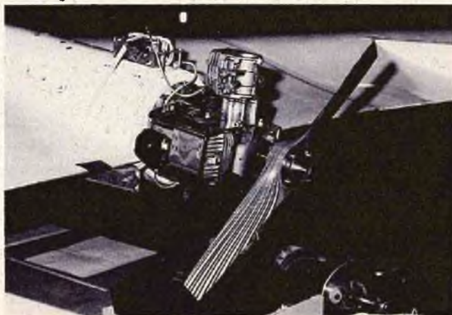
This engine installation has flown Mini-Sniffer to 20,000 ft. altitude.
