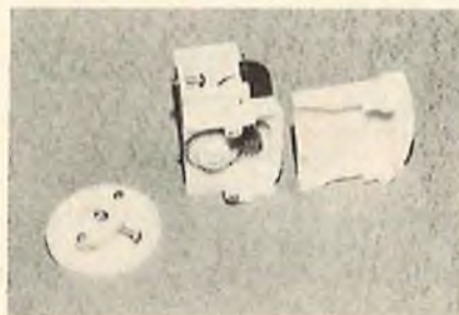
Drive motor in saddle mount and plastic motor base with top half cut away; gear secured to axle by set screw.
