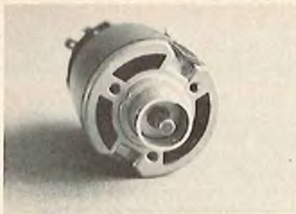
Inner tube of coupling end. Water jacket glued in place over boss on end plate.
