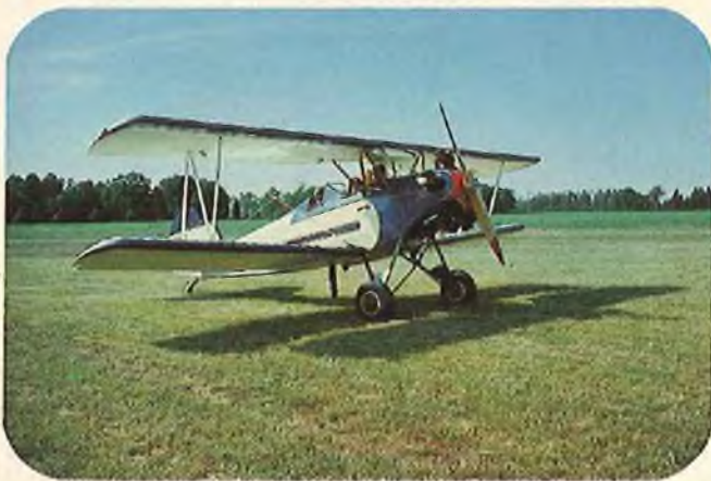
Fleet Biplane is a symphony of struts, wires, and fabric. No starter, even on this big radial, just "prop and hope".
