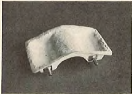
Underneath of hollow motor mount, showing where cooling water will flow. Note the inlet and outlet tubes.
