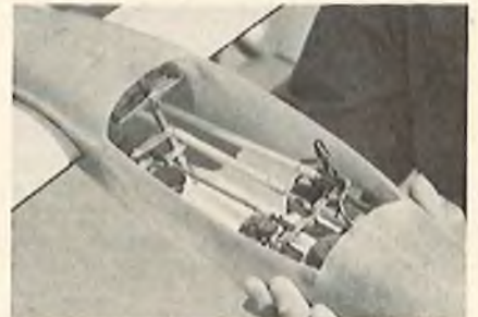
Blaine Rawdon's pivoting mechanism for rotating wings.
