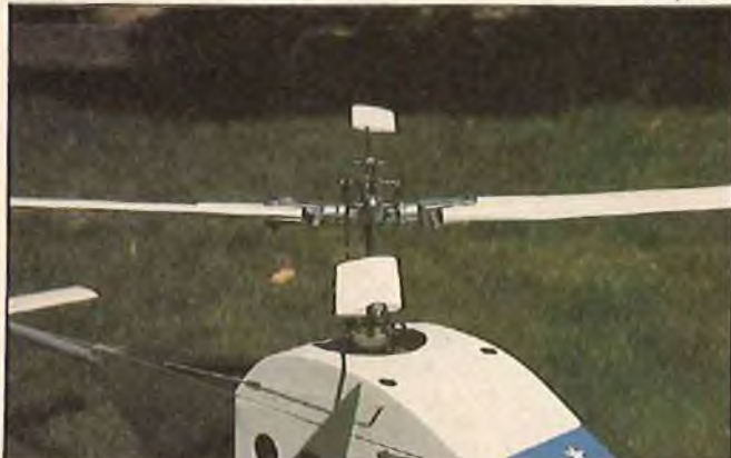
End view of control rotor showing the +8°paddle rigging.
