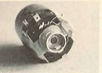
Brush plate end w/jacket tube in place; again with pre-drilled holes.
