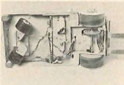
Bottom of truck with wheels in full turn. (R) Resistor in top center of truck for slow speed.
