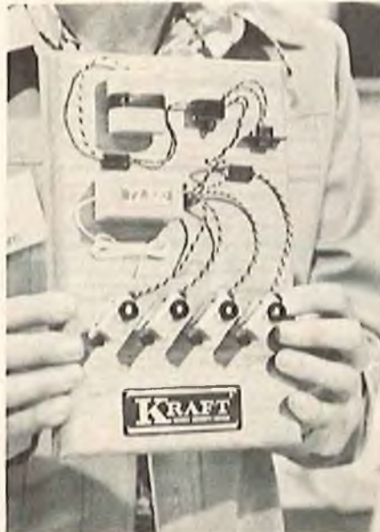
Kraft KPS-18 servos give full house control at 5 1/2 ounces.
