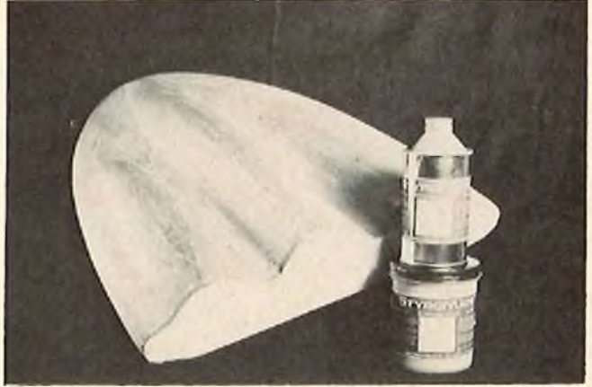
The entire hull cut from the end of a foam paddle board and prepped with StyroMate.
