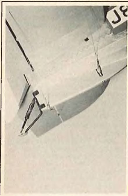
View of functional tail skid and horizontal stabilizer wire brace attachments.
