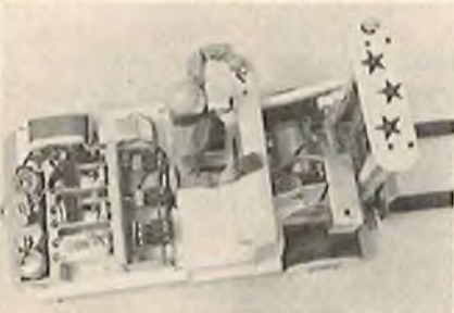
Top view of Senior Truck. Controller system in neutral; nicad batteries in rear; receiver, batteries on side.
