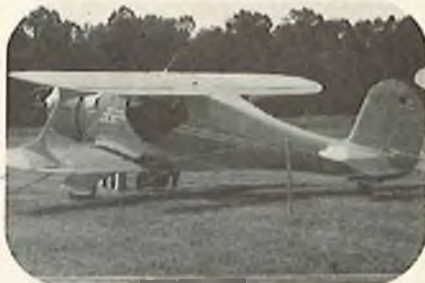
Staggerwing Beech, with top wing set aft of bottom wing, is a beautiful scale subject.
