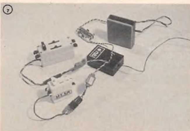
(1) R1, R2, R3, R4 and R5. (2) PC board with nine discrete components. (3) One half the size of a postage stamp. (4) Completed Buffer Amps. (5) Completed Buffer Amps ready to be placed between receiver and servo. (6) Buffer Amp in use with two different types of servos in parallel, a 3 wire with a 4 wire. (7) System hook-up showing Buffer Amps in use with an older receiver and 3 wire as well as 4 wire servo in use.
