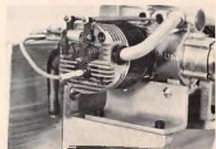
Johnson's spring clip installed on the Damo 4 cycle twin.
