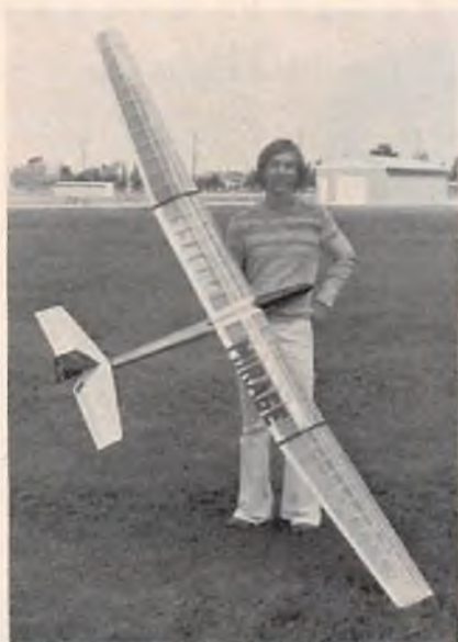
Mike Reagon and his Mirage. Note elevator is hinged on right side only.
