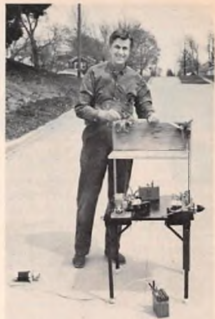
Paul Johnson runs up his Damo. Paul doesn't like to crawl around on the ground when checking out engines so he carries this folding leg collapsible table test stand. On the lower level are an OPS twin in-line and a Gannett 4 cycle.
