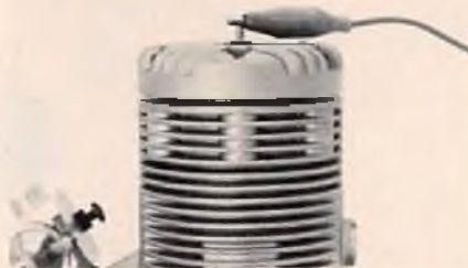
A sub-miniature alligator clip really latches on to the top of a glow plug.
