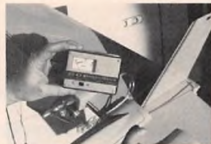
Checking battery voltage under load with a battery tester, S & O shown, can warn you of low battery voltage.
