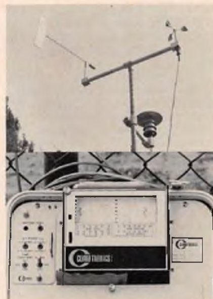
Pacific Soaring Society's weather station. Sensing units are mounted on pole above recorder.
