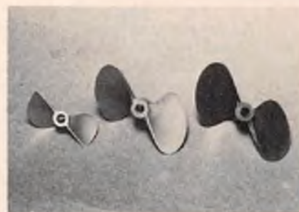
Typical power props; from left to right, a J. Gale C-20 in beryllium bronze; an Octura 1457 in metal, and an Octura 1460 in plastic. All three use a dog-drive system.
