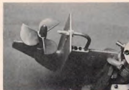
A J. Gale three-bladed prop on the K & B 21 outboard. It has been found that the performance of this motor can be increased by judicious use of props, and tuning them.
