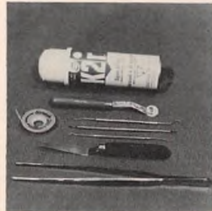
A cap from a can of spot remover keeps the sharp part under control.
