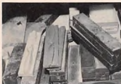
Just a few of Kelly's many male/female molds - he produces these from steel filled epoxy.
