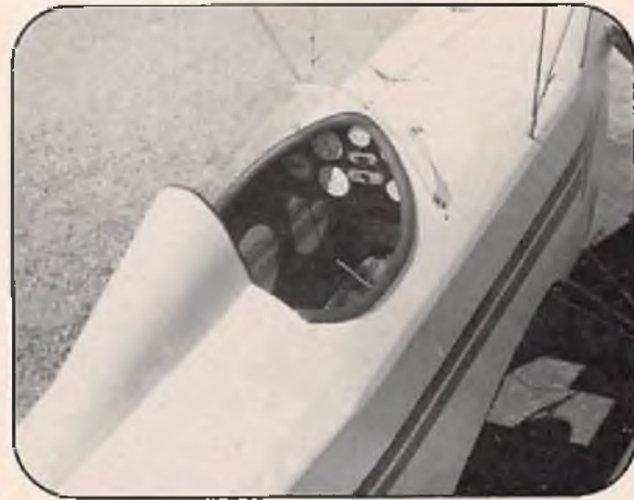
The office. Notice the beefed-up fuselage construction. The small forward projecting stubs on the cabane diagonal braces are lifting points on the C.G. Headrest is 3-ply Strathmore Bristol drawing paper. Coaming padding is windshield wiper vacuum hose Hot Stuffed in place.
