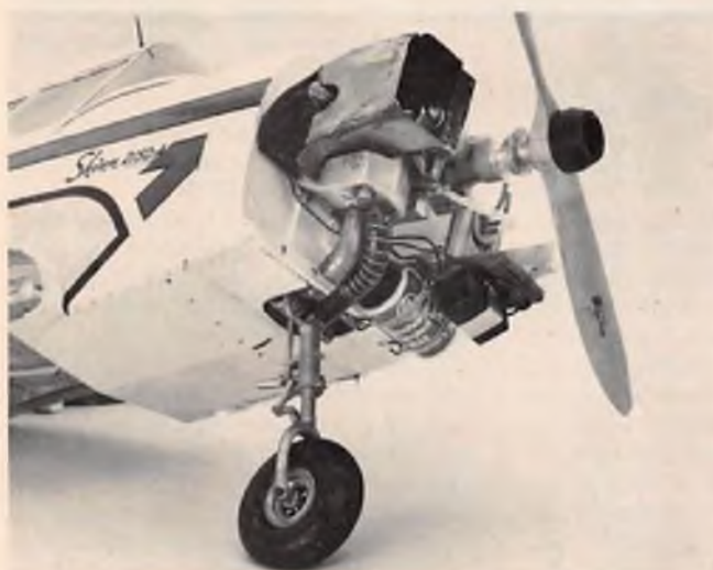
The On-Board installed on Shinn 2150-A. The square duct over the engine helps prevent over-heating when the cowl is on. All of the air entering the cowl is directed through the head fins of the Webra .61.
