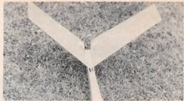
Even the control linkage is up out of the grass, but they may be run under the V-tail.
