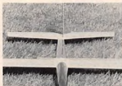
Head on of Mirage showing offset vertical fin and flat wing center section.
