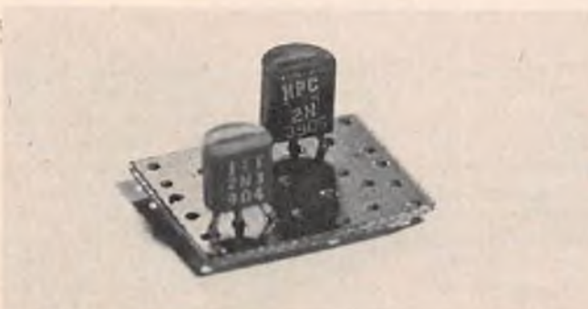
Q1 and Q2 in place.
