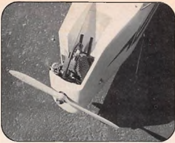
The Quadra's nest, showing twin 1/2" stacks brazed to muffler, and part of the aluminum anti-ignition interference shield. Probably unnecessary, but why take a chance?
