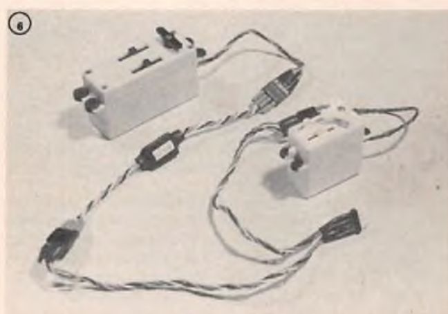
(1) R1, R2, R3, R4 and R5. (2) PC board with nine discrete components. (3) One half the size of a postage stamp. (4) Completed Buffer Amps. (5) Completed Buffer Amps ready to be placed between receiver and servo. (6) Buffer Amp in use with two different types of servos in parallel, a 3 wire with a 4 wire. (7) System hook-up showing Buffer Amps in use with an older receiver and 3 wire as well as 4 wire servo in use.
