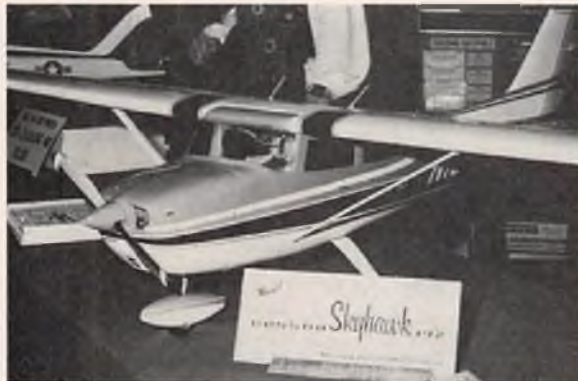
Cessna 172 Skyhawk from Sig Mfg. Co. Plastic fuselage shells, foam wing core, many hardware and scale details. 65" span, .60 engine.
