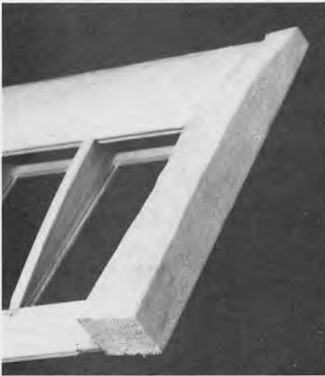
Tip block carved to rough shape, ready for Hoerner upsweep.
