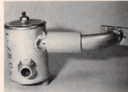
This McCoy pipe manifold gives more horsepower and mounts the muffler forward in front of the LH rear tire. The exhaust exists out the side of the body.
