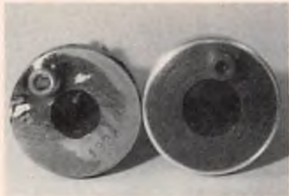
S.T. crank, on the left, compared to McCoy's full circle crank on the right for K & B 21.
