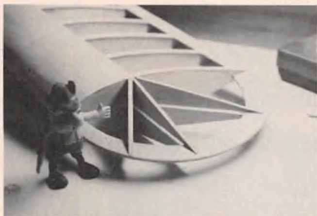
Completed wing tip showing tip braces in place.
