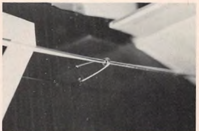
Wire pushrod guide for elevator epoxied into fuselage side.
