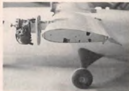
Left wing and Nacelle of Twin Otter. Engines will be on one servo for throttle. Note flap which will operate in prototypical fashion. Model will have ailerons operating as flaperons.
