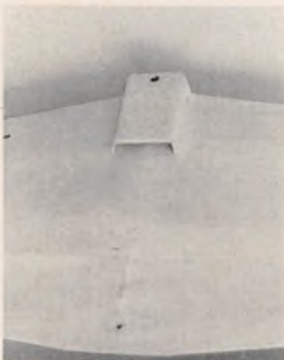
View of partial radiator attached to wing.
