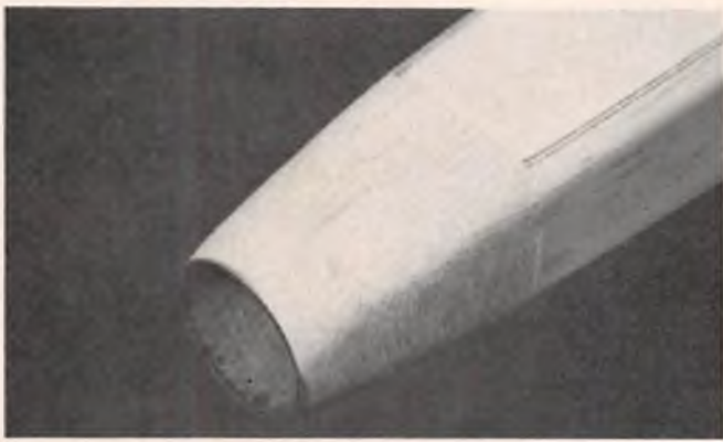
Sand noseblock to within 1/32" of plywood liner.
