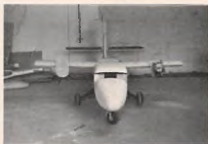
Bill Jaenicke's Twin Otter. Wingspan 12.5 feet, Outer wing panels plug into center section. Fuselage is 9.5 feet in length, all-up weight will be 55 pounds.
