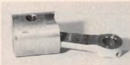
S.T. aluminum piston is conventional with 2 clips holding in piston pin. Rod is fully machined from bar stock and appears to be strong enough to do the job. Lower end is bushed.
