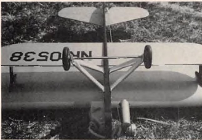
Landing gear installed. Note throttle pushrod at L.E. of wing, left of muffler.
