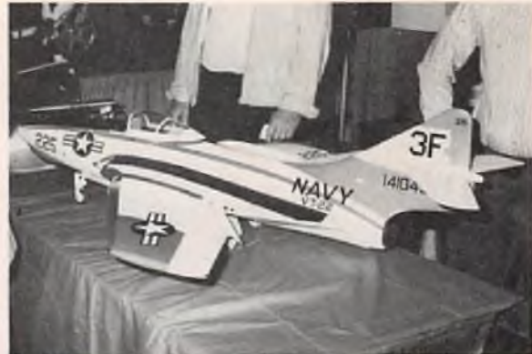
Latest ducted fan from Jet Hangar Hobbies. F9F Cougar for 7.5cc and Turbax I fan unit. Semi kit with epoxy glass fuse, foam wing.
