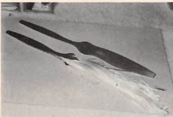
Kelly Products, P.O. Box 38, Western Springs, IL 60558, showed the internal construction of its fibreglass filled props.
