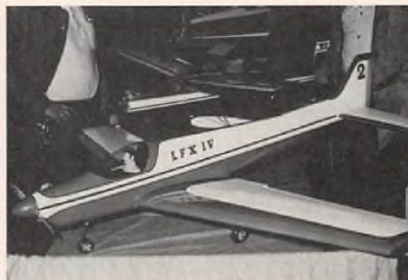
LFX IV , a high performance pattern plane for AMA or FAI maneuvers. 62½" wingspan, fiberglass and foam, ply covering. Johnnie Casburn Mfg. Co.
