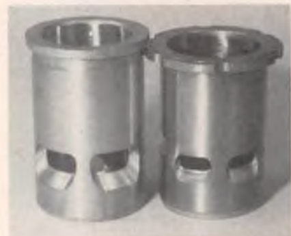
Transfer ports in the S.T. sleeve, on the left, are almost twice as big as the K & B ports.
