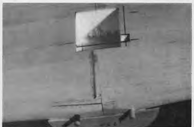
Top view of wing shows nyrod route for cable. Groove was later filled with micro-balloons before painting.
