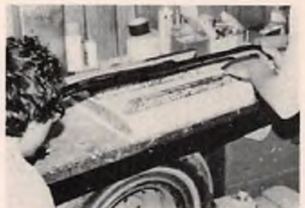
Cutting the cores. Bars on top of foam billet are steel and hold any movement or warp out of foam billet. Wheel under counter is for car, not large model.
