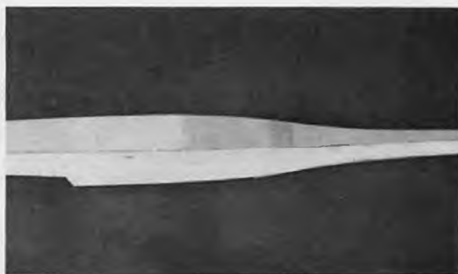
Cross grain bottom sheeting installed.
