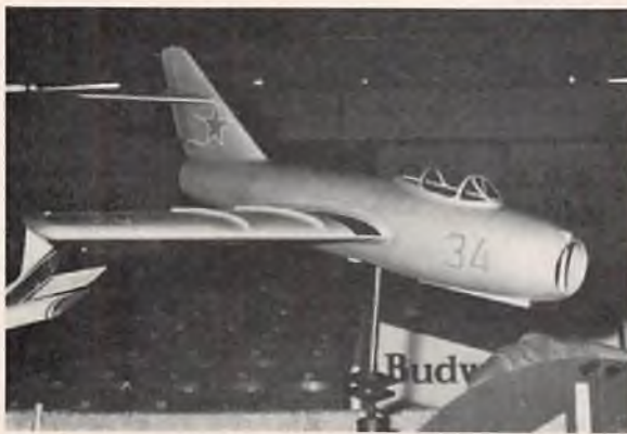
57" wingspan, .60 ducted fan Mig-15 by Byron Originals. Kit includes fiberglass fuselage, molded wing and tail, fan unit, less engine.
