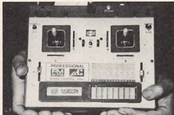
New Aristocraft import, 8 channel Werner R/C system with many programmable functions including reversing, travel rate . . .
