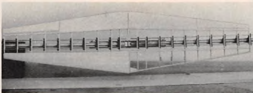
A-Justo-Jig is sure way of building a straight wing.
