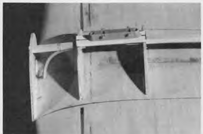
The release mechanism in place --- very scale like. Vortac also provides additional mounting clamps with the release mechanism in case you want to mount something else. We used one for an auxiliary fuel tank which is attached for static display.
