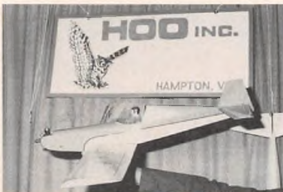
SB-2 Scout , 1/2A sport trainer for two channel R/C, 19 to 25 oz., 36½" span, 226 sq. in. area. Hoo Inc. 12 Mac Alva Dr., Hampton, VA 23669.
