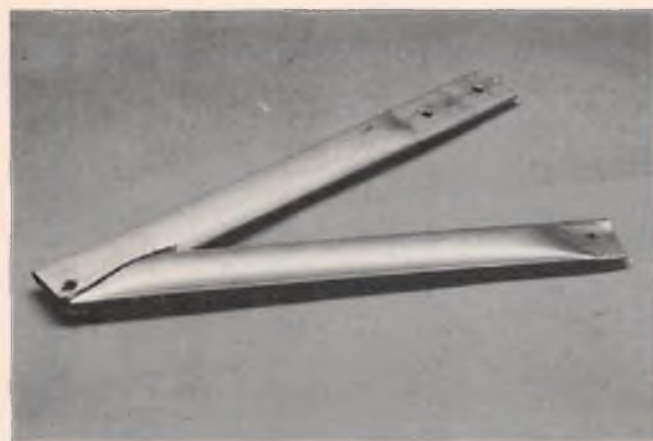
Landing gear struts assembled and ends flattened.
