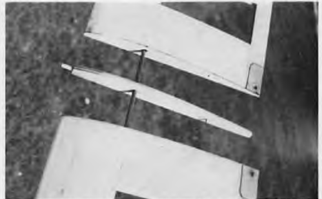
Wing joiner detail. Note rear alignment pin and front locating dowel.
