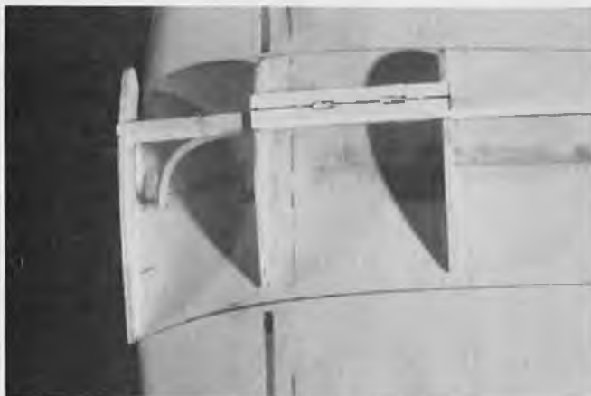
A small plywood mount provides all the support required for the release mechanism. An inner nyrod serves to route a fish leader or nylon cable to the drop servo.
