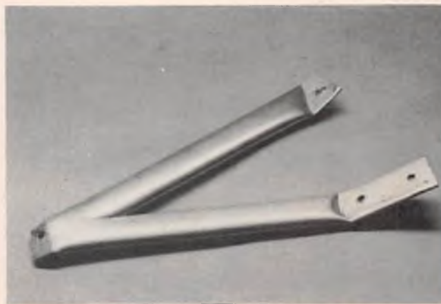
Final bends and landing gear is ready to install.
