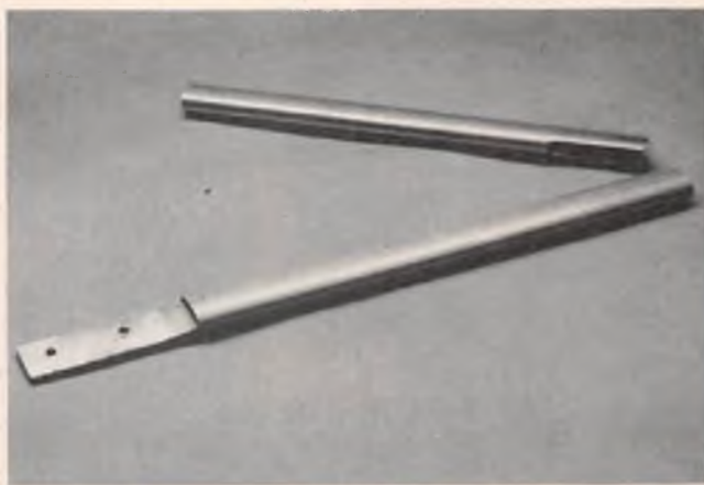
Landing gear struts made from 5/8" streamline aluminum tubing. Bottom strut shows 1/16" x 1/2" hard aluminum fitted inside tubing.
