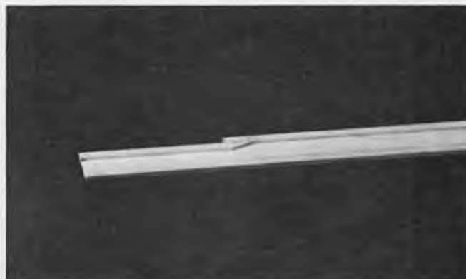
Fuselage tail detail showing longeron installation.
