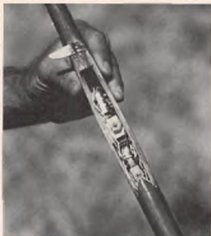
"Innards" of Dave Thornburg's R-C hand launch. Servo's and receiver fit close, see text. Finger rest matches with wing trailing edge. Threaded nylon block is wing hold-down.
