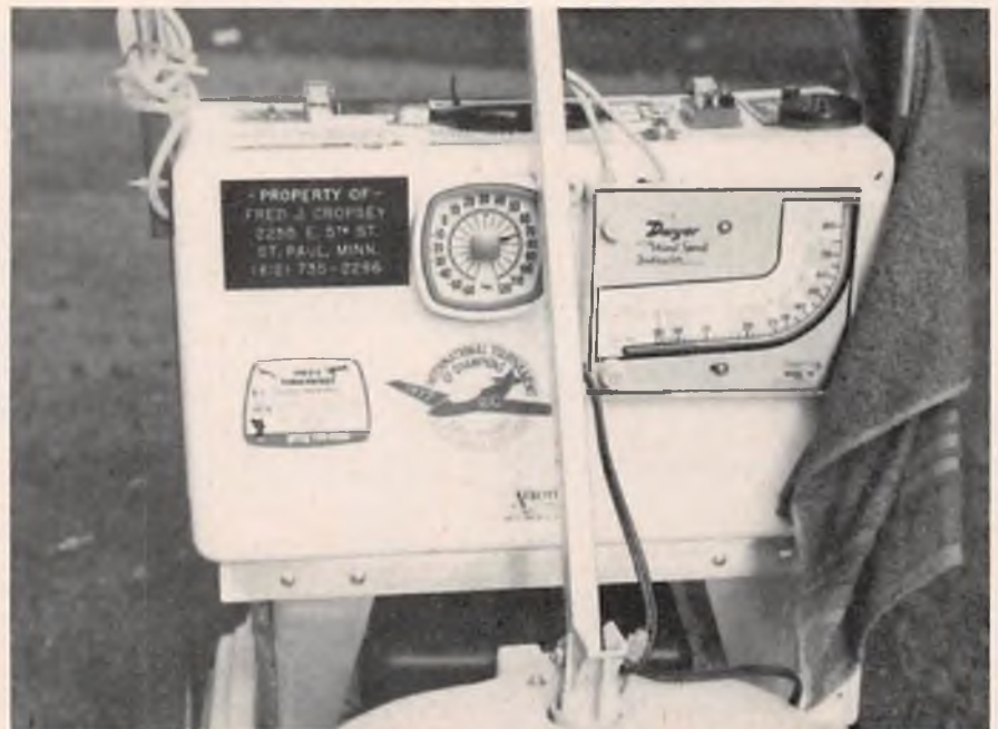
Front view showing thermometer, wind speed indicator and motivating handle. Note aluminum stand that supports Flyin' Box.
