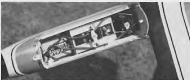
Radio installation. Sliding tray for rudder servo. Wing locating dowel comes thru bulkhead to secure rear of canopy.
