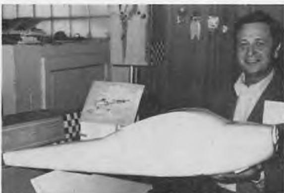
Fiberglass fuse for Cessna 182; one of a number of glass or plastic and foam imports. Avionics Int'l., 403 Clagett Dr., Rockville, MD.
