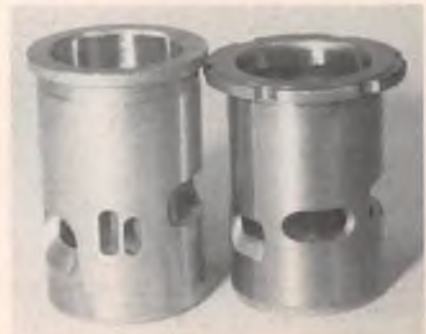
S.T. sleeve on the left and K & B on the right showing the 2 PDP ports in the S.T. sleeve which are approx. 1/2 the size of the K & B ports.
