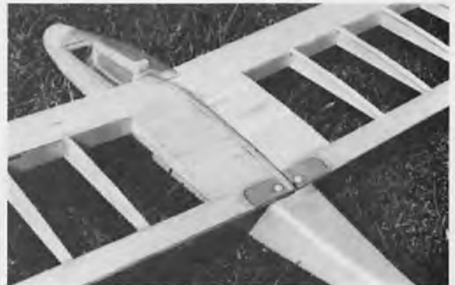
Rear wing hold-down bolt detail.
