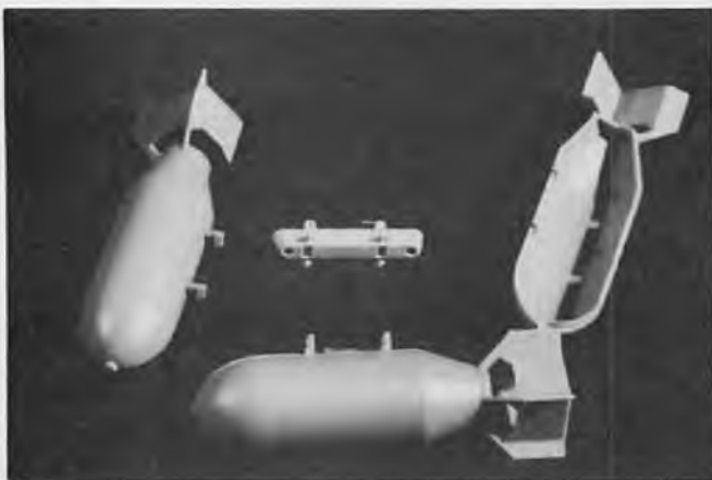
The release mechanism is shown together with one assembled and one "exploded" bomb. Charcoal or chalk dust make a great filler for the "explosion" on impact. The molded nylon bomb is nearly indestructible.
