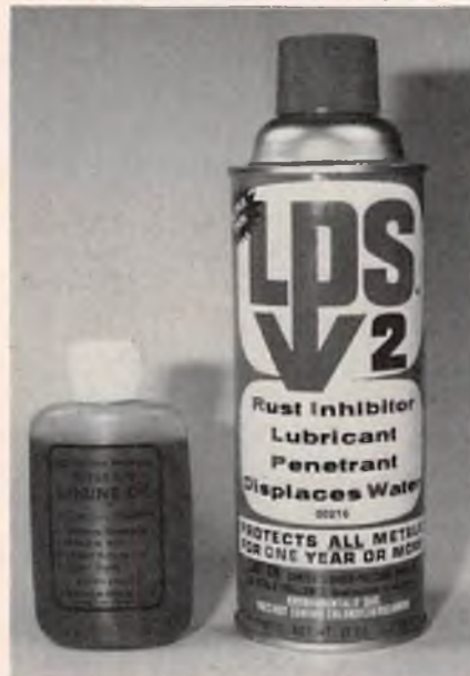
Two good products you should know of are Prather Products, "After Run Engine Oil," on the left, and LPS #2. Prevents gumming & rust; longer engine life and easier starts. If you're not going to be running the engine for awhile, remove the glow plug, back cover and air filter and flush engine out with LPS #2 (not #1 or #3 or WD40). Oil the critical parts with Prather oil. Available at your hobby shop and the LPS #2 from your hardware store.
