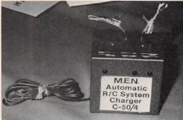
New automatic nicad charger from MEN. Adjusts rate from normal to trickle, as required. Claimed to extend cell life.
