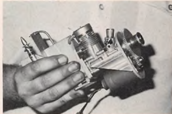
One of many electric starter units for glow engines, this one on K & B outboard. Eastcraft Specialty, 709 Longboat, Beachwood, NJ 08722.
