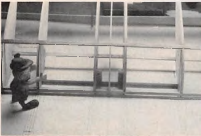
Install 1/64" plywood half ribs as shown.
