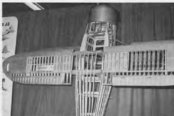
Quarter Scale Stagger Wing Beech D-17S from Model Engineering of Norwalk. 96" span, 20 lbs. Aluminum cowling, plywood/balsa, 2700 sq.
