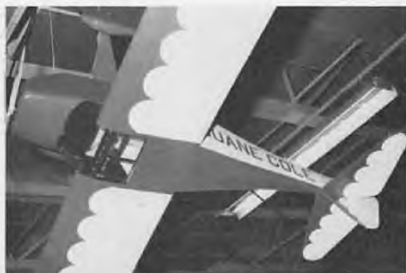
Clipped wing version of the popular Taylorcraft, in Quarter Scale. 88" wingspan with a flying weight of 18 to 22 lbs. NAME, Inc.
