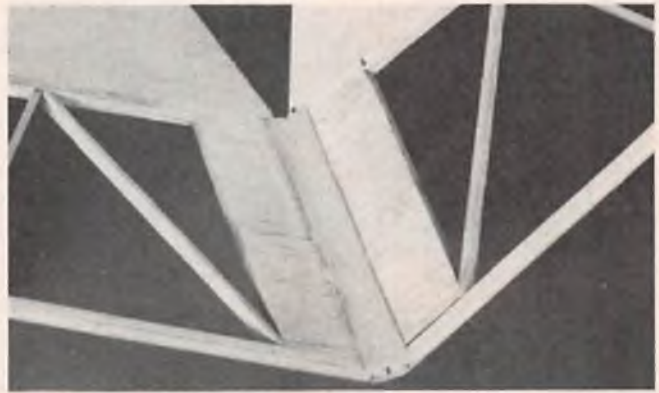
Triangular joiner strip is sanded to concave cross-section.
