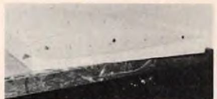
Wing pattern made from formica or similar material. Sands well and hot wire slides on its surface easily. Patterns are also long lasting.
