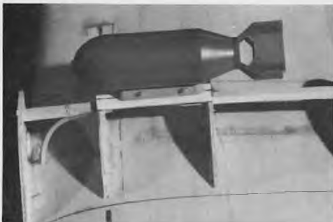
Test for binding before closing in. After testing we removed the unit and cable. After completing the model there was no difficulty in threading the cable and attaching.
