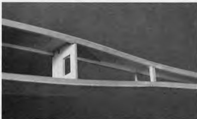
Fuselage detail showing bulkhead and cross brace. Note notch for NyRod tubing.
