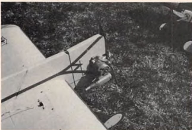
Switch and antenna wire protrude thru hatch cover. Note throttle pushrod at L.E. of wing.
