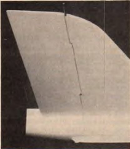
Rudder and fin with hinge pin partially installed.
