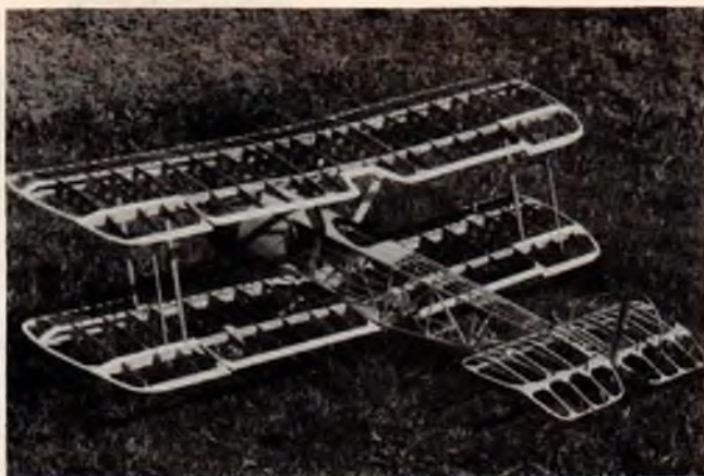
Three-quarter rear view of "Pup." Photo shows prototype with symmetrical stab. Was later changed to a flat stab for better performance.
