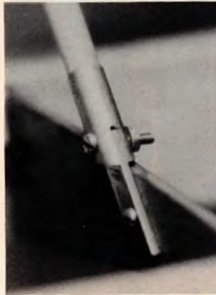
Adjustable alleron pushrod detail. See text.
