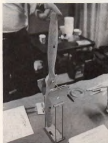
High Point Products has long legs for their balancer to accommodate large diameter props.
