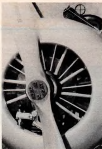
William Bros. 3" Gnome cylinders hide most of the engine inside the cowl.
