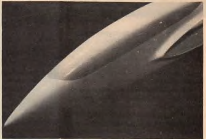
Nose section showing canopy trim and wing fillet.
