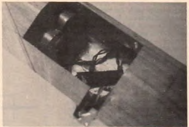
Battery compartment. Foam packing removed for clarity.
