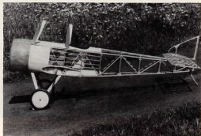
Completed fuselage ready for covering. This is when things get exciting.
