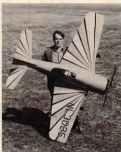
Nick Ziroll's latest addition to his plan sets in this F8F Bearcat shown in racing colors. Span is 86" and both canopy and fiberglass cowl are available.
