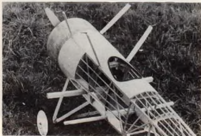
Note the plug-in spars for removing the lower wings for transporting aircraft.
