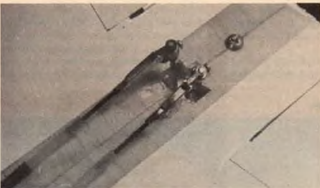
Elevon linkage and screw to secure bottom fuselage to wing.
