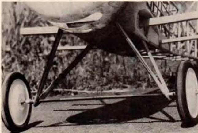
Close-up of landing gear detail. Good view of plug-ins for lower wings.
