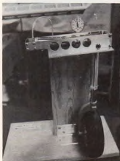
Annco Mfg. displayed possibly the strongest, neatest set of retracts for large scale aircraft ever. Shock absorbing.
