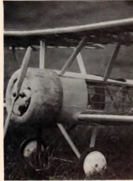
Fiberglass cowl makes the completed nose section just like the full-size one.
