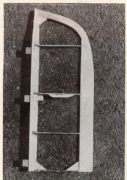
Close-up of aileron. Note the hinges are secured by small dowels.
