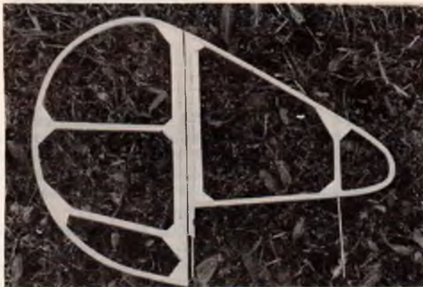
Completed fin and rudder. Fin tailpost now runs to bottom of fuselage.
