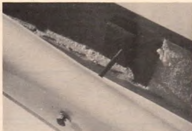
Long screw pulls top and bottom fuselage snugly against wing.
