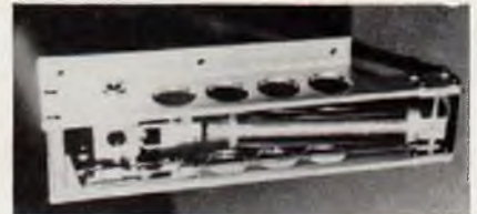
Annco Manufacturing will be producing this good looking retract gear for Quarter Scale at what could be very attractive prices. Gear is air operated, positive locking and beautifully machined.
