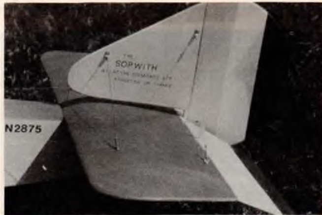
Fin lettering is made up from Zip-A-Tone Follo Light No's 16, 20 and 36 point. Fuselage numbers are Helvetica Medium 48 point (1/2").
