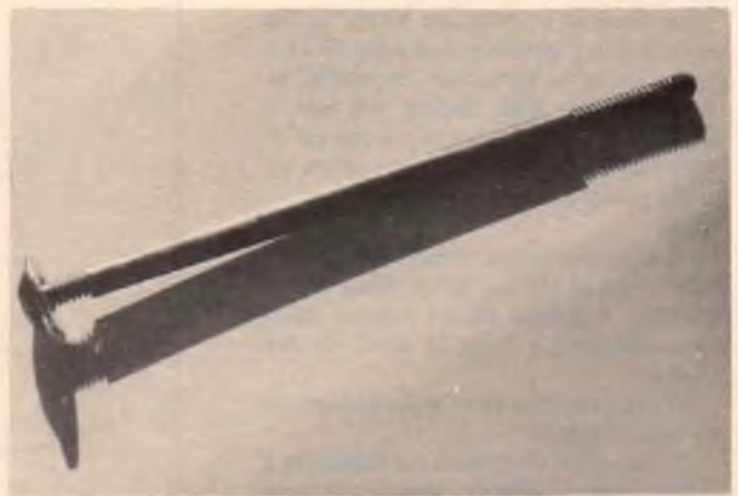
Long screw was made from book binder screw and post.
