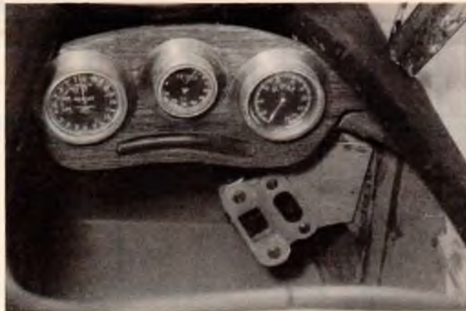
Instrument panel looks like the real thing. Note switch & charging plug located on panel.
