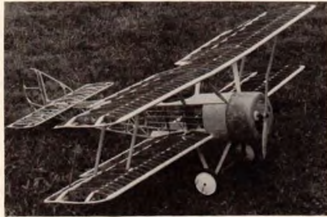
Three-quarter front view of framed up "Pup". Looks too good to cover with fabric.
