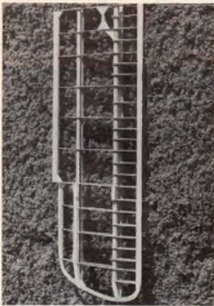
Lower wing panel completed. Wing tips are also laminated strips.
