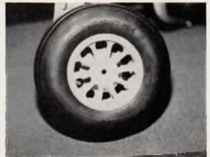
P-51 type wheels and tires for Annco's new retract system will also be available. Wheel is machined and aluminum, wheel is very secure and tire will not come off it is claimed.
