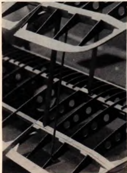
Strut attachment and alleron pushrod tie between wings.
