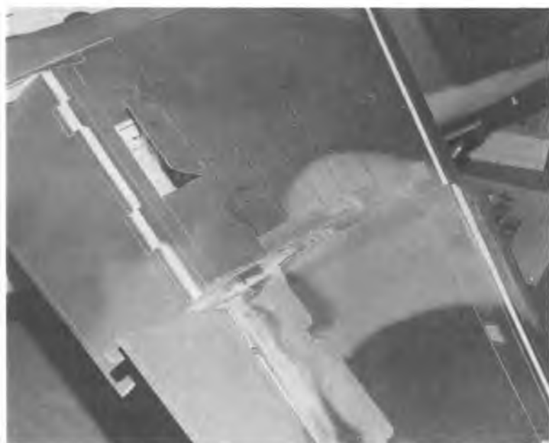
Just forward of the flap is spoiler that opens only on up alleron. Kit for this A-7 attack aircraft is coming from "Jet Hangar Hobbies."
