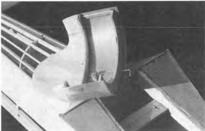
Top cowl half showing locking mechanism.
