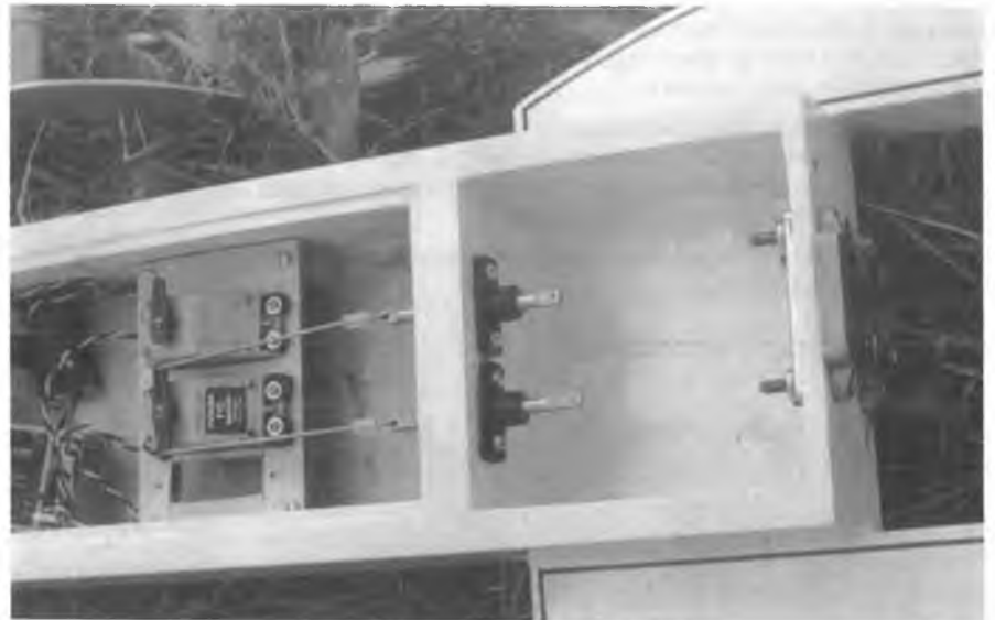
7. Typical pushrod seal mounting system for outboards.
