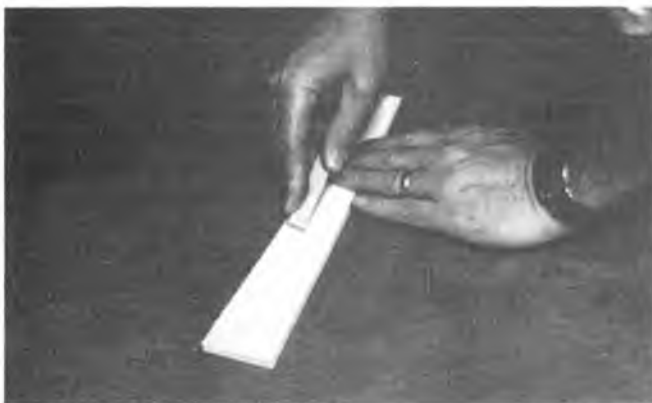
Having cut through one surface to form hinge, crease this cut into surface with a square corner of wood.
