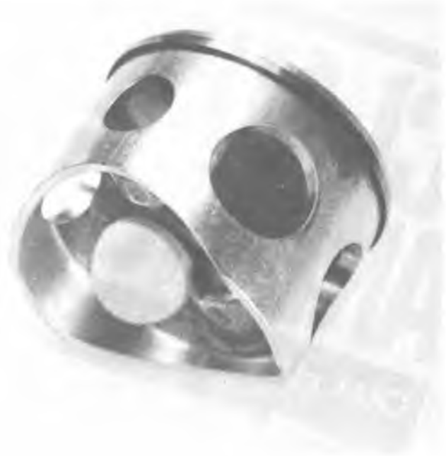
Piston weight has been reduced to the minimum.
