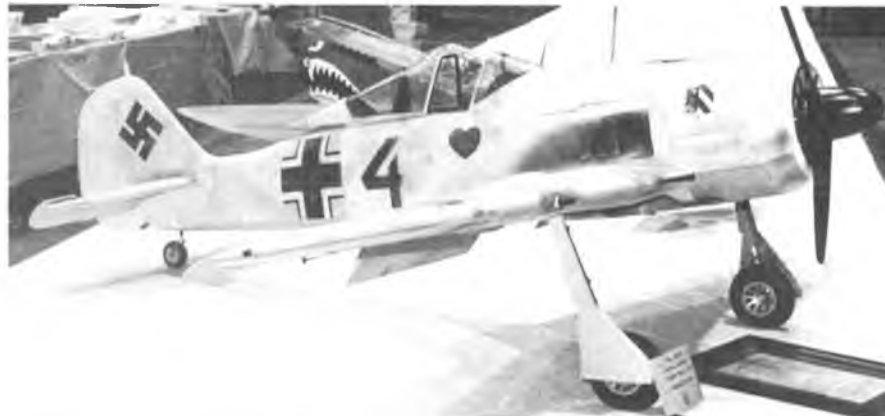
Melvin Nypiuk's scratch-built FW-190A is big. 44 pounds, 108 inch span, Anco retracts and a Chrysler West Bend 5 c.i. engine.
