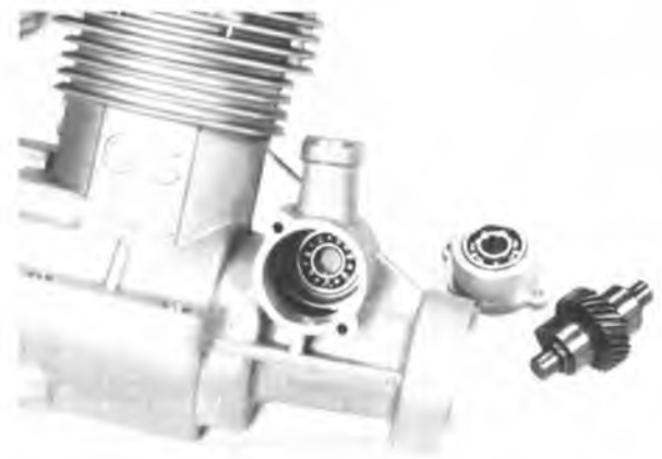
The helix gear driven camshaft is supported on each end by husky ball bearings.
