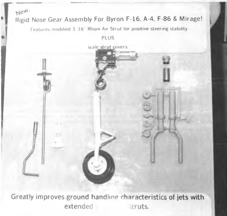
Byron Originals continue to improve features of their existing kit models. In this case it is a scale improvement for retract nose gears.
