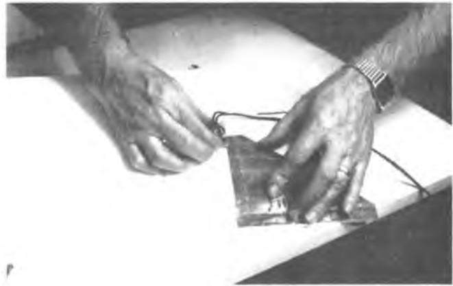
A slot cutter with suitable templates is used to cut the fin slots and aileron linkage slots.
