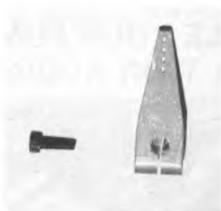
5. Freedom Boats' clamping rudder control arm.
