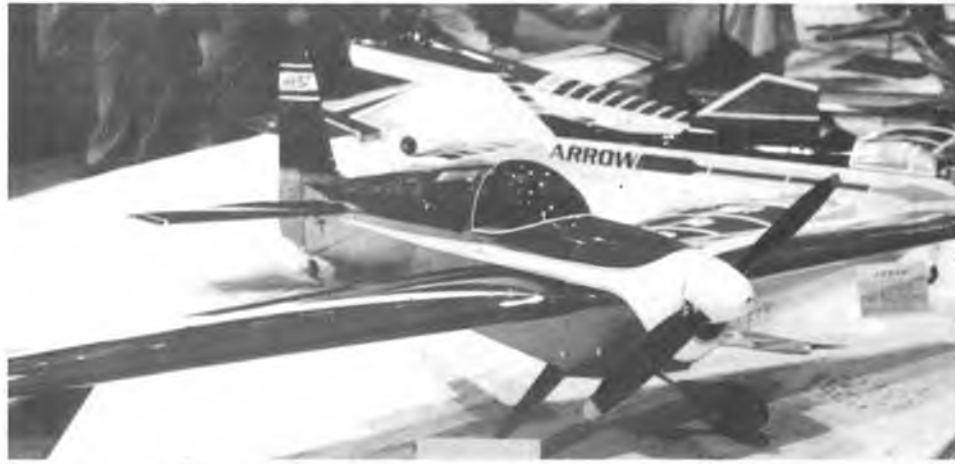
Gerry Graham's "Akrobat II" modification of Laser configuration at 1000 sq. in. It performs well with his 3:1 reduction .60 2 cycle power plant. It is being marketed by Aerobatic Specialties.
