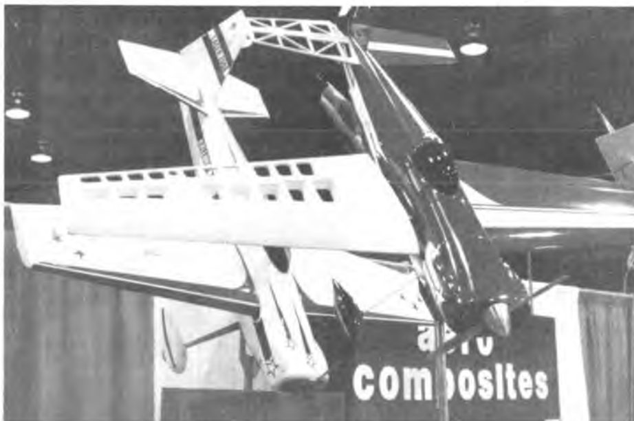
Mallory Models' Laser. Note cut-away wing to save weight. Most of our models are overbuilt.
