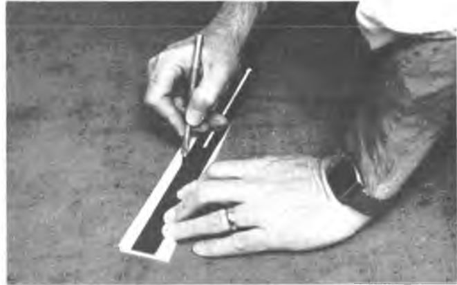
After cutting the "Fome Cor" parts, to form the hinges, cut through one skin of the control surface with a sharp knife as shown.
