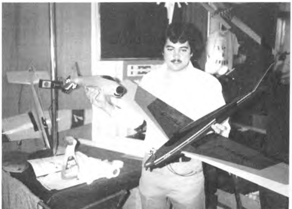
David Verhaeghe of JM Glascraft holds prototype Hummin-Bird. This particular model is glow powered, but the ship is designed for 05 electric systems. Fuselage plug at left shows cooling air inlet for Silent Power.
