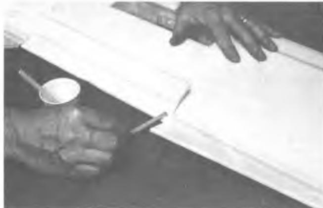
Tape the control surfaces in place as shown, fold back, apply epoxy and tape the surface in the down position until cured.
