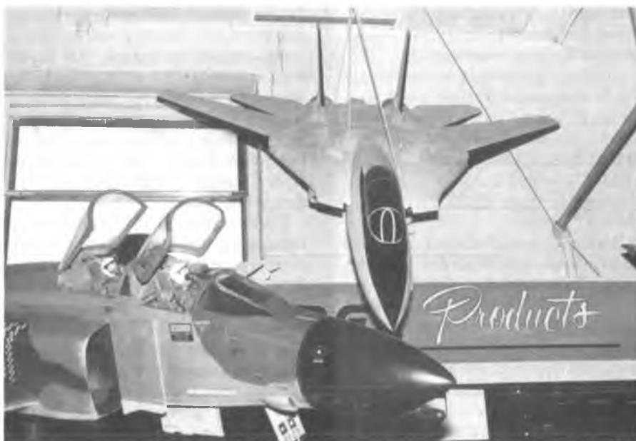
"Jet Model Products" booth with Tom Cook's new F-14 Swing Wing fighter on display. Wing positionable in air, 22 pounds with O.S. Max 65's. Super kit available for Tom's F-4 in foreground.
