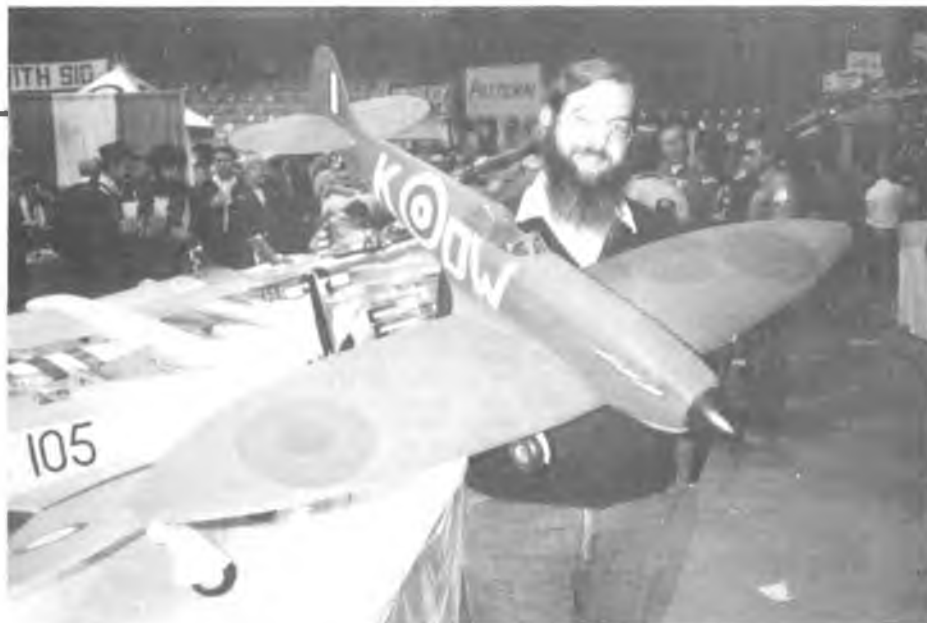
Keith Shaw with Stand-Off Scale Spitfire which utilizes Pilot retracts and Astro 25 geared motor with 16 cells. Bottom side of nose has adequate cooling air intake.
