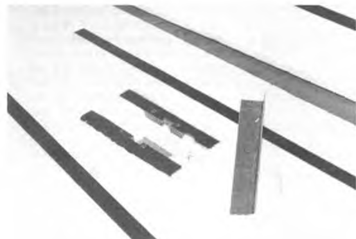
"Bob Violett Models" had great display of carbon fiber applications. This shows Magnalite angle mounts for retracts in foam wing. Lightest and strongest system I have seen.
