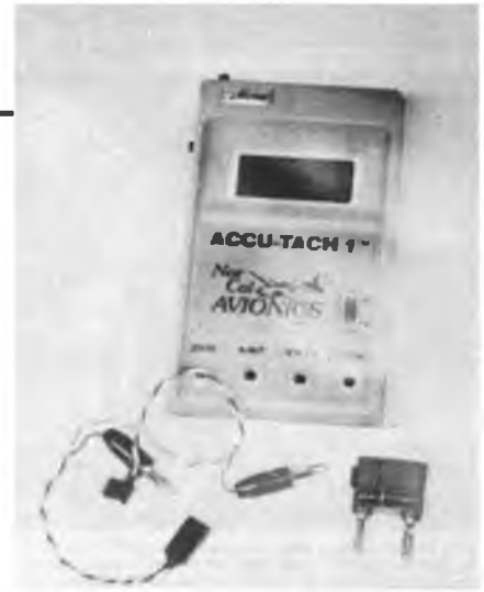
Accu-Tach II by Nor-Cal Avionics, with servo and large battery checkers.
