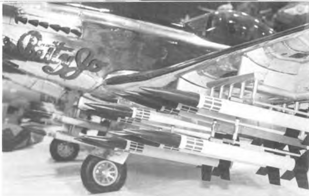
Larry Horbaez' fun-scale P-82 is loaded for bear with Estes rockets that can be fired in air. Not for AMA sanctioned events, the 60 pound model flies with two Kawasaki 3.15 c.i. engines. If you think the Nosen P-51D is big, just hook a couple of them together.
