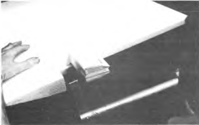
The wing cores are completed by cutting the motor mount reinforcement slots.
