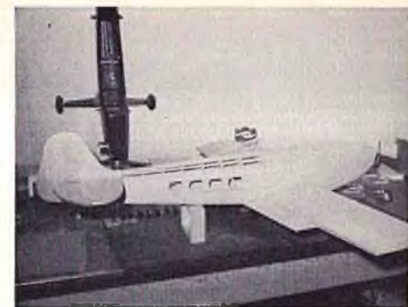
The basic Denight structure prior to covering.
