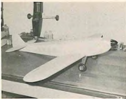
The Denight ready for color dope, cheek cowl, and wheel pants.
