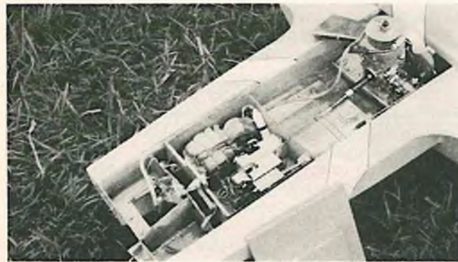
A typical installation — Don Jordan's Super Challenger with TAS engine.
