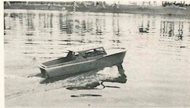
Houston's Frank Traina entered this Corvette hull with hand planked deck. Gannett 4 cycle engine.
