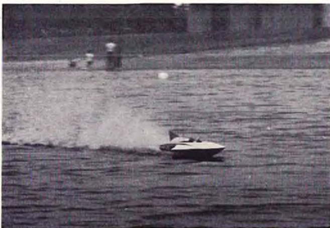
At speed, Jim Henry's Hornet rises up on sponsons and lower half of propeller.
