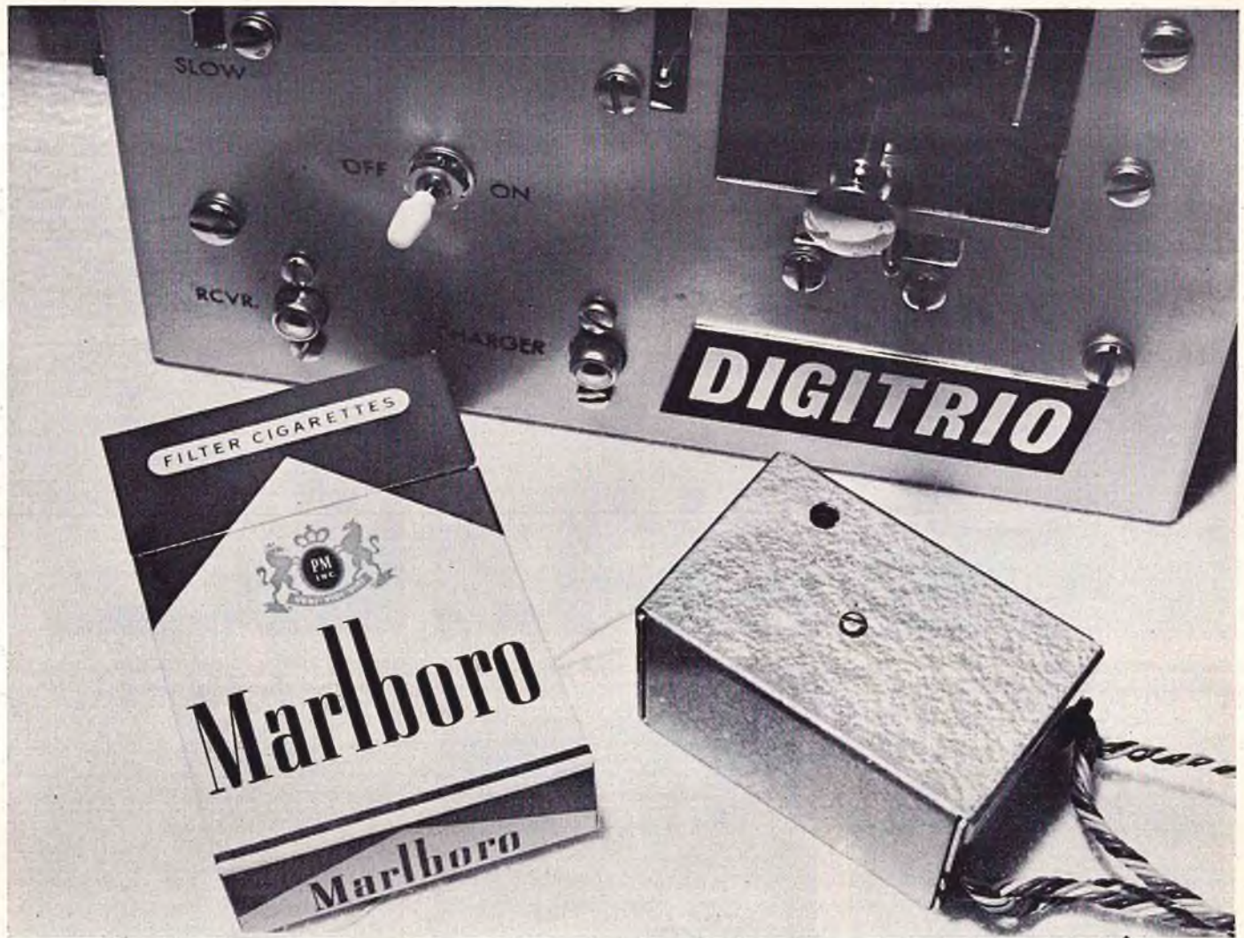
Receiver, decoder unit shown measures 2¼" x 1¾" x 1¾". Together with 3 Controlaire servos and five nicad pencils, entire airborne weight of Digitrio system is 15 ounces. Kraft servos can also be used, as amplifiers will be shown for both units.
