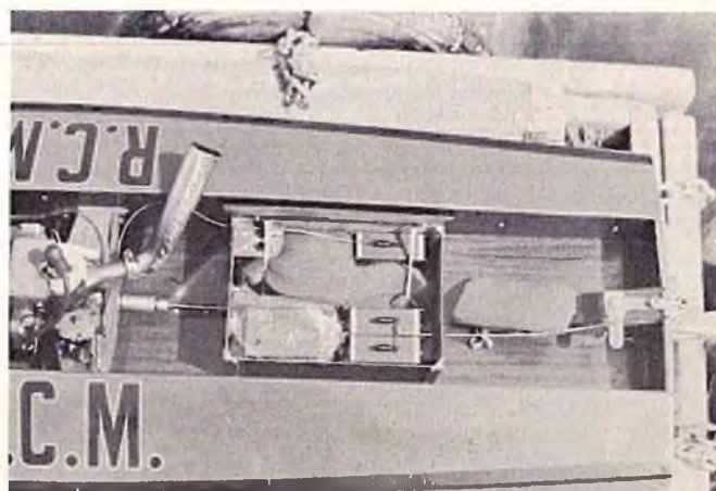
Equipment compartment in the White Heat. Two C & S Proportional servos paralleled to give the needed 8 lbs. of thrust for rudder.
