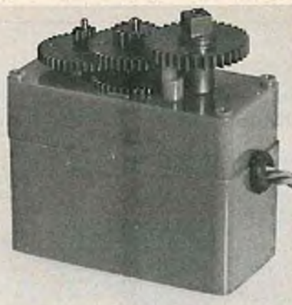
Gear train is Super-Mini servo.
