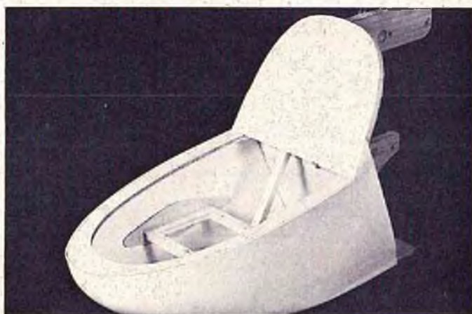
Inside view of fuselage showing servo rails and ply supports... latter contact cemented to ABS fuselage sides.
