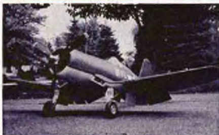
Richard C. Larson 662 Sedgwick Libertyville, Illinois 60048 Built from Royal Gossair Kit, this F4U-1 has a wingspan of 62", weight — 8 1/2 lbs. Super Tiger 71 engine & Kraft Sport radio. Covered with Japanese silk span.
