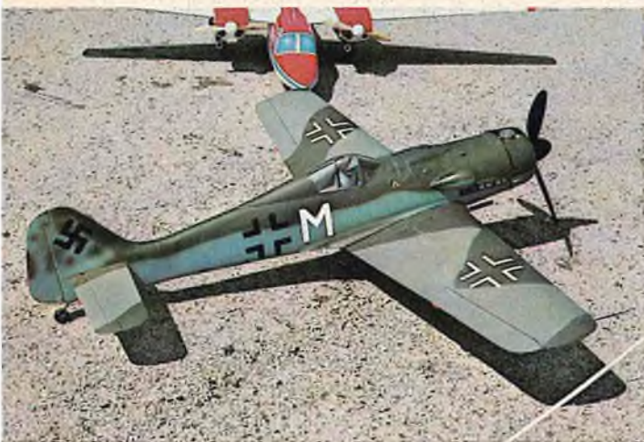
Steve Naber's Fw90D with K & B resin and Aero Gloss dope, OS Max SR .60 with Perry Pump and Rom-Air retracts, Kraft radio.
