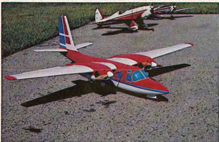
Shrike Commander by Billy Fryman uses two OS Max .60's and Futaba radio.
