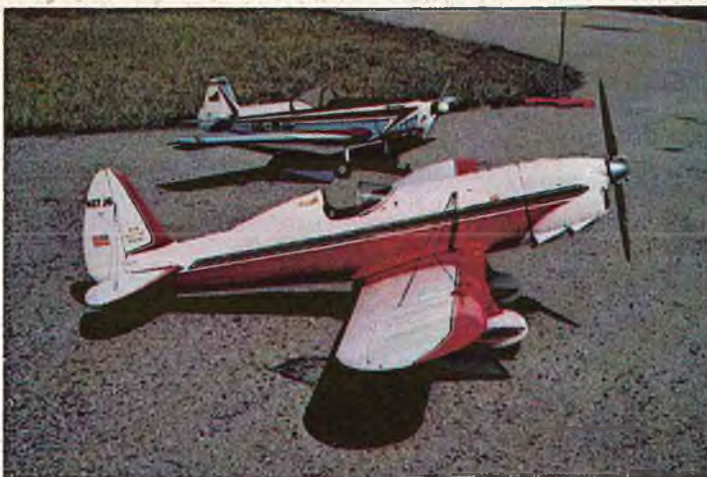
Ryan STA by Denzil Fowler, finished with K & B Epoxy with HP .1 engine, Kraft radio.
