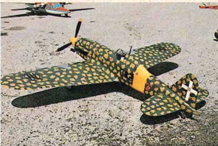
Lucchi C-202 by Bud Atkinson used Enya .60 and EK radio and Rom-Air retracts.
