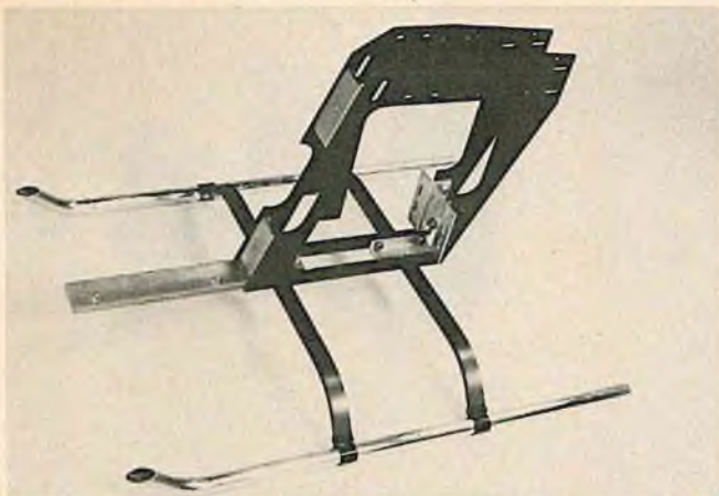
The blue anodized frame halves bolted together with the flat center channels. Note PEM nuts in channels.
