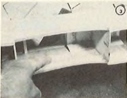
3 Preparing fuselage side for subsequent servo installation by smearing 5-minute epoxy on the area.
