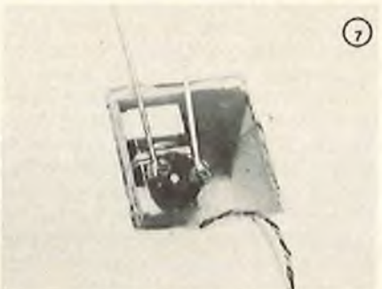
7 Vertical alleron installation showing a servo mounted in a Super Kaos .40 wing. The wing is deep enough to accept the entire servo.
