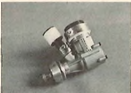
My Rossi F 60 Speed converted to marine use with a brass water-jacket epoxied in place, and an OS No. 4 flywheel. Going well, but needs routing out a bit.
