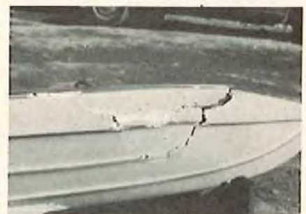
Honest, fellas, it wasn't my fault! This guy got in front of me when I was traveling fast, and --- BANG! (My boat doesn't have a mark on it — I bury 4mm music wire in the glass-fibre around the outside edge of the deck!)
