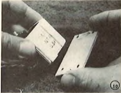
Servo about to be attached to ply plate which is part of horizontal servo installation.
