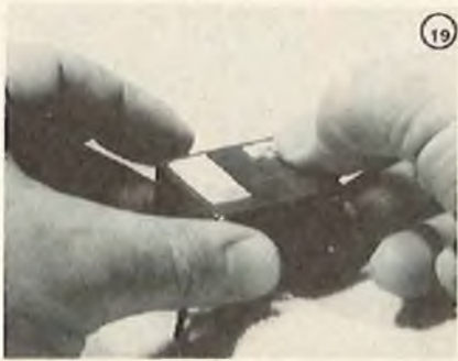
19 Rubbing tape residue off of servo case.
