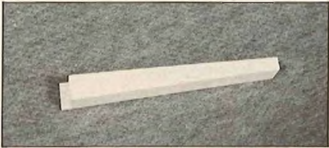
Balsa side block showing cut-out for bulkhead 2.
