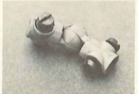
Center piece can be removed to make a single universal.
