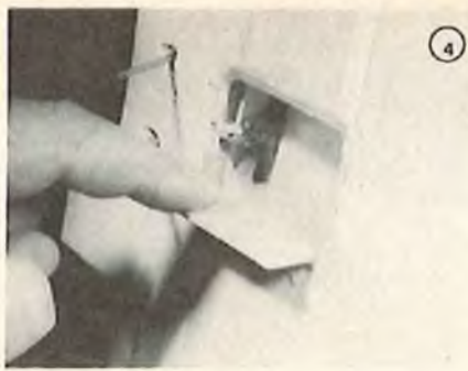
4 Preparing vertical alleron installation by smearing 5-minute epoxy on the longer side.
