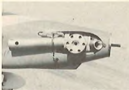
New front intake K & B 6.5 In Jeff Berken's Toni. Jeff uses a remote needle valve as described in the text, mounted to the firewall to keep his fingers further from the prop.
