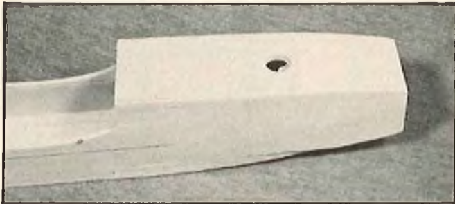
The bottom of the fuselage showing the chin block and fuel tank compartment bottom block.
