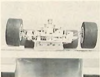
A much simpler Tweak Board, but one that is very effective. Has a piece of 1" special plywood with a piece of 1/4" glass cemented on top. Make sure wood is flat. Left side of photo, a 3/8" rod is placed under the tire. The other front tire has raised 1/8" off the glass. The rod is switched to opposite front tire & the amount of the opposite front tire is checked. It should also be 1/8", otherwise chassis is tweaked. Never use the ground to check tweak!
