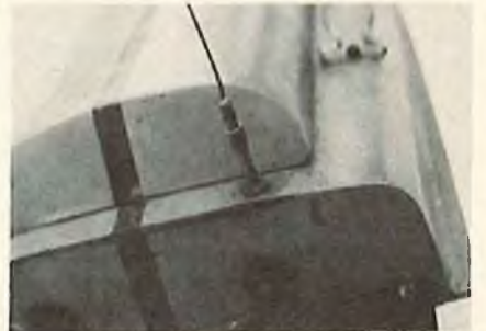
Banana plug and socket fitting. Beware of vibration with this one.
