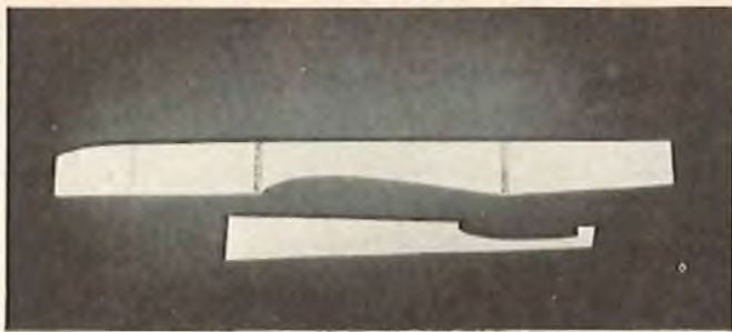
Fuselage side showing wing and stab cut-outs.
