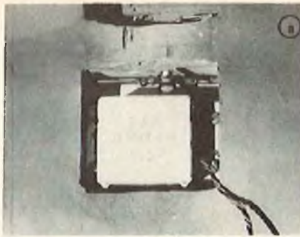
Horizontal aileron installation in a Skylark wing. This is a twin . . . open above servo is for throttle servo.
