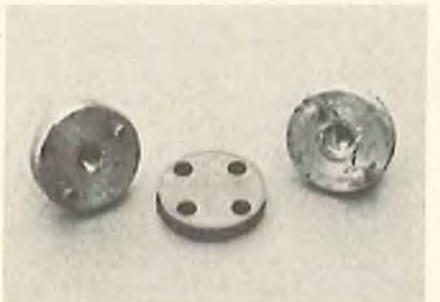
Racing Models pin-and-disc coupling - will take up to 3bhp.
