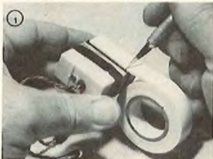
1 Installing hobby-type mounting tape on a servo.
