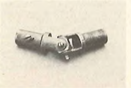
A small, metal coupling, taken from an old TV tuning knob.
