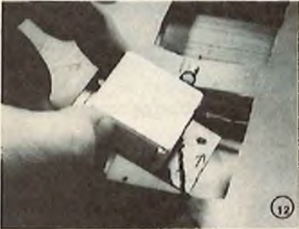
Servo attached to mounting plate, about to be installed in Skylark wing.
