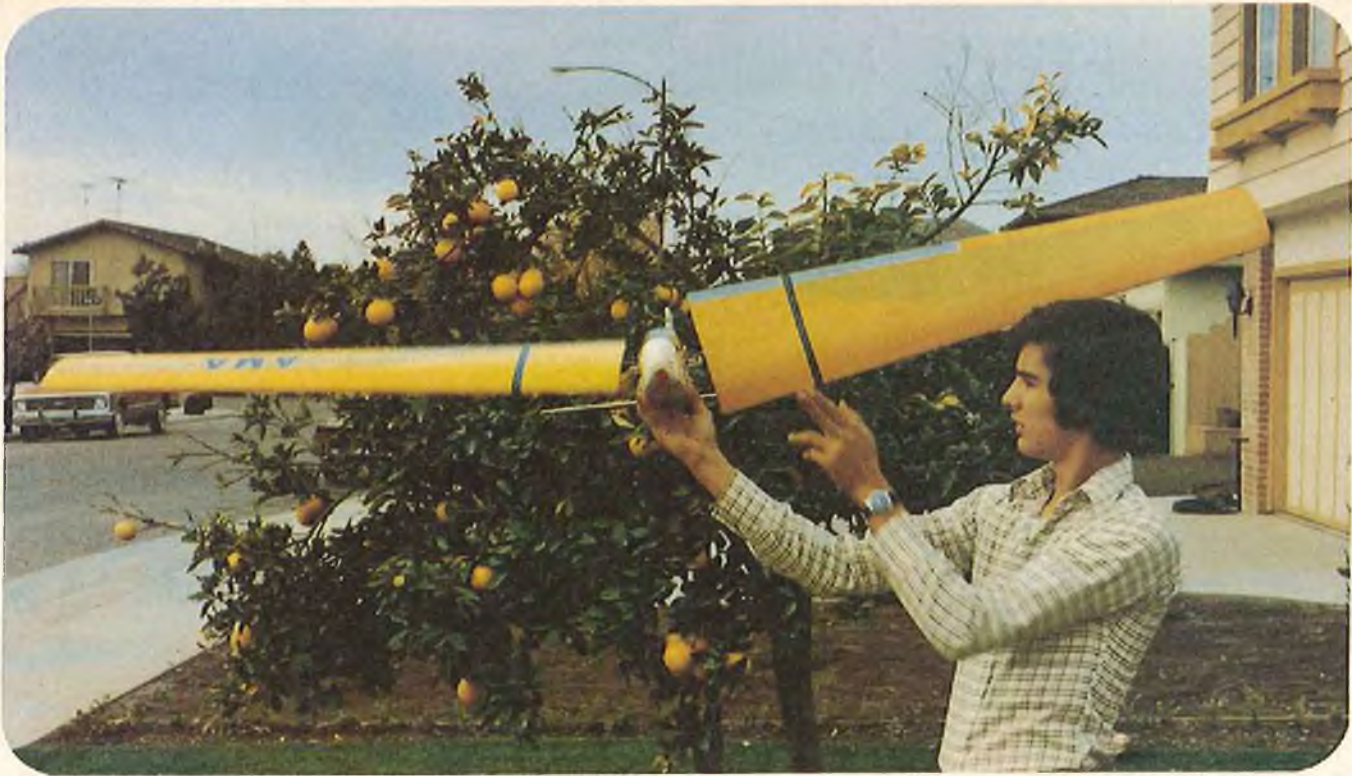
Author Billy Walker demonstrating rotating wing panels on glider.
