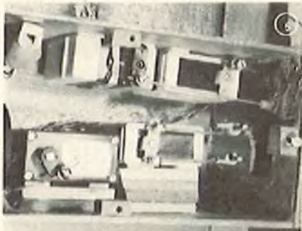
5 Quarter Midget installation showing two servos taped directly to the sides, and two servos mounted on Stand-Offs.
