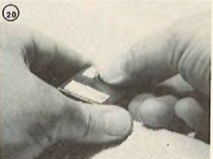
20 Another view of tape residue being rubbed off of servo case.
