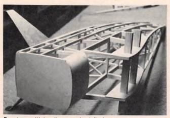
Fuselage with landing gear installed.
