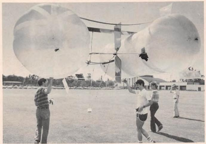
Caltech students test their ten foot model of a solar powered airship. Caltech photo by Richard Kee.
