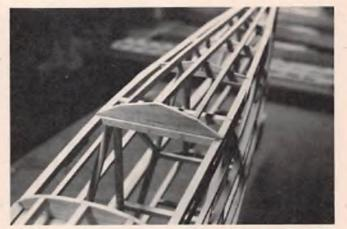
Fuselage bottom showing access hatch detail. Note rounded front former and angular rear former.
