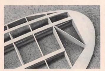
Wing tip with geodetic rib installed.
