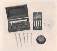
Midget tools of the detailing trade: Morris E-Z tap and die set, E-Z socket wrenches, X-Acto 6412 Carbon Drill Stand Set with bits from No. 80 to No. 61, jeweler's screwdrivers.
