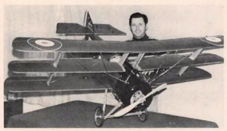
George 'Woody' Clapp and his first RC model. A Sopwith Triplane which was drawn and scratch-built by Woody. Now that's a fairly ambitious project for a first time RC modeler, small wonder he's wearing such a broad grin. Wires are functional and the spoked wheels are scratch built as well.
