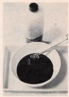
Immerse the board into the Etchant.
