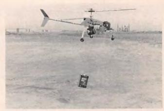
MH-17 lifts off with cable canister and a full gallon can of missile mist fuel.
