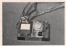
The Mocontrol VC electronic speed controller, now sorted out and working very well.
