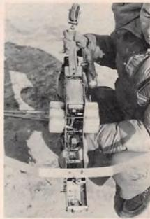
Bottom view of fuselage. Note dual fuel tanks. Tail boom removed in this picture.
