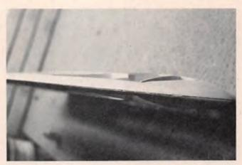
View of wing tip showing reference mark for sanding.
