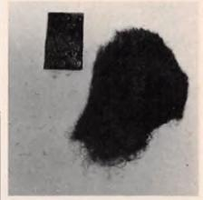
Remove the black resist with steel wool.
