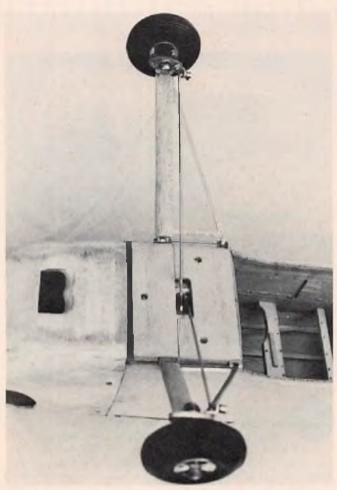
Balsa cover finishes bottom of fuselage and is held in place with three screws. Installation is neat and clean.
