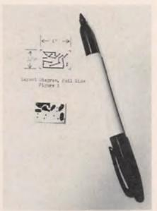
Apply the resist to the copper side of the pc board as shown in the layout diagram.
