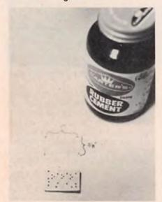
Cement a copy of the drill diagram to the side of the cut pc board without any copper.
