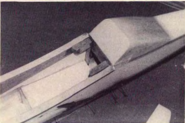
P-51 fuse bottom w/foam belly pan, wing mounting blocks, foamboard cockpit floor. Pins holding canopy in place.
