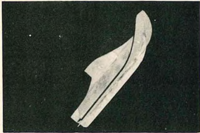
Finished front ski. Note runner on bottom and built-up top.
