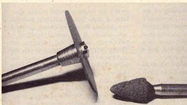
Dremel cut-off disc, on the left, is used to rough cut the air grooves in clutch bell and the small tapered stone is used to finish the grooves.
