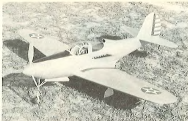
No model engine or exhaust sticking out on this one. Bob Walker's Gold Coast entry was modified from Top Flight P-39 kit. Extension shaft turns prop. First in Sportsman Class. Bob is from Lantana, Florida.
