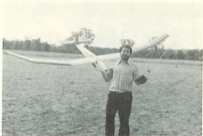
Dr. Richard Solomon from Sydney — Electrolite electric sailplane, Hunter Valley Champs, Muswellbrook, NSW, Australia. Keller motor 14/6 folding prop, direct drive 3-Meter wing 14 oz. wing loading.
