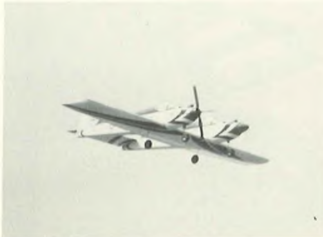
Will it fly on one engine? Sure, any Kougar will fly on one engine. Dummy feathered prop is just to show it will also take off on one engine. Either one!
