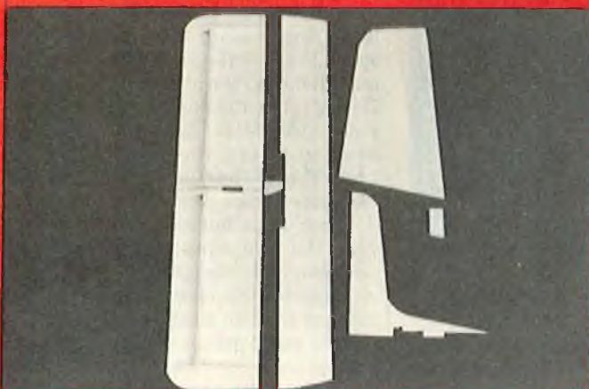
All the tail parts completed — note fin tab and slot in stab.
