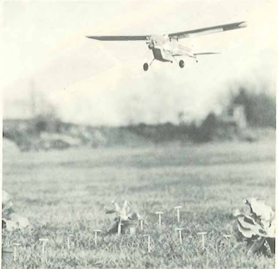
Making a test run, a radio controlled model airplane delivers a virus-laden liquid spray over cabbage plants to infect harmful insects. The virus infects only cabbage loopers, says entomologist K. Duane Biever of USDA's Biological Control of Insects Laboratory, Columbia, Missouri. The idea behind the experiment: Cabbage loopers from non-infected areas of a field will be a source of food for parasites and predators. Then as the virus spreads from infected "hot spots" of the field, it will be one of several pest controls in a balanced ecosystem of integrated pest management. Photo courtesy of U.S. Department of Agriculture.
