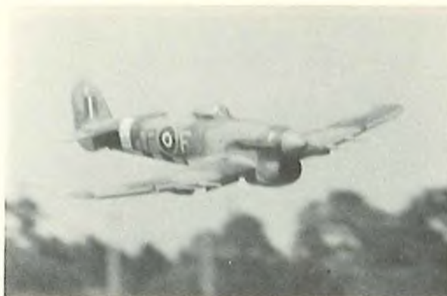
Original design Giant Scale Hawker Typhoon flies with piped Rossi .90. Pipe is buried in fuselage. Wayne Knight's creation, 1/6 Scale at 22 pounds.
