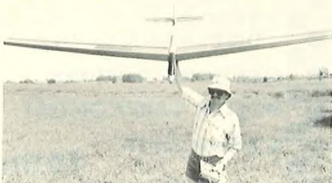
Tom Nellson, one of the North West Soaring Society's top fllers, with his multi-channel Bob Dodgson "Maestro Megan" designs. At 140 in. wingspan, 1300 sq. in. wing area and 4.5 lbs. weight, this is the petite end of the size scale ships discussed in this article!
