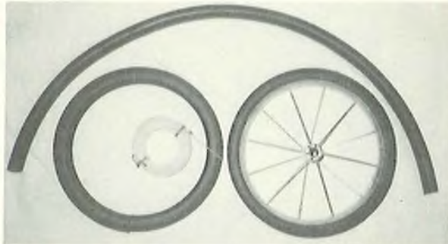
Spoked wheel as purchased and necessary material to rebuild it. Heater hose and nylon weed-eater line.
