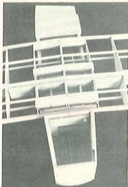
Wing mated to fuselage — note landing gear blocks installed in wing.
