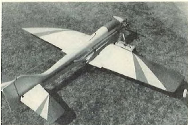
Note pipe "re-entry" into fuselage and downward. Provides a minimum of messy goo with no power loss.
