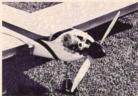
One of the first prototypes — all white with black trim. Big mill sits at angle for proper fuel flow level. This is the design you'll see in the winners circle.
