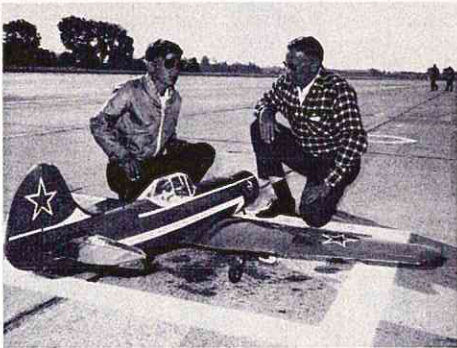
Jimmy and Bill Hiller, Sr., ready for Nats round. YAK powered by Webra, Top Flite 14 x 6 prop. Pro-Line radio, Go-Pop fuel.
