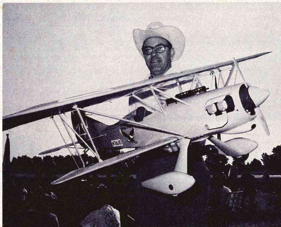
Top scale points went to Lumley Chipmunk by Hale Wallace. Ship totaled on 1st flight. 9 lbs., Webra .60, Top Flite 13 x 5½ prop, Kraft radio.
