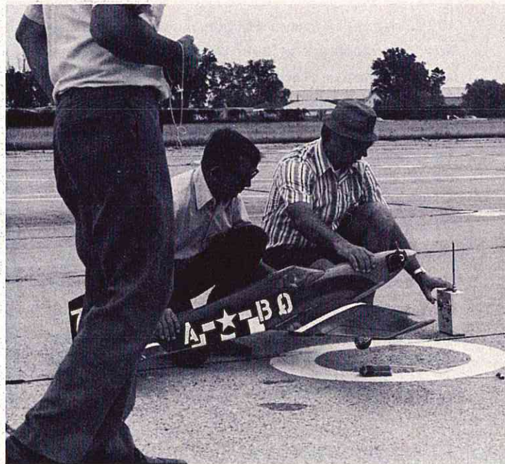
"Miss Florida" was Mustang-X original by Jim Kirkland. Placed 5th. Smallest ship at 5½, was fitted with original retracts, Pro-Line radio, Super Tigre .46.
