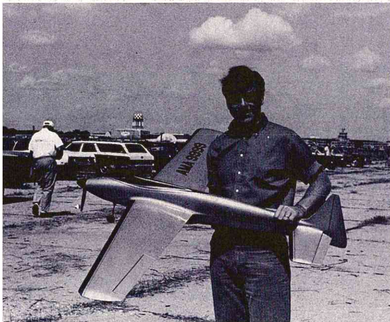
Banshee is new pattern ship by Jim Martin, 3rd place in 1971 Chicago Nats. Pro-Line radio, new Rom-Air retracts, Silence-Aire muffler. To be kitted by J & J.
