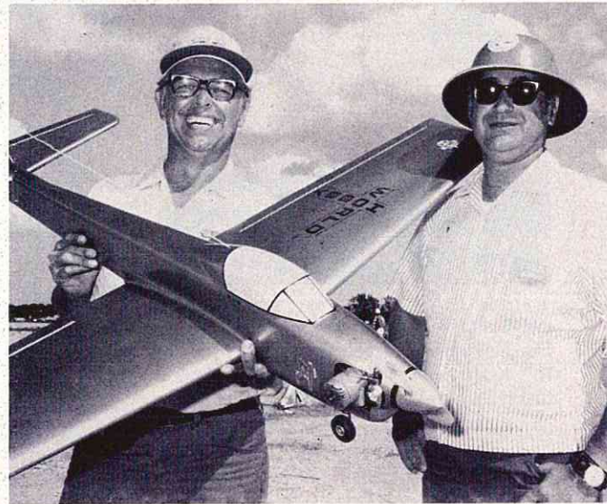
Bob Reuther, Hobby World chief, was Pylon events director, flew C Pattern with A-6 Intruder. Kirkland design weighed 7½ lbs. from Skyglass kit. Kraft radio and retracts in neat ship.
