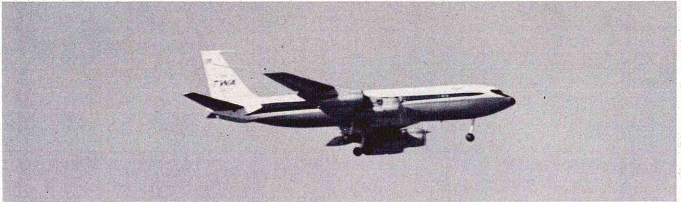
Paul Martin flew crowd-pleasing Boeing 707-320. Flew very well on 2 ST .60 engines with 11 x 7 props.
