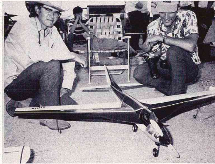
"Warlock" is original pattern ship by Jim Wilmot. 7 lb. ship had ST .60, modified Posittract retracts for mains. Outriggers contact ground first, ease ship into landing. Good idea . . . Ed Sweeney, AAM Editor, interested.
