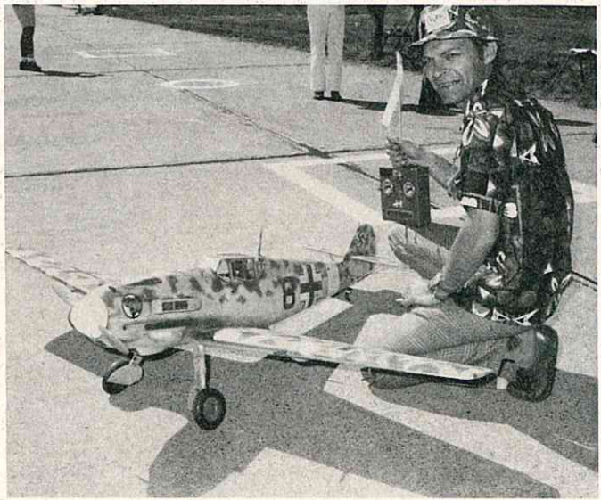
ABOVE, LEFT: Platt Me 109 weighed 9½ lbs., used OS Goldhead .60 RR. Top Flite 12 x 6 prop. Fox glow plug. Go-Pop scale special fuel. ABOVE: Dave Platt had usual high scoring scale point ship for 1971 Nats. This one, Me 109E-4/N trop. Stall on takeoff wiped nose out. Repaired for attempt next day. Top Flite 12 x 6 prop. Fox glow plug. BELOW, LEFT: Dornier DO 335 by Bud Atkinson is veteran of scale meets. 10¼ lb. ship powered by Enya .60 had Logictrol III radio. 11 x 7¾ prop. BELOW: Best Junior in Scale went to Jimmy Hiller, Palos Park R/C Club of Chicago. Jimmy, RC veteran at 14. YAK weighed 8½ lbs. . . .
