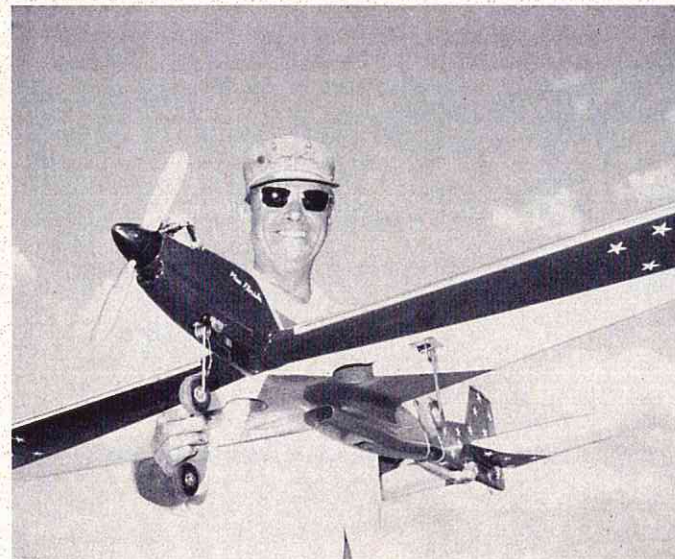
"Miss Florida" was Mustang-X original by Jim Kirkland. Placed 5th. Smallest ship at 5½, was fitted with original retracts, Pro-Line radio, Super Tigre .46.
