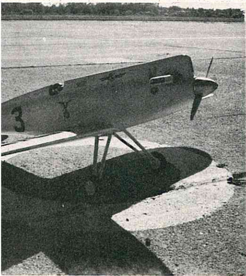
Howard "Pete" was scale rendition for FAI event by Alex Chisholm, AMA Dist. X V.P. Kraft radio, K & B .40.
