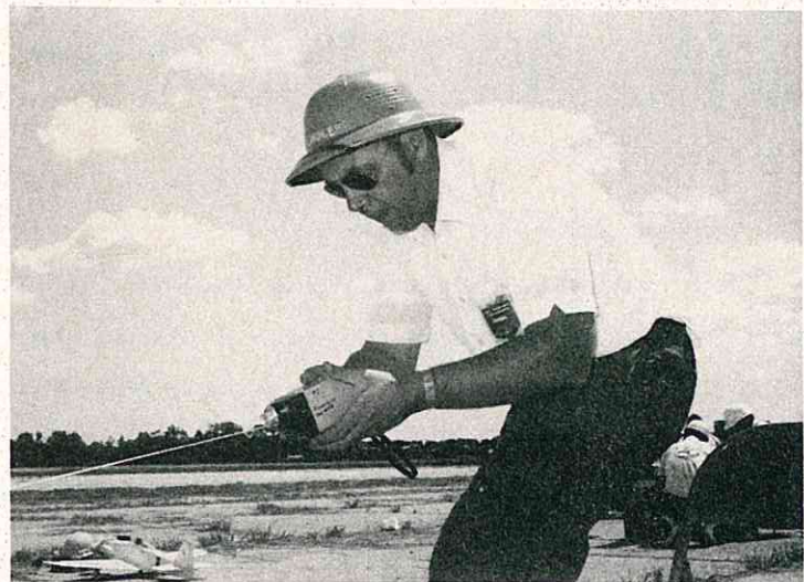
DB meter is inexpensive device available at Allied Radio Shack outlets. Here Don Lindley takes reading.
