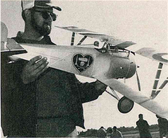
BELOW: VK Nieuport with Nungasser trim by Dave Dobbs. 6 lbs. ship had OS .60, 14 x 6 prop for power. Heathkit radio in 2" scale ship.
