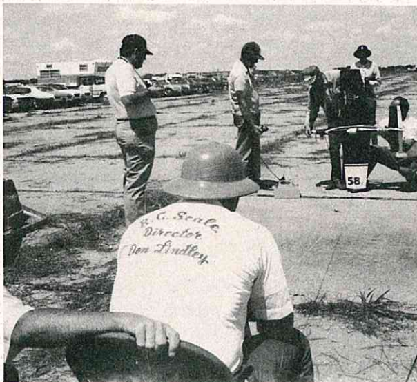
Muffler noise output was measured at 15' distance. Don Lindley collected data for muffler research effort. Measuring sound complex . . .
