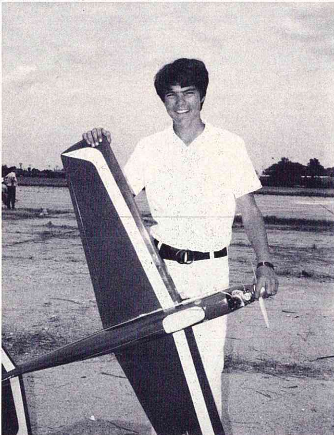
Jerry Worth and Pantera (Panther) X-7 for 1971 Nats. 7½ lbs. ship had Webra, Pro-Line radio and retracts.
