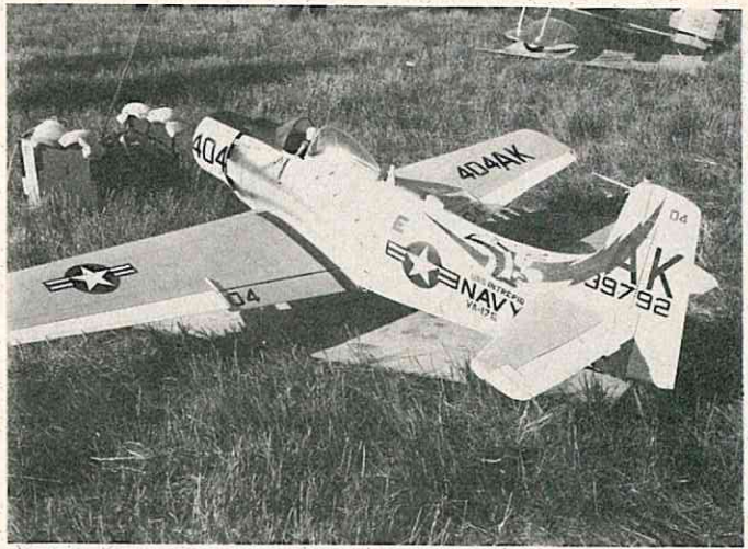
More detail of Skyraider finish. Workmanship apparent. ST .71, 12 x 6 prop. Micro-Avionics radio.
