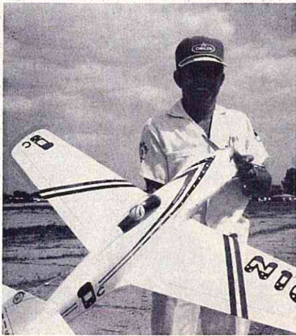
ABOVE: Hal DeBolt and 8th place Mustang original. K & B .40, Orbit radio, Pete Reed 50% nitro fuel. BELOW: Minnow and Cliff Weirick, 14th at 1971 Nats. PCS radio, K & B .40, K & B Supersonic Speed fuel.
