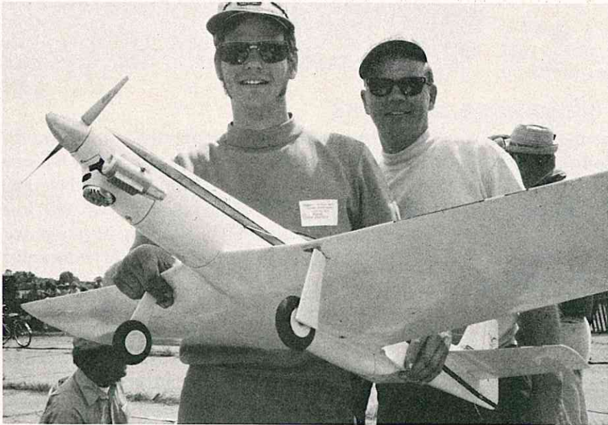
BELOW, LEFT: Bob Noll, Endicott, N.Y. had neat red and white original P-51 for 5th place in FAI racing event. Silence-Aire muffler, Pro-Line radio, K & B .40 RR engine. BELOW, RIGHT: Jeff Bertken – co-designer of Miss BS – placed 6th with his Lee/K & B .40 powered version of popular racing ship. Kraft radio, K & B idlebar plug, most popular.
