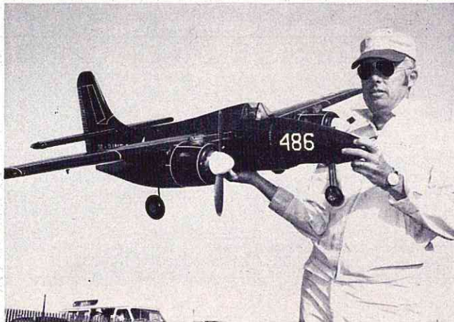
Grumman F-7F was 12 lb. entry by Bob Campbell for 1971 Scale event. 2 Webra .60's plenty of power with 11 x 8 props. Kraft radio. Kitted by RC Kits.
