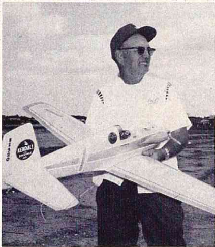
ABOVE: Hal DeBolt and 8th place Mustang original. K & B .40, Orbit radio, Pete Reed 50% nitro fuel. BELOW: Minnow and Cliff Weirick, 14th at 1971 Nats. PCS radio, K & B .40, K & B Supersonic Speed fuel.
