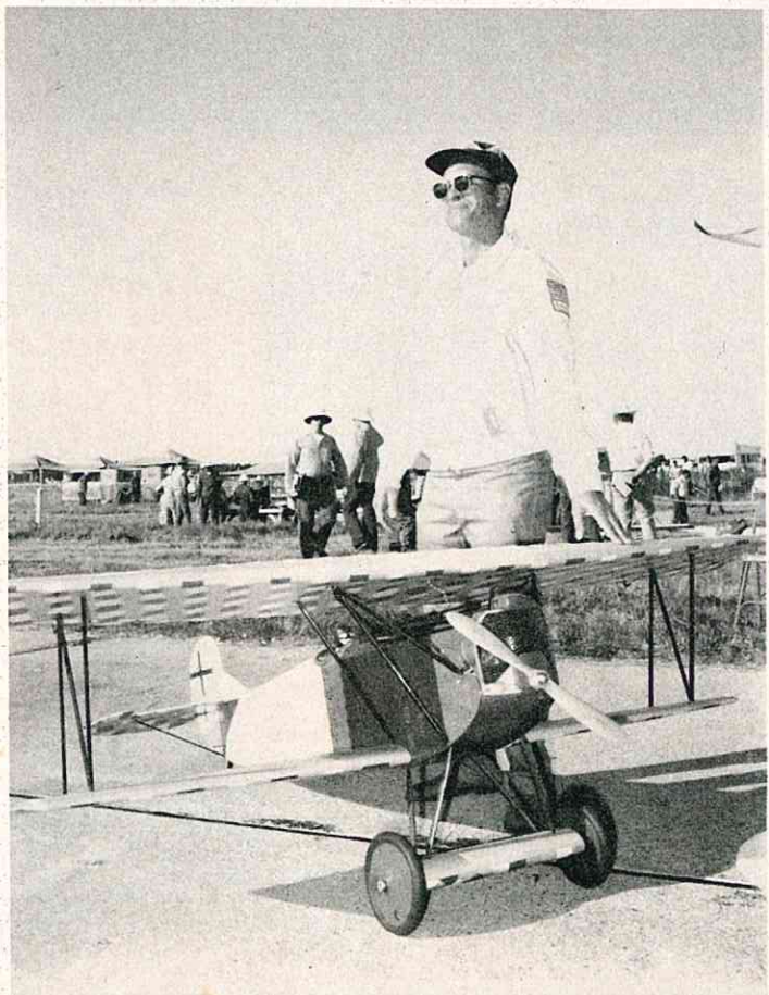
Bill Bertrand and 1/4 size Fokker DVII are Nats veterans, ship's 4th Nats performance. Placed 7th. 15 lbs., O & R compact engine, 22 x 4 prop, EK radio.
