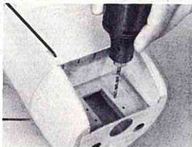
Drill engine and equipment mounting holes.
