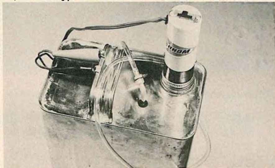
Pump mounted and vented as suggested by author. Tatone stick-a-tube in top of container holds fill line. Rubber gasket under cap on pump mounting.
