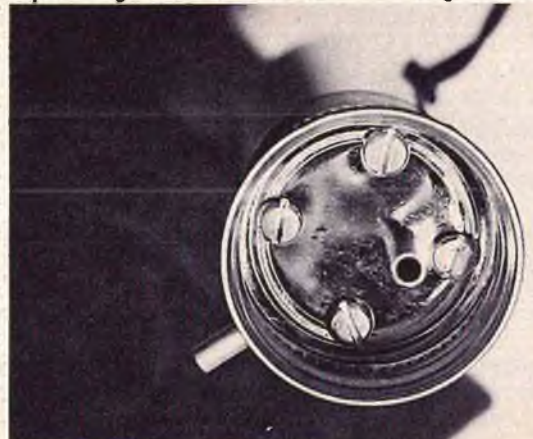
Mounting screws act as spacers allowing fuel container to be vented. Read article for other suggested venting ideas.
