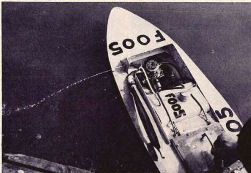
Gazelle with Taipan Goldhead and covered-out Super Tigre Mag III carb. If you look carefully, you will see that the throttle is less than half open, but the cooling system is already working with the boat at a standstill. Note also the throttle linkage going through the tank.
