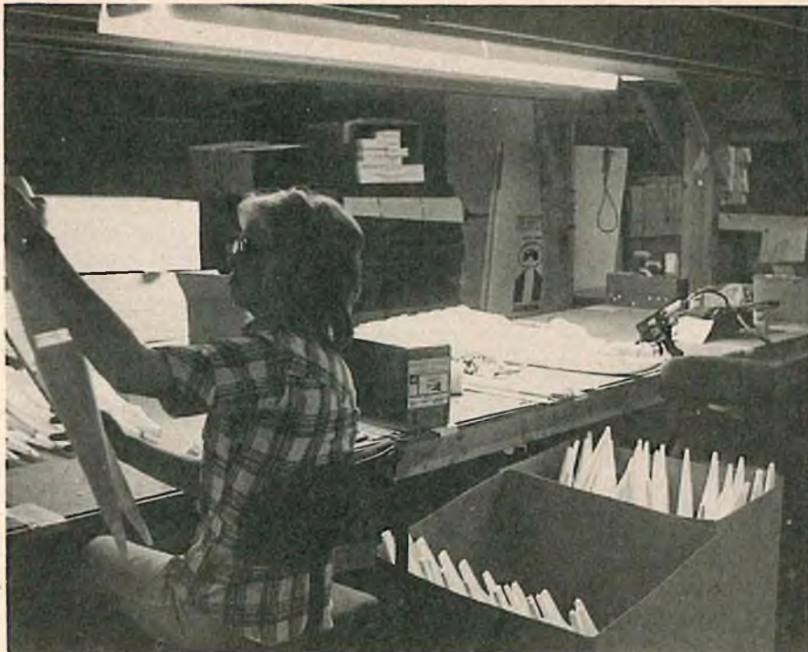
ABOVE: Packing small kits, the proper number of parts are taken from each bin on right and placed into boxes by employee. RIGHT: Foam ARF's are assembled from pre-molded parts.
