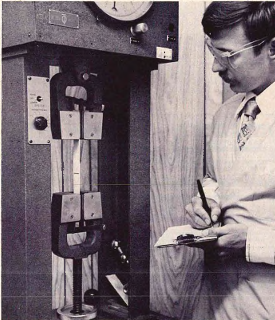
Pacer engineer testing the cyanoacrylate bonds on a tensile testing machine.
