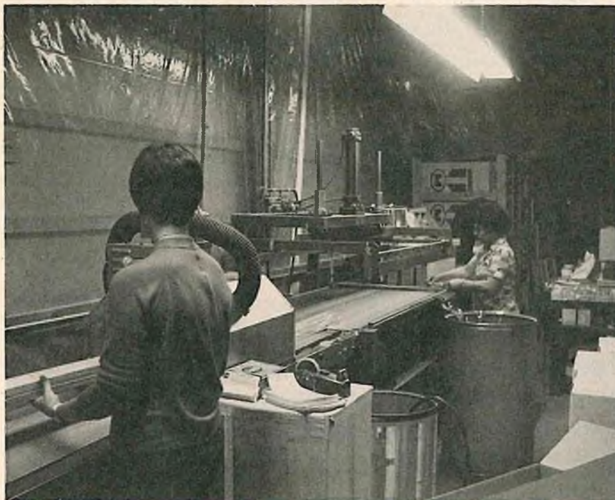
RIGHT: Heat shrink plastic is used to wrap balsa sheets and small kit boxes. BELOW: Midwest Products' Frank Garcher tends business in the front office.
