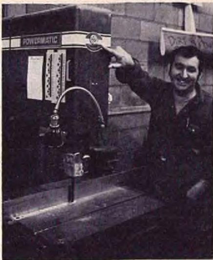
LEFT: Bandsaws similar to this are used to cut balsa and other materials into sheets which are then sanded to close tolerance and cut to length. Bob Vojslavek, REV's president, shows his is "powered by HP".
