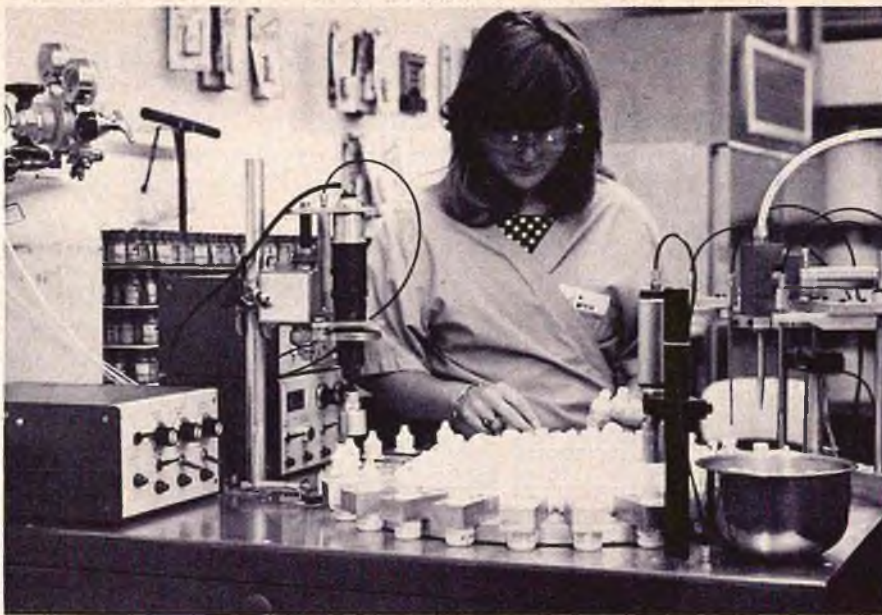
Zap being filled by automatic gas transfer filling machine.
