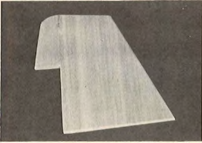
The rudder is of simple two-piece sheet balsa construction.
