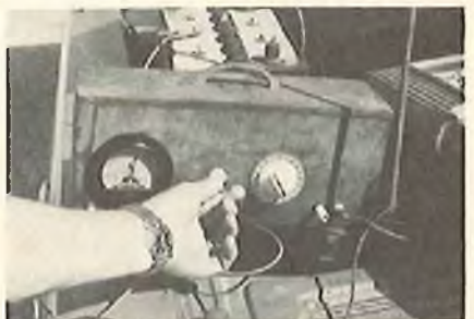
Adjusting the variable resistance to keep the current at a constant 6 amps.
