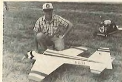
Dean Koger had the largest pattern airplane with 1050 sq. in.; 10 lbs. Uses Proline, Rossi & pipe.
