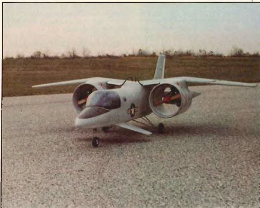
FIG. 4: Grumman design 698 VTOL; two O.S. 40 FSR's in 7" ducts.
