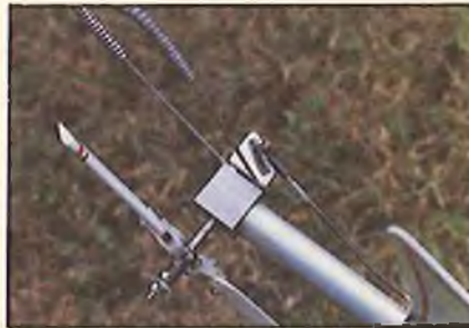
Harold Moore's mod. to Hell-Baby tail. Copper pictured upside-down for clarification.
