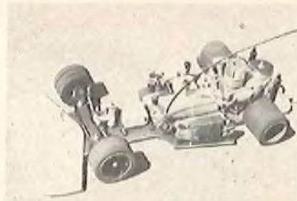
Phil Booth's P.B. car. Notice the rear tires are smaller than the fronts. Large round unit behind K & B 3.5 is a very quiet muffler.
