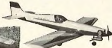
SUPER LUCKY FLY SUPREME New Fibreglas Fuselage-Wings covered with 1/64" plywood
