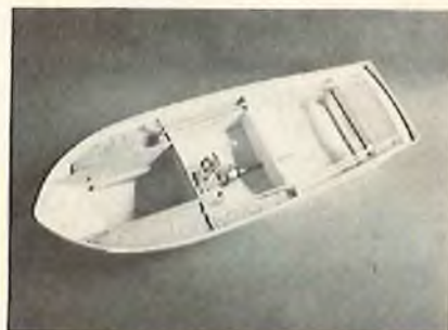
The 'Taifun' with engine and stern-tube fixed in place. Notice expanded foam, used to prevent sinking (I'm an optimist!).
