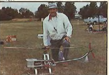
Bill Youmans scratch-built with Kraft .60 engine.
