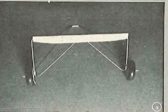
(1) Bottom view of basic fuselage structure. (2) Top view of basic fuselage structure. (3) Glue 1/16" ply doubler inside fuselage. (4) Bottom view of fuselage showing 1/16" balsa sheeting (5) 1/2" sq. balsa & bulkhead cut out in cockpit area. (6, 7, 8) Wing panels built by clamping spars together. (9) Main L/G block ready for installation.
