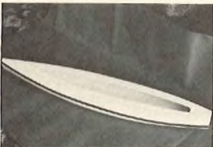
The Impi hull molded in glass fibre.
