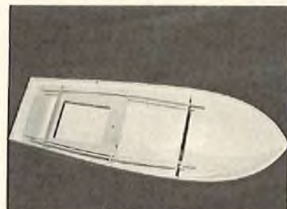
The Graupner 'Taifun' hull in ABS, with some of the reinforcing parts built in.
