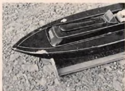
Prototype Cobra after a hard ride! The new Hobbypoxy filler soon sorted this out, and the hull is now as good as new.
