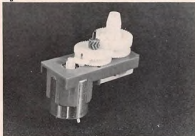
Gear, next to motor pinion, in lower gear ratio position. Less responsive, slower transit time but more power.
