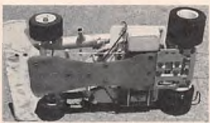
With the tuned pipe coming over the top of the radio tray, the batteries and receiver are moved underneath.
