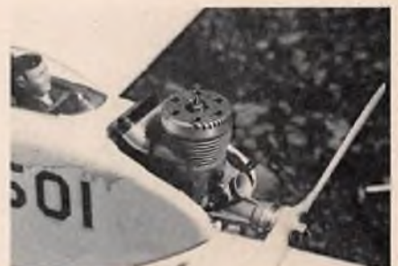
Powerful .60 featuring front rotary disc intake built by Ralph Cooney, Fourmost Racing Products and flown by Dick Hanson.
