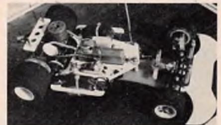
Jeff Rold's race winning Associated RC200 car featuring Futaba radio, K & B 3.5 engine modified with McCoy parts.
