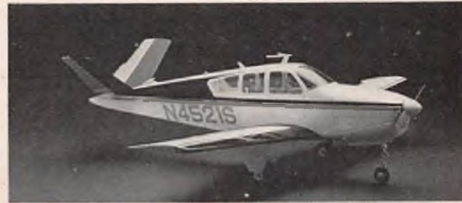
BEECHCRAFT BONANZA • Span 36 in. • Area 216 sq. in. • Length 28.5 in. • Weight 22-28 oz. • Engine TD .049 • Wing loading 14.6-18.6 oz./sq. ft. — $29.95
