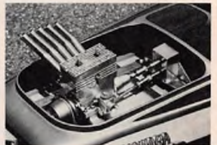
Bob Gregory built the 2 cylinder, 2 cycle water cooled engine and drive train. Engine uses numerous McCoy .60 parts. Beautiful workmanship.
