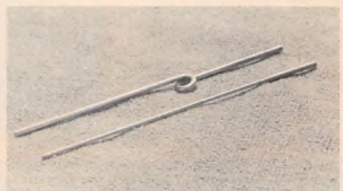
Comparison between stock Robart retract gear leg (3/32" m.w.) and modified leg made from 3/32" O.D. brass tubing and .062 (1/16") music wire. Modified leg is almost 1/10 of an ounce lighter --- works just as well.
