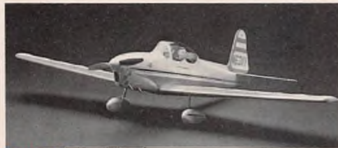
CHIPMUNK • Span 36 in. • Area 216 sq. in. • Length 28.5 in. • Weight 22-28 oz. • Engine TD .049 • Wing loading 14.6-18.6 oz./sq. ft. — $29.95
