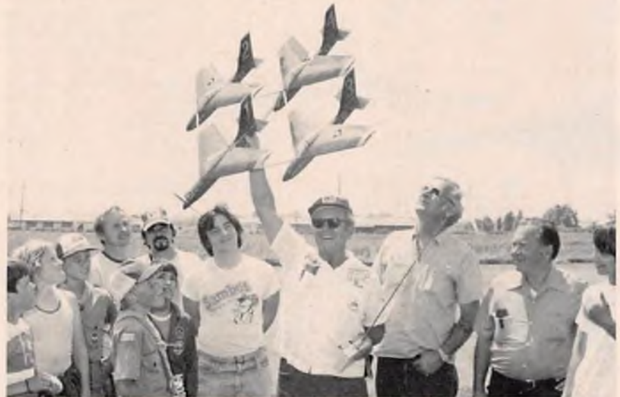
The 'Bluebirds' fly fine on a Max .10 in the nose. An .051 Tee Dee can't pull them.
