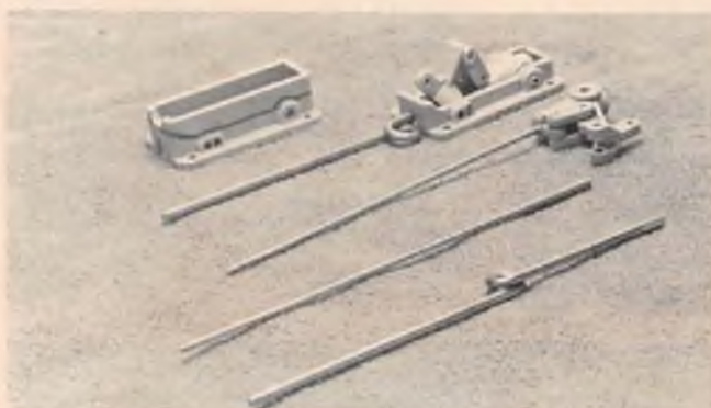
Robart retract mechanisms come apart by removing four set-screws for modification. Larger screws act as landing gear trunnion/pivot and hold gear leg in position. Brass tubing on 1/16" music wire is as long as stock leg support.
