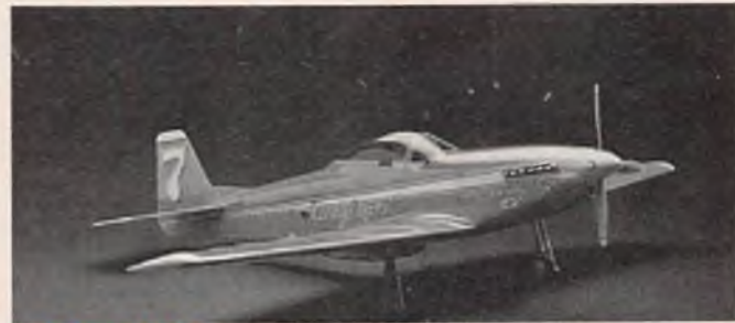
P-51D MUSTANG • Span 36 in. • Area 216 sq. in. • Length 28.5 in. • Weight 22-28 oz. • Engine TD .049 • Wing loading 14.6-18.6 oz./sq. ft. — $29.95
