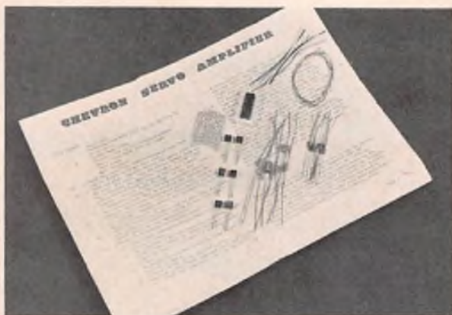
Chevron servo amplifier kit. Board is easy to assemble with good dependable parts and excellent instructions.
