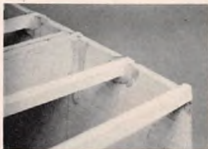
Hull structure showing joints made with new Hobbypoxy No. 3. Thixotropic epoxy glue. As can be seen, it doesn't run.
