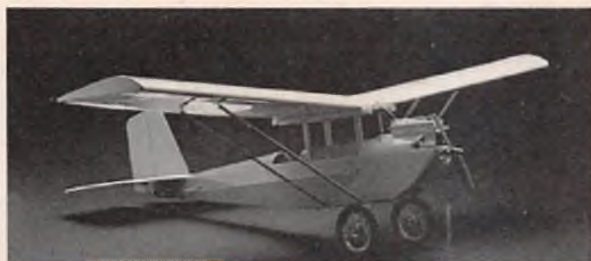
PIETENPOL SKY SCOUT (1/2-A 'PETE') • Span 42 in. • Area 284 sq. in. • Length 26 in. • Weight 22-27 oz. • Engine QRC .049 • Wing loading 11-14 oz./sq. ft. — $22.95
