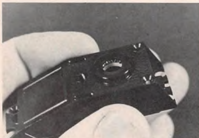
Ball bearings mounted in top cover. Balls are placed in groove and retained with plastic ring. Apply a drop of Hot Stuff to retainer ring.
