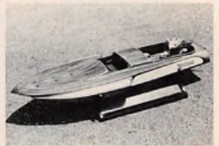
Bob Gregory's Drag Boat uses a Hallet Drag Hull. Length 42", Beam 10", mahogany veneer ply decking, ash wood structure, and leather tuck and roll upholstery.
