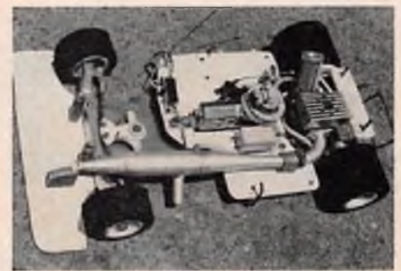
The new trend in exhaust systems as used by Butch Kroells and Rich Lee. Outlet is on the side of the pipe.
