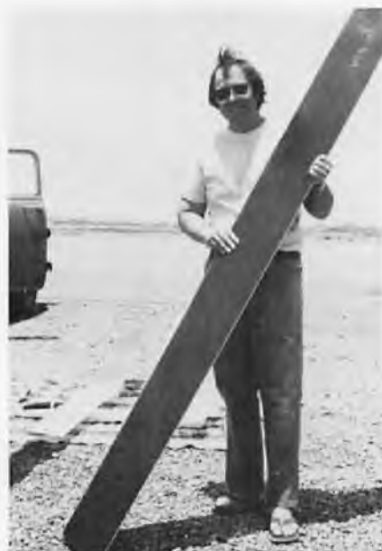
Bill Mueller holds the laminated plank as it comes out of the press prior to ripping into widths.
