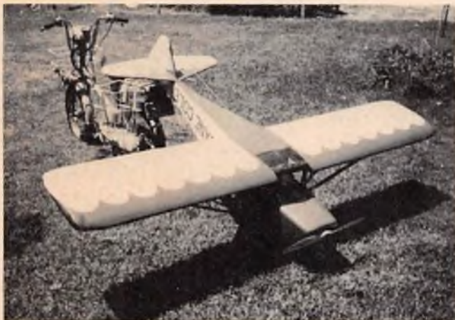
TOP LEFT: Wings attached using large turnbuckle. Cover hatch bolts in place which makes easy visual safety inspection. TOP RIGHT: Strut ends are bolted between two spade bolts. Be sure to use elastic stop nuts at these points. ABOVE LEFT: On its back showing off landing gear and engine opening in cowl. ABOVE RIGHT: Original started out with scale size prop (18 x 10) but had to be changed to a 20 x 8 for best results. LEFT: You meet the nicest people riding a "Honda."
