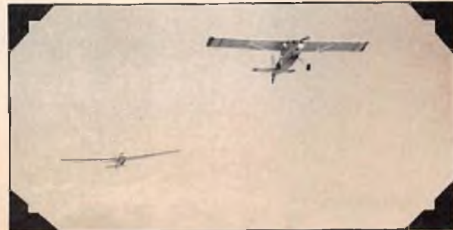
A Schweizer 233 on the tow. Normal altitude above the ground is 3000 to 3500 feet before you cut loose and start thermal searching.
