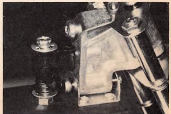
The secret of the steering mechanism is a cast pivot block that converts servo fore and aft motion into front fork tilt.
