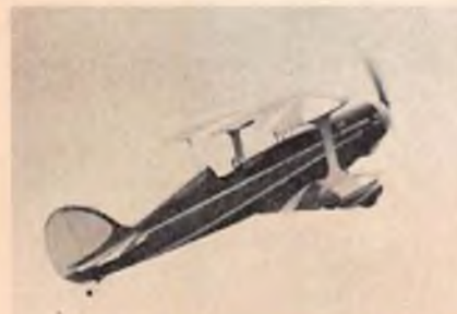
Norm Casella's Cass Super Skybolt rockets up. That big prop is being turned by Norm's new Super Drive unit --- twin .40's on a belt reduction.
