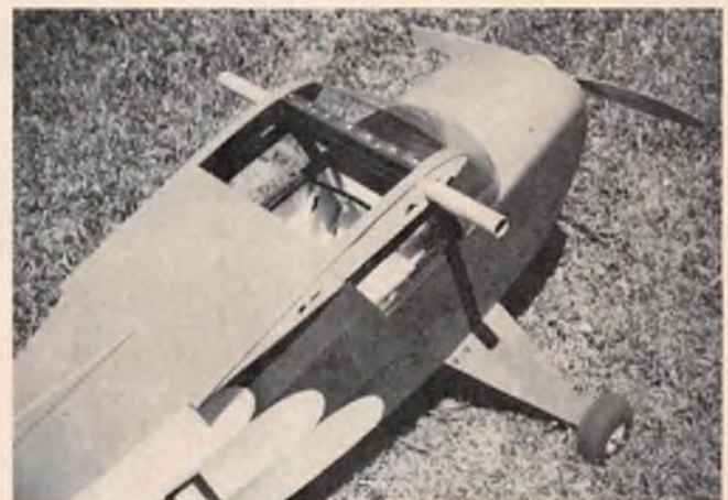
TOP LEFT: Underside of tail showing C.B. tailwheel assembly. Goldberg long horns were used on each elevator. TOP RIGHT: Top view assembly showing 3/64" x 5/16" steel straps for braces. ABOVE LEFT: Wing panels ready to attach to fuselage. ABOVE RIGHT: End view of wing panel. Rear aluminum tube plugs into center section. Front hole accepts tube built into center section. Note servo extension cable for servo in each wing panel. RIGHT: Large aluminum wing tube built into center section. Note spade bolts on landing gear for wing strut attachment. Smaller wheels shown on Taylorcraft are for use with wheel pants.
