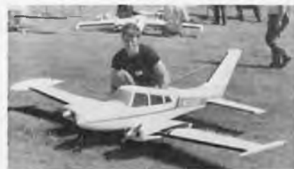
Guy Fulton, Athens, Illinois, and his Nosen 310. Two ABC S.T. .60's, MRC gear and 26# of impressive looking twin.
