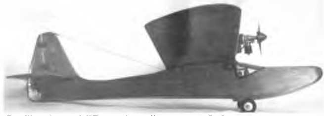
Profile view of "Dreamboat," an early R/C design which had rudder and "kick-up" elevator. Note step under leading edge of wing to reduce "plowing" before applying the elevator, which could only be used momentarily since it was full throw.
