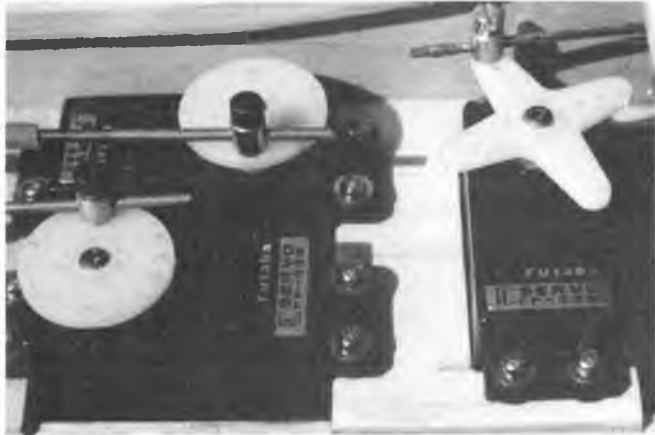
Close up of servo hook-up. Pushrod connectors can safely handle the air loads on Big Bird Too.
