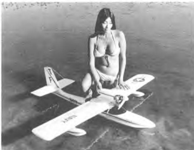
The "Wavemaster" had full house control (rudder, elevator, aileron and engine control) and was very responsive both on the water and in the air. Step was located under the C.G. location and was of "boattail" design instead of transverse.
