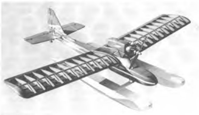
The twin float "Sunday Seaplane" has good water performance because the floats are large and spaced well apart.
