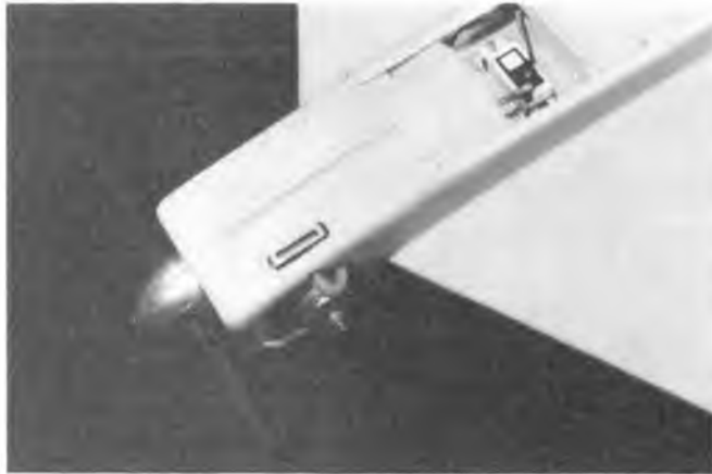
Exhaust is blown out the bottom via a Du-Bro Mini Mufflaire.
