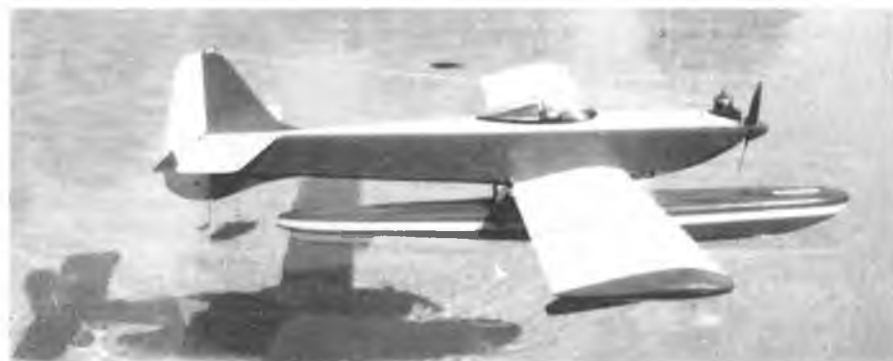
Converting a land plane to a seaplane by replacing the landing gear with a single float and wing tip stabilizing floats, as in the "Islander" design, usually gives more reliable water performance than will twin floats.
