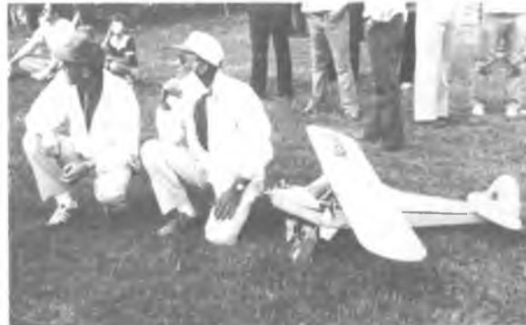
Wesley Van Wyngardon (left) and Wayne Helgager (Sioux Falls, SD) both flew J-3 Cubs that had been enlarged to 84" wingspan from the Sig J-3 kit design. Identical except for a red diamond on the wing of Wesley's model. .60 powered, 8 pounds.
