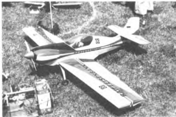
Dale Cordes (New Ulm, MN) built this O.S. .90 powered Zlin Z-50L from an Ohio Super Star kit. 80" span, in colors of German World Aerobatic team.
