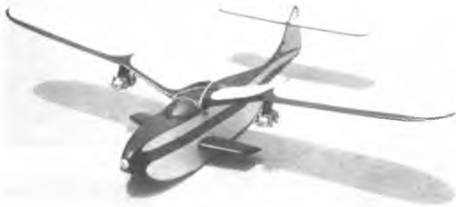
Jetex powered flying boat using "Sponsons" for lateral stability on water. Marginal effectiveness in cross winds.
