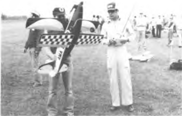
Bill Schneider (Colwell, IA) checks out the needle valve setting on the S.T. Bluehead in his 54" Knight Twister, scratch-built from Bill Heger plans.
