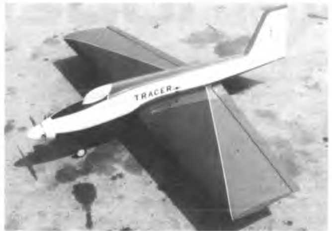
Another mind blower from Bill Evans. This is his pattern aircraft. 60" span, weighs 7¼ lbs., O.S. .60 with tuned pipe and retracts. Maneuvers are unreal.
