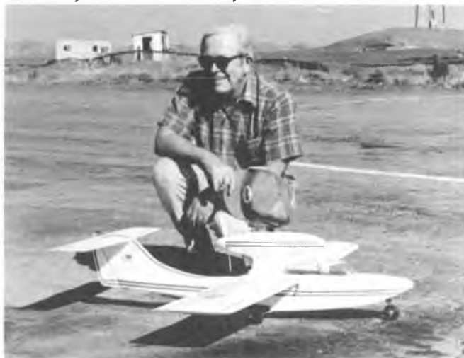
The "Pondhopper" hull was essentially a box-type cross-section with a straight transverse step under the C.G.
