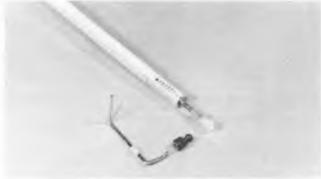
Internal rudder linkage components using Du-Bro ball link.
