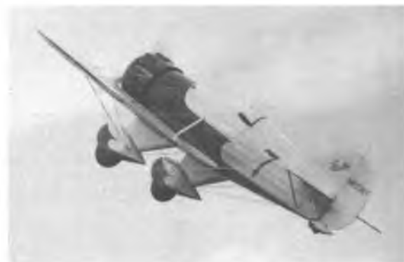
The Quadra in Richard Steine's (Minnetonka, MN) Gee Bee Senior Sport hauls its 19 lbs. up convincingly. 90" span, red and cream.
