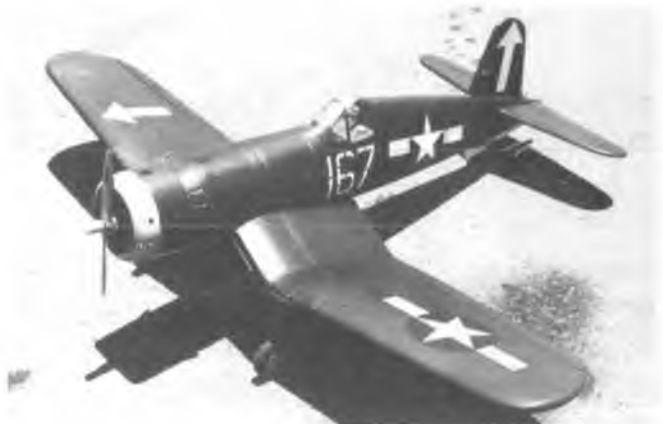
Built from a Jemco kit, Steve Alvarado's F4U Corsair, 6¾ lbs., O.S. .50.
