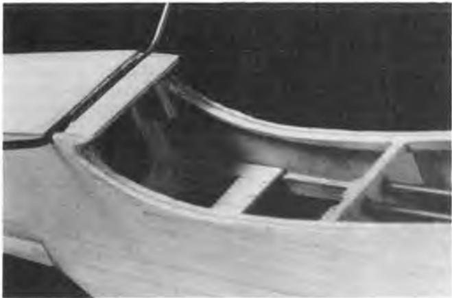
Landing gear torsion bars fit in slot of L.G. mount.
