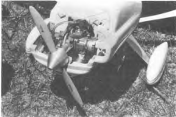
Ray Dray (Rochester, MN) had a Fox twin in his 16 lb. Nosen Citabria. Fox twin is an ideal engine for this type of cowl.
