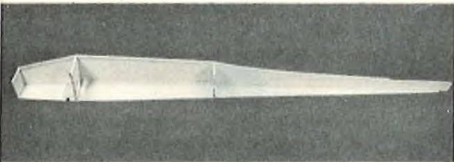
Basic fuselage assembly with left side removed to show internal detail. Structure is simple but very rugged.
