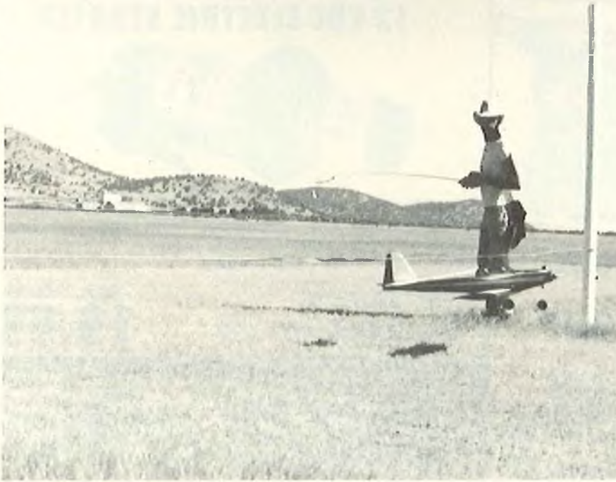
This photo taken by Terry Miller, of Darrell Mullen during the Ilmbo event at Klamath Falls, Oregon. Darrell is flying an Andrews Trainermaster, powered by a Fox .45 BB Schnuerle engine, and equipped with flaperons. The Ilmbo ribbon is set at the 2' level in this shot. Incidentally, the vertical stabilizer did clear the ribbon.
