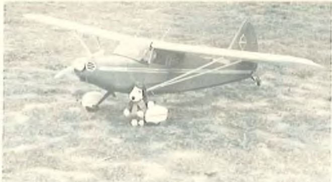
Tony Paul's big scale Stinson. Quadra engine, bird is covered with Ceconite and painted blue and white --- with Krylon spray cans! Files beautifully!
