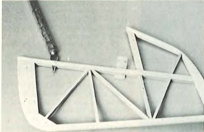
Slotting rudder for hinges. Be careful to cut the slots straight and on the centerline of the surface.
