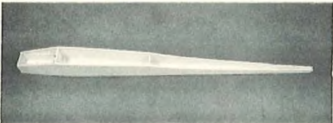
Basic fuselage assembly ready for installation of pushrods and top sheeting.
