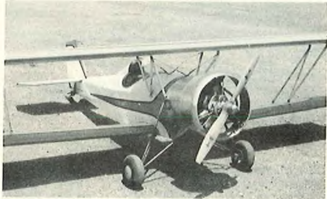
Forrest Edwards made this 3 cylinder engine from Salto .30 parts.
