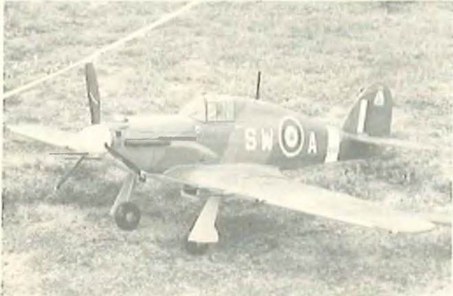
Bill Dunn's monster Hawker Hurricane. Bill drew his own plans for this 85" span, .60 powered beauty. Markings represent bird Bill flew during the Battle of Britain --- he was the first U.S. "ace" of WW II.
