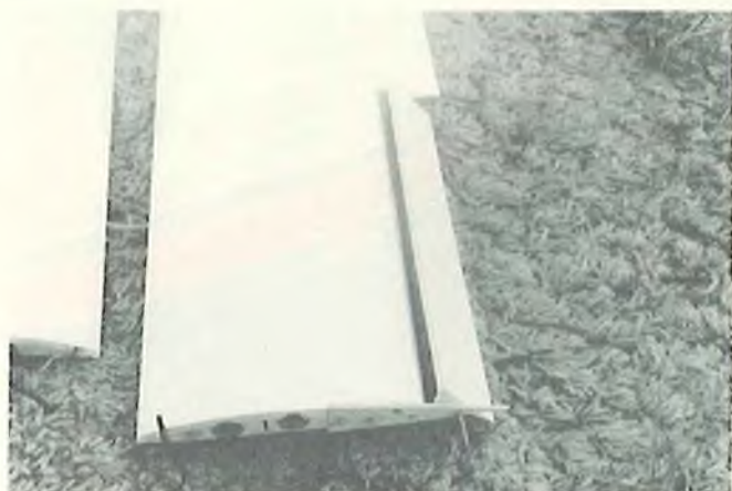
Drag flap design for Mark Smith's "Pffft." Actuated by square tube torque rod (no relation) mated with same in fuselage.
