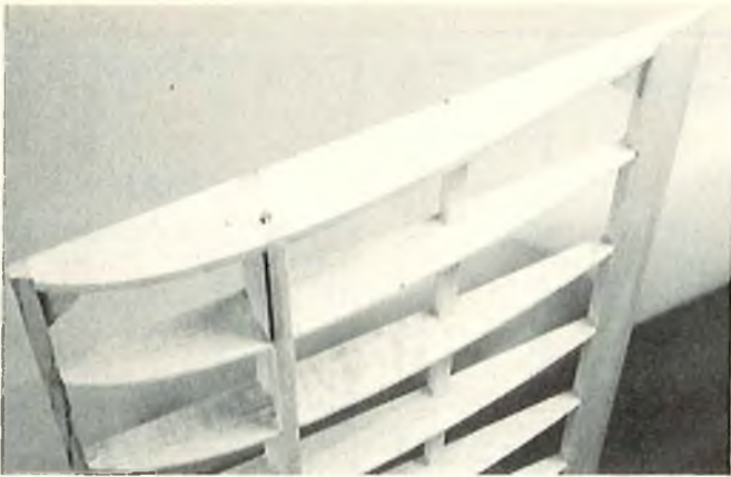
3/16" hole for wing joiner tube drilled in W-3 rib.
