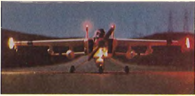
Good shot of all lights — note belly strobe and wing tip skids.
