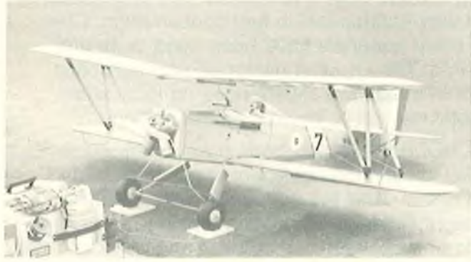
Another of Bill Dunn's home-grown scale designs --- the Falrey "Flycatcher." This .60 powered biplane has an 80" span and features rubberband loaded lower wing flaps for true scale operation. Biggest problem is to balance the pull of the bands to flying speed so flaps deploy on the landing approach! Seems that the local Colorado Springs newspaper provides just the right bands for this great flying scale ship.
