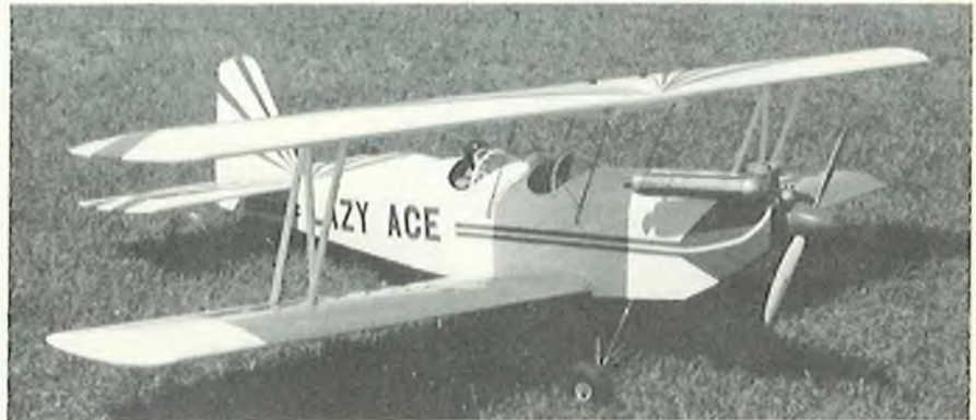
Lazy Ace with Silence-Vox muffler on Webra .91, soft purr at high throttle.
