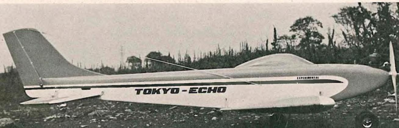
As mentioned, the main advantages for aileron-only control is that this system can be used for scale models, providing adequate control action without deviating from scale dihedral. On low wing single channel designs, smooth maneuvers can be performed, eliminating many of the undesirable characteristics of rudder-only control. Again, an exaggerated amount of dihedral is not necessary, as it would be in the case of rudder-only configurations.
