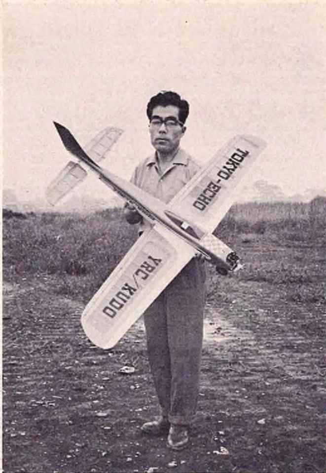
*The author and a Tokyo Echo prototype. A new standard in single channel performance with aileron-only control. Has been flown 6-channel with slight modification.*
