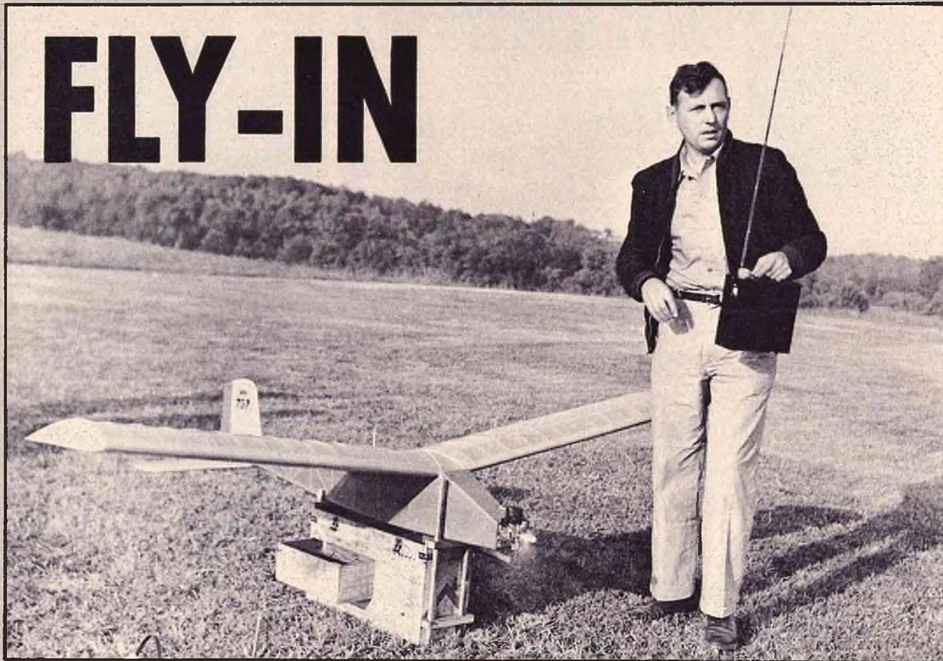
*Hill's original design—88" span, Merco .49 engine, Sampey gear. 4½ pounds of fuel!*
