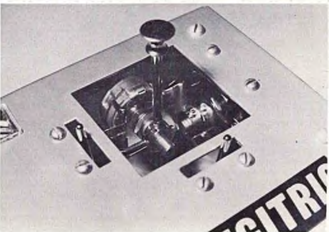
Left, top to bottom: Transmitter case with all hardware mounted. Second and third photos show detailed close-ups of stick and trim pot assemblies. Fourth photo, opposite, shows the completed stick from the front. Above, top; Throttle stick assembly and P.C. board mounting posts. Above: Proper position of transmitter and P.C. board during final assembly and checkout.
