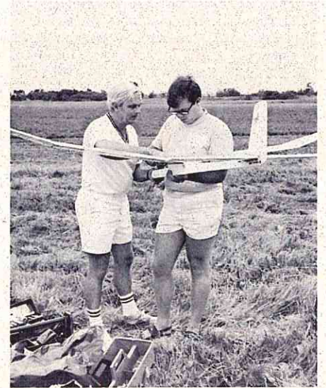
Jeff Mrlik's winning sailplane featured a fiberglass fuselage, modified Cirrus airfoil. Wingspan is 151" with a total area of 1370 square inches. Weight is 5 pounds. Astro-Jeff, designed by father, Jerry, has all-flying stab and rudder plus spoilers.
