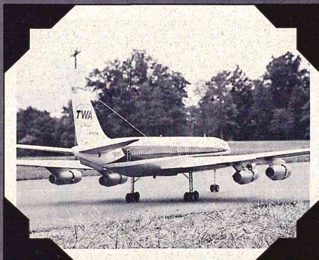
Original design retracts operate from crankcase pressure stored in accumulator.
