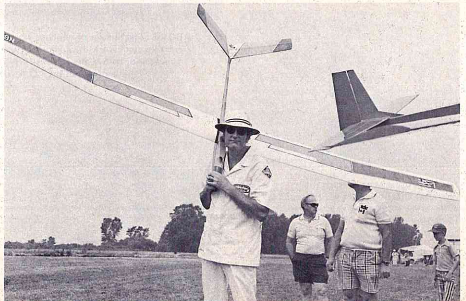
ABOVE, LEFT: Long wings — 195" original design by Jim Porter of Bonita, Iowa. Shrike-W weighs 5 lbs., has all-flying surfaces. ABOVE, RIGHT: Bob Gill (r), winner of Precision, adjusts servos in Airtronics Olympic as Tom McCarthy assists. RIGHT: Gordon Pearson, Ann Arbor Michigan with beautifully finished Airtronics Grand Esprit.
