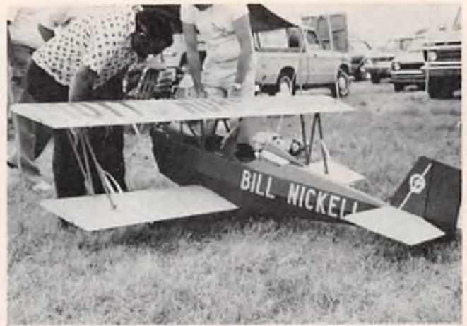
Nosen Gere Bipe by Bill Nickell. Power Max .80 with Du-Bro prop drive. Weight 24 lbs., wing span 8'. Covered with Permagloss. Hand carved pilot (foam). Two servos on elevator. Aileron and rudder mixed for coordinated turns. Flew superb!
