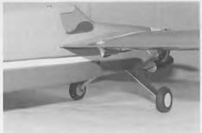
Landing gear position lends itself to good ground handling.
