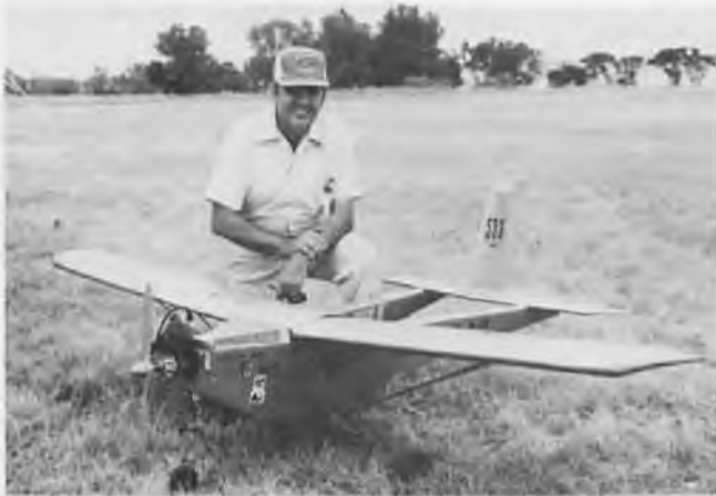
T.G. McNeely (45) from Oklahoma City, Oklahoma. Original aircraft called "Bee Boo" or "Big Bird". Powered with a Quadra 18/6 prop (air flow), weight 23 lbs., wing span 97", covered with Coverite. Finished with acrylic enamel. Unique features include loud speaker aboard and speaks to crowd over 2M-FM. Pulls banners, drops toilet paper (up to 3 rolls one at a time). Drops paratroopers - up to 6 on command or 1 at a time. Built of cardboard and wall paneling. WOW!
