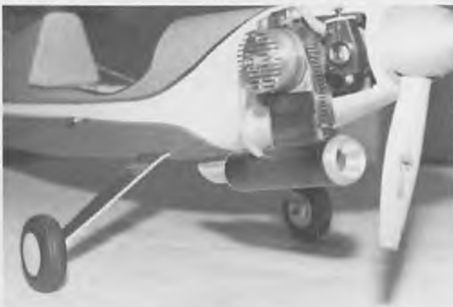
Completed nose section showing side mounted K & B .40 with Semco muffler.
