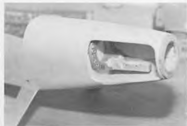
Nose section showing CB aluminum mount installed.
