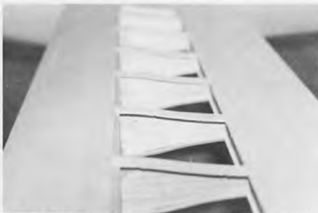
View of wing panel showing reflex. Note cross grain capstrips.
