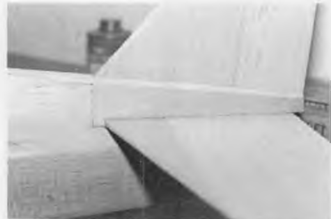
Close-up showing fin and stab installed.
