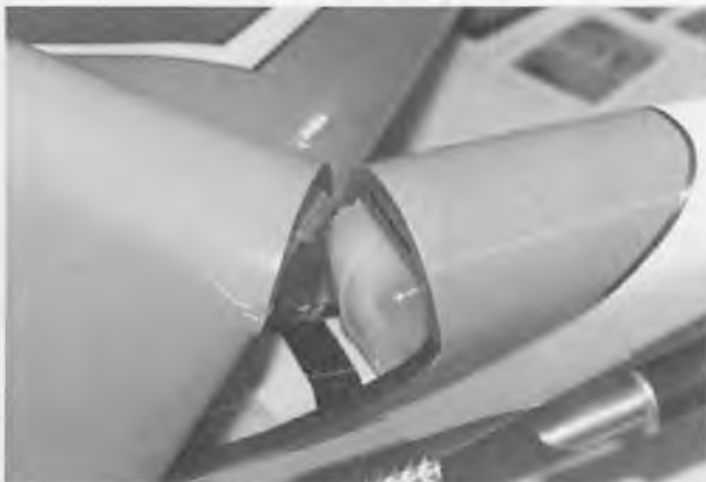
Plywood tongue fits into slot in forward bulkhead.
