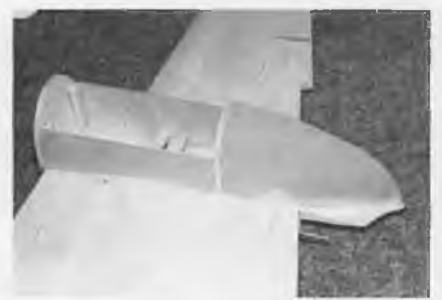
Micro-balloon filler at stationary section between flaps.
