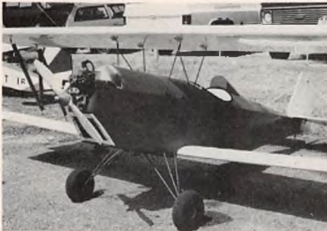
Nosen Gere Sport , built by Garland South (55) from Cleveland, Oklahoma. Powered by modified McCullen chain saw engine. 18/8 prop, weight 25 lbs., wing span 96". Covered with Sky Loft and MonoKote. Modified his own engine. Tail wheel is Tatone nose gear for .19 size plane.
