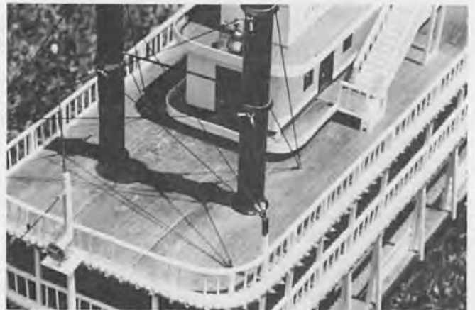
Most of the details are functional (spot light and bell shown in this photo). Decks are made of basswood, used by model railroaders for house siding.
