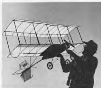
Here is Johnny Litchenburg of Historical Aircraft Research & Development Co. in Kansas, with his replica of the #3 version of the Chanute Glider of 1886 - but with a power pod & wheels added. Johnny builds many replicas for museums around the country - and covers them with good old Coverite.
