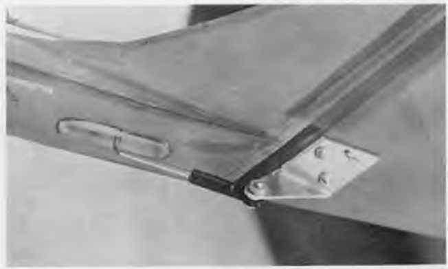
Detail of control horn on rudder.
