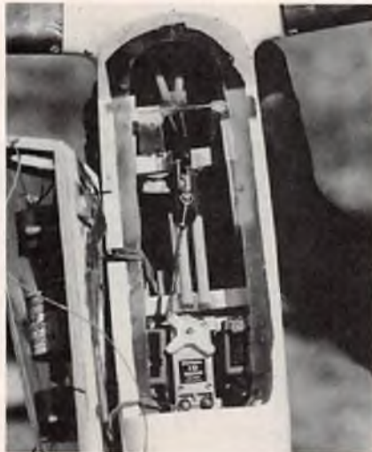
Dave Peltz uses slider on fiberglass tubes for smooth spoiler action.
