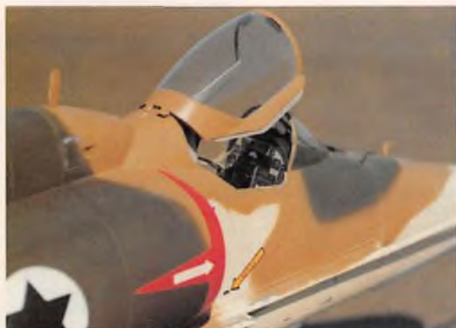
Looking into cockpit with canopy raised. Complete instrument panel and gunsight on glare shield.
