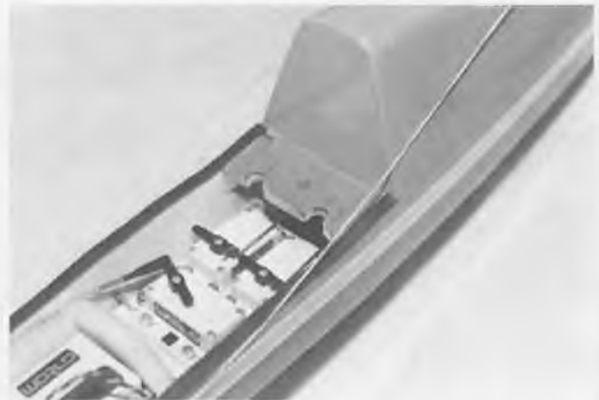
Servo installation is tight but sufficient.
