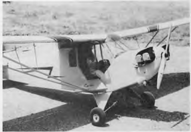
Clipped wing Nosen Cub by Wendell Roberts and Terry Dench (43 & 29) from Little Rock, Arkansas. Quadra powered 16/6 prop, weight 17 lbs., wing span 7' 10". Covered with Coverite and finished with K & B Super Poxyl. Completely detailed after actual full size aircraft hangared at Batesville, Arkansas. Excellent interior detail. Flew well.
