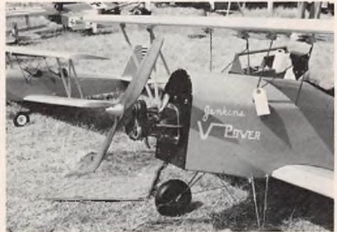
Nosen Gere Sport , built by Kenny Jenkins (Lazy Ace in near ground) of Jenkins R/C Aircraft Inc., North Kansas City, Missouri. Powered by special engine drive - Jenkins V power, two Kraft .61's mounted to a reducer 1.9:1 ratio turning a 24/10 prop at 6,000. Jenkins plans to market this drive, with engines, in the near future. Engine sounded like a twin when opened-up.
