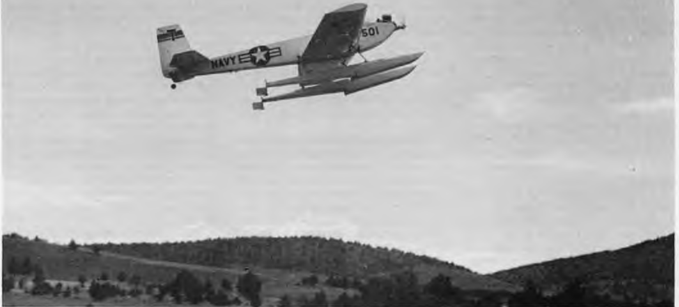
Dick Hansen's floats on his modified Taurus. Optional water rudders were connected to rudder horn.
