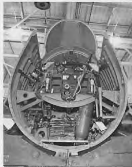
An F2G fuselage separated on the major seams just below the cockpit rim and at the headrest. This part is shaped the same on both the F4U and the F2G. (Photo by Goodyear Aircraft.)
