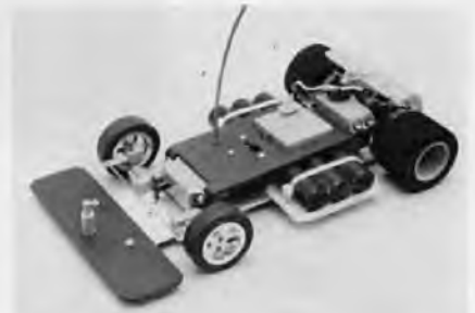
The top of the MRP line, also from Jo Mac is the model #929. This car features the MRP chassis with Jo Mac radio and resistor type speed control.
