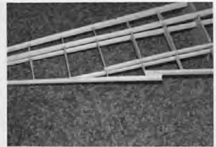
Detail of 1/4" sq. spar between W7 and W8.
