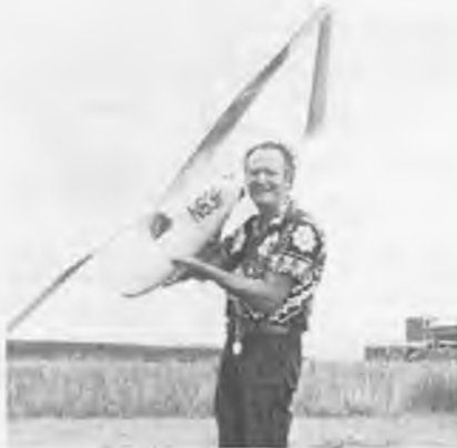
This is the Ihex, a Stan Hall design, built by Gordon Pearson, President of the LSF. The Ihex was photographed at the SOAR Nats. It was covered by Gordon in Super Coverite, painted with K&B Superpoxy. Span 147".
