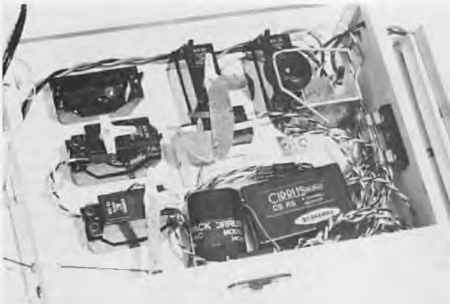
The radio compartment houses a Hobby Shack Cirrus radio operating a maze of clever mechanisms.
