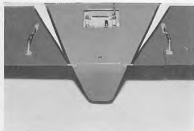
Close-up of notch in rear of wing for removal.
