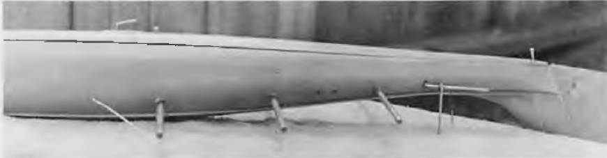
View of hatch showing tow hook and hatch hold-down bolts.
