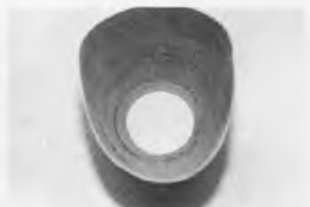
Cowl with foam removed and opening cut in FW4.
