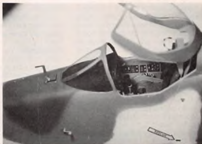
Ejection seat, control stick, and R.H. switch console can be seen inside cockpit. Angle of attack sensor, pitot tube, and windshield blower are details on nose.
