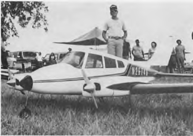
Don Apostolico's, from Broken Arrow, Okla., Nosen Cessna 310 twin Webra .61's, 11/8 props. All up weight 28 lbs. Wing span 10' 2". Covering and finish - MonoKote and Super Poxyl enamel. Pro-line retracts - gear drilled out to accept 3/16 wire struts - Sonic cylinders. 8 servos and flaps. Looked super in the air. Flew with engine cowls removed. Won Most Impressive and Outstanding trophy.
