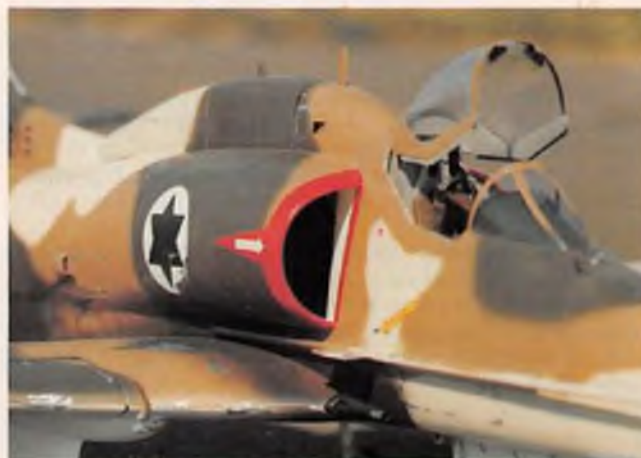
Hump back to house electronic gear is distinctive Israeli feature. A myriad of details are seen in this photo. Weathered finish and 20mm gun powder burns are authentic.
