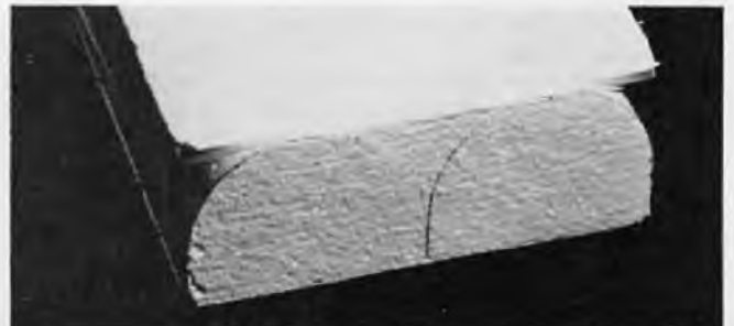
With the parts from the first cut stuck lightly in place with transfer tape, the end shape is cut.
