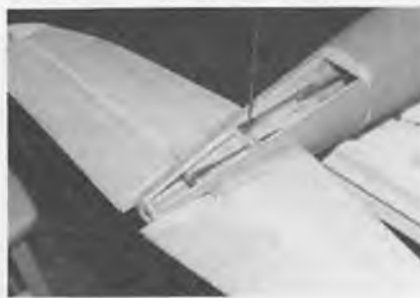
Pushrods in place - rudder view.
