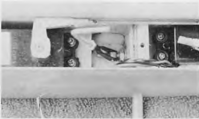
Swivelling tow hook mechanism.
