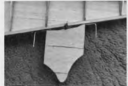
Stationary section between flaps and control horn.
