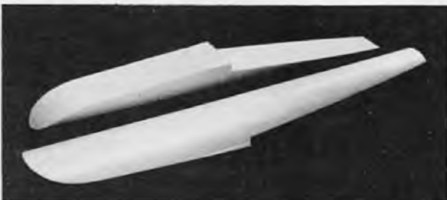
Two foam cores are easily made with only two hot wire cuts.
