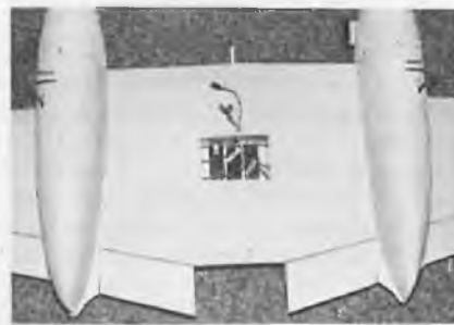
Servo installation in wing for throttle, aileron and flap.
