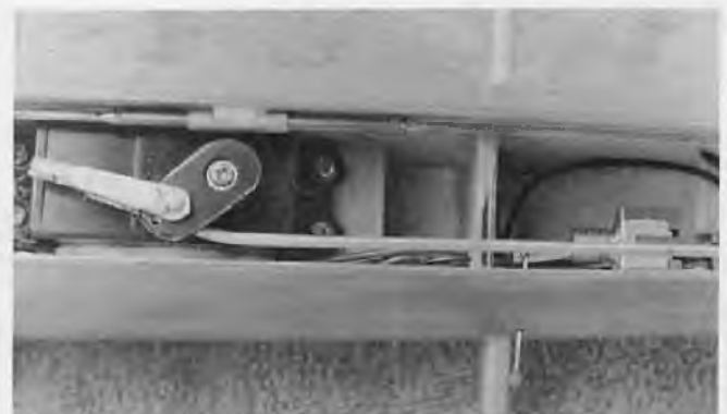
Differential elevator drive detail. Servo arm in level flight position. Note reversed clevis and bend in pushrod for clearance.
