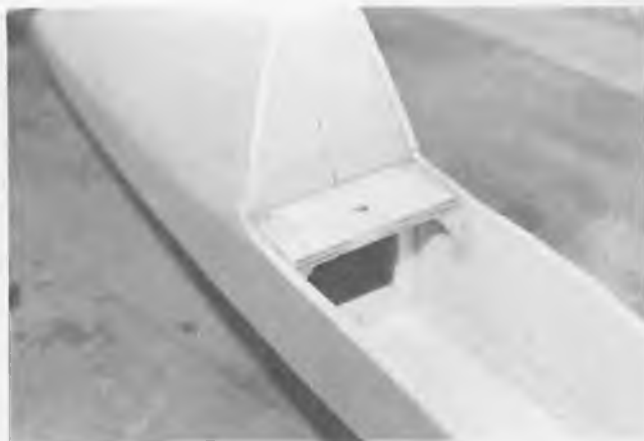
View of rear wing hold-down plate.
