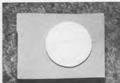
FW4 cemented to foam block.
