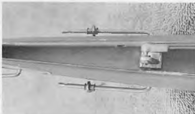
Elevator drive showing cast aluminum boat tiller - Strong!
