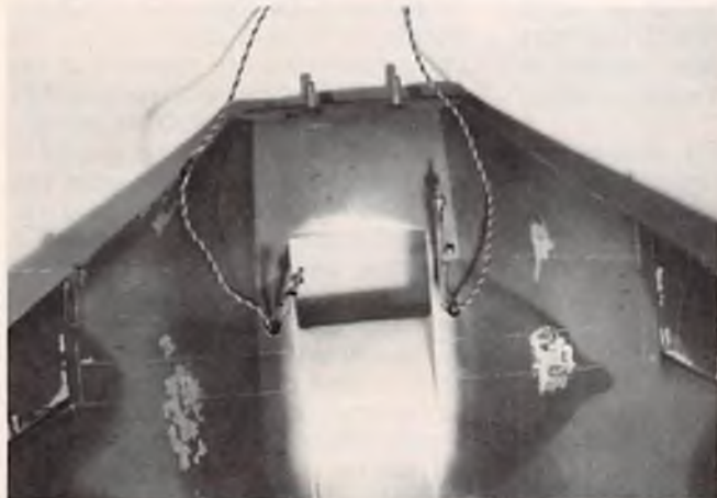
Top center of wing shows auxiliary air intake for ducted fan. L.E. slat detailing can be seen. Pneumatic lines for retracts and servo leads enter fuselage.
