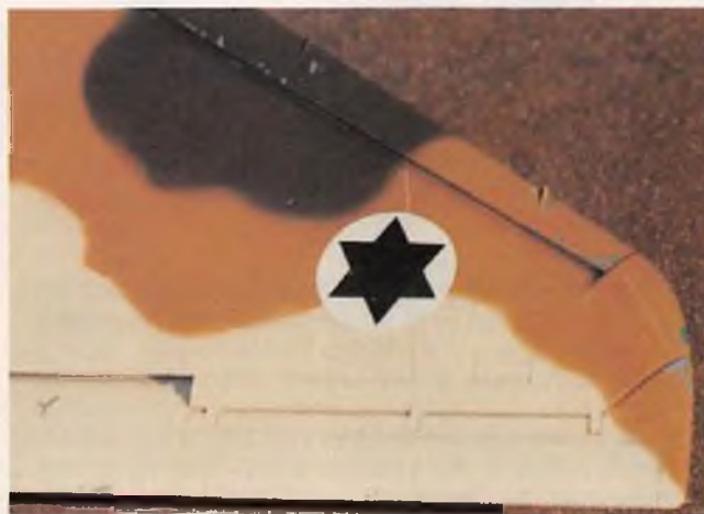
Leading edge slat appears to be open but actually uses air brushed shading to create the illusion. Paint chipping and color feathering are clearly shown.
