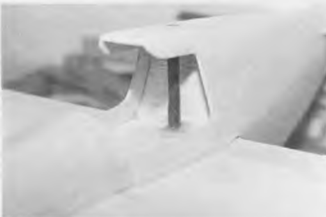
Guide tube for wing hold-down screw.
