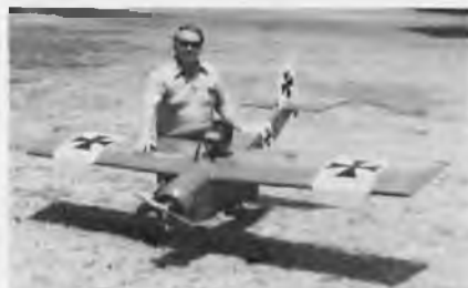
Chuck's Eindexer, 8' 8" span 16 lbs. Webra .91 power, designed & built in 8 days for Jumbo Fly In.
