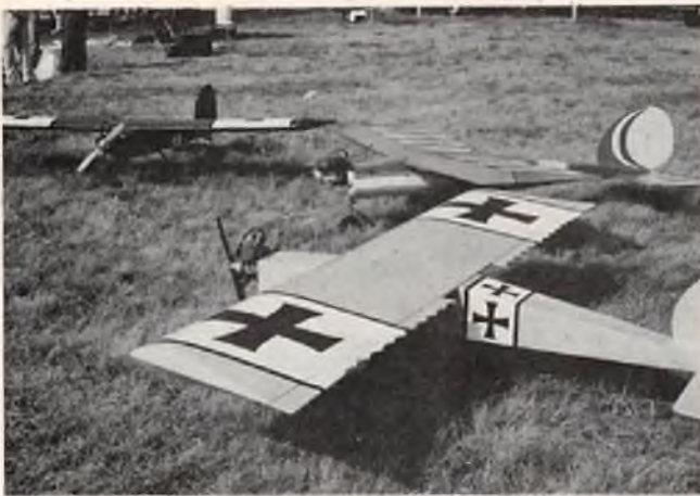
"Super Stick" a design effort by Morrall and Pringle of Tulsa, Oklahoma. Members of Tulsa Glue Dobbers. Aircraft powered by Quadra, 18/6 prop, weight 35 lbs., wing span 8' 6" (2400 sq. in.). A Phil Kraft Ugly Stick enlarged 1.7 times. 1/8" ply and foam construction. Balsa tail construction trainer for Quadra. Morrall and Pringle plan to kit this bird with landing gear kit, wing kit and fuse kit available. Plans will be available in 3 months. Kit priced between $150.00 and $175.00.
