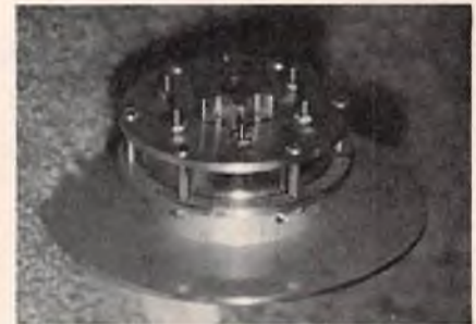
(L) Disc will be attached to other side of housing. Thick alum. collar already bolted to it. Collar will act as mount for 3/4" steel winch hub end and be used to mount 6" hub flanges. 3 set screws are mounted in collar and will set into holes in winch drum. (C) Previous assembly but hub flange attached. Flange is 1/8" thick alum. plate and held in place with 3 countersunk screws. Groove machined in face of disc will mount on clutch housing. Groove holds assembly concentric with engine crankshaft. (R) Disc assemblies are clamped to clutch housing using 6-32 machine screws. Screws have their tension adjusted slightly to align winch drum shaft with crankshaft. Assembly must be completed at this point on engine with clutch housing held in place with clutch shoe assembly.
