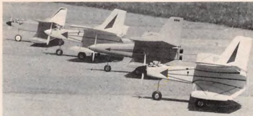
At left Astron (K & B .21 powered). Right three are the larger K & B .40 powered version. Successful formation flying with these look-a-likes is an accomplishment.
