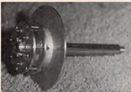
(L) 3/4" steel winch drum hub in place and held with set screws. The far end of the shaft is machined smaller to fit the support bearing used at that end. (C) Other flange is attached to 3/4" steel hub. Flange has a thick alum. collar attached with 3 countersunk screws and collar is held firmly on shaft with 3 set screws placed into depressions drilled in shaft. If depressions are not used, fine forces will squeeze the flanges from the hub. (R) Exploded view of all the parts and their relative positions to engine. All that remains now is final assembly and a base so far bearing can be aligned with engine.
