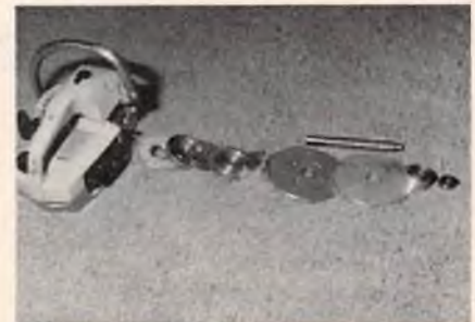
(L) 3/4" steel winch drum hub in place and held with set screws. The far end of the shaft is machined smaller to fit the support bearing used at that end. (C) Other flange is attached to 3/4" steel hub. Flange has a thick alum. collar attached with 3 countersunk screws and collar is held firmly on shaft with 3 set screws placed into depressions drilled in shaft. If depressions are not used, fine forces will squeeze the flanges from the hub. (R) Exploded view of all the parts and their relative positions to engine. All that remains now is final assembly and a base so far bearing can be aligned with engine.
