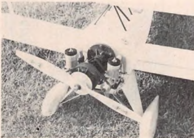
Two Rossi .60's on a Byro Drive. Custom engine mounts and front pulley besides engine arrangement presented an unusual challenge for the builder.
