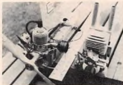
O & R and Super Hustler side by side. O & R is much smaller and a great deal lighter. Hopefully it will fill the gap between large glow engines and the 2 C.I. gas engines.
