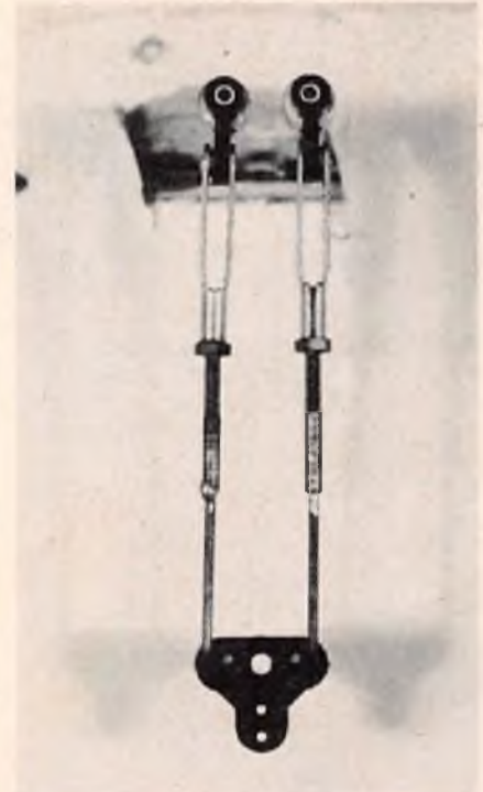
Aileron linkage in Miss Norway. Short pushrods do not create any installation or operating problem.
