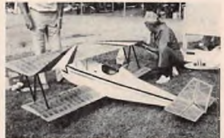
Gere Sport by Darrell Neyland. Quadra powered, MonoKote covered. Darrell hails from Austin, Texas.
