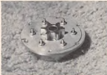
(L) Bell housing drilled and holes countersunk to accept flat head machine screws. (C) Alum. disc mounted to housing with bolts. Inner side of disc was relieved in center to allow it to seat on the conically shaped housing. A lathe was used, the same effect could be obtained without machine work with a washer between disc and housing on each bolt. (R) Housing and disc from other side. Holes around the perimeter of disc will be used to sandwich housing to a disc on the other side.
