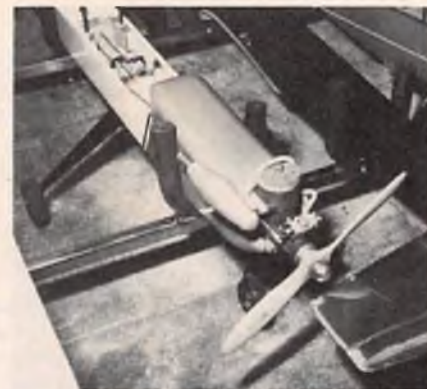
Padding for cradles is soft foam refrigeration insulation tubing.
