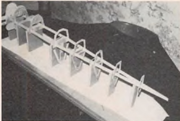
3) Frame ready for landing gear mount and floor board.
