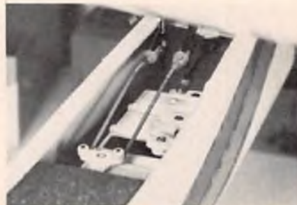
View with wing raised. Servo arm is put on servo, retaining screw installed, wing dropped down and secured.
