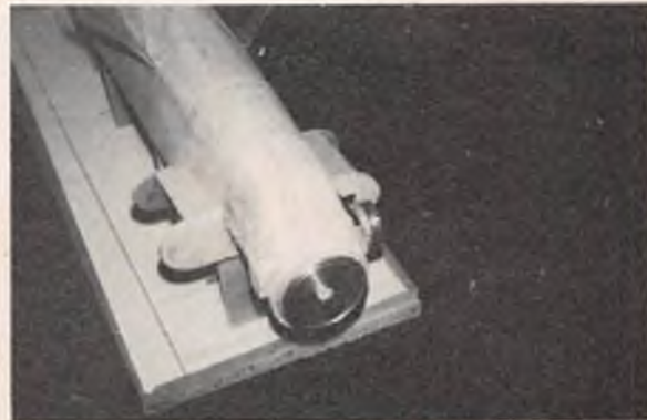
8) Chin blocks complete, whittled and sanded ready to remove spinner back plate.
