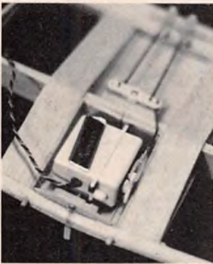
Close-up of aileron servo. Note servo board hold down screw in front.
