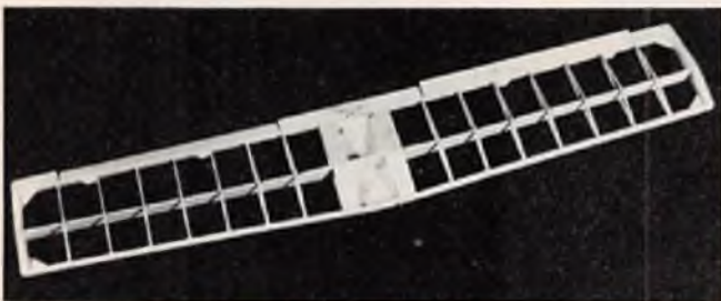
Completed wing awaiting servo installation. Wing is lighter and stronger than sheet rib type.
