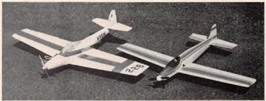
Small R/C airplanes often require many techniques all their own. "Li'l Cobra" Quarter Midget and Half-A "Miss Norway" shown use servo mounting/attaching techniques described.
