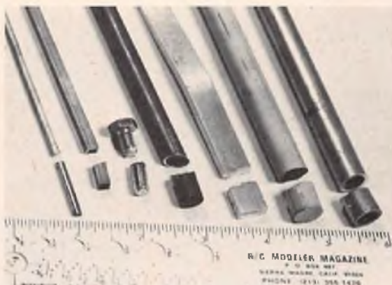
Materials cut for our test were (L to R): 5/32" music wire, square brass tubing, 3/16" steel bolt, 3/8" dia. steel tubing, 3/16" x 1/2" aluminum bar stock, 1/2" dia. maple dowel, and 1/2" dia. thick wall stainless steel tubing.
