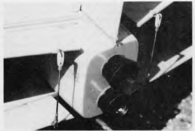
Aft view showing elevon linkage to top wing. Servos located in lower wing. Tailpipes add to looks.
