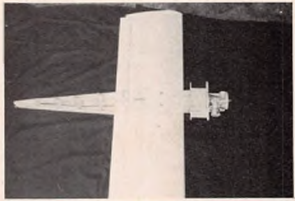
18) Top view of wing after being fitted, hold-down holes drilled and tapped. First time bolted down.
