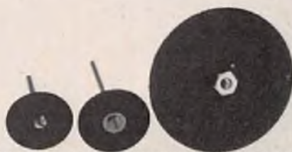
A 1" abrasive cutting wheel is shown on left, the 1" HOB Tuf-Grind in center and the 2" Tuf-Grind at right. With any cutting tool, caution must be used to let the wheel cut, do not try to force it.
