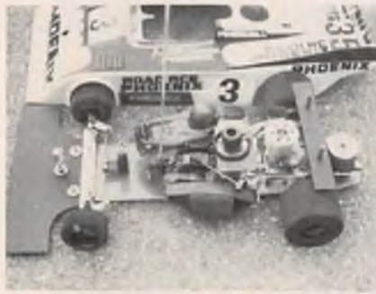
(L) Naoki Ishihara, Japan, was Top Qualifier in both sessions with Phoenix Road Ace car. (C) Ishihara's car is a very basic designed car featuring light weight, O.S. Max 21 ABC engine with McCoy type muffler and Sanwa radio. (R) Curtis Hustling was 2nd qualifier in the first round, won 2nd Semi Main by 2 laps over Phil Booth and was running away with the Main Event when his flywheel locked up.
