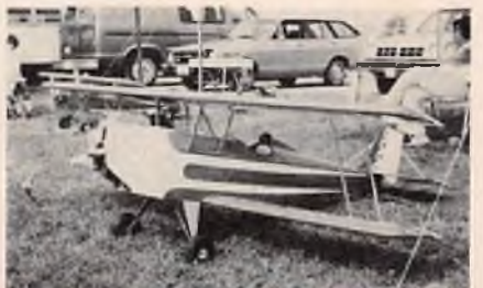
Gere Sport built and flown by Garland South of Cleveland, Oklahoma. Powered by McCulloch chain saw engine.
