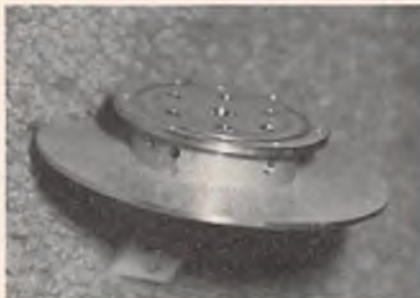
(L) Disc will be attached to other side of housing. Thick alum. collar already bolted to it. Collar will act as mount for 3/4" steel winch hub end and be used to mount 6" hub flanges. 3 set screws are mounted in collar and will set into holes in winch drum. (C) Previous assembly but hub flange attached. Flange is 1/8" thick alum. plate and held in place with 3 countersunk screws. Groove machined in face of disc will mount on clutch housing. Groove holds assembly concentric with engine crankshaft. (R) Disc assemblies are clamped to clutch housing using 6-32 machine screws. Screws have their tension adjusted slightly to align winch drum shaft with crankshaft. Assembly must be completed at this point on engine with clutch housing held in place with clutch shoe assembly.
