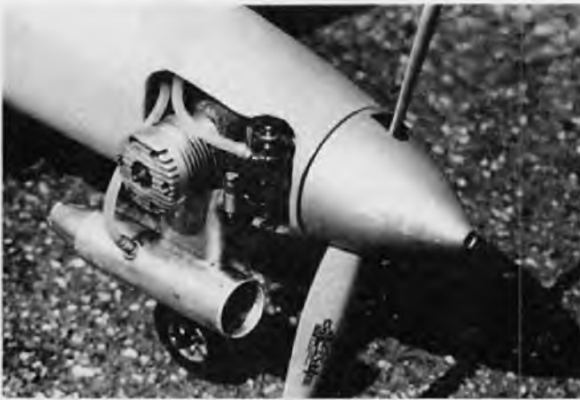
Side mounted K & B .40 with Zinger 10/6 prop and CB spinner. Tank is pressurized for maximum output.
