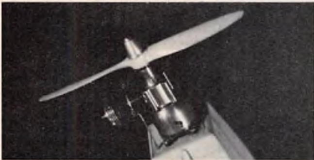
Simple throttle 'hook-up' works well on Cox Golden Bee if engine is well 'broken in' before attempting complete throttling.
