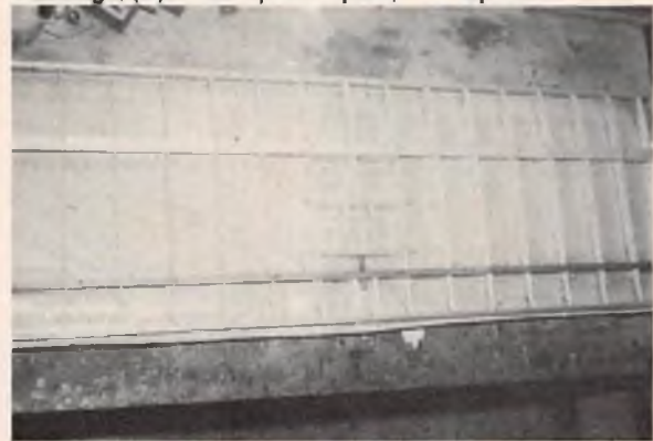
14) Wing ready for top sheeting.
