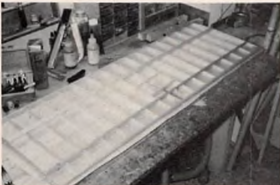
15) The wings top sheeting is complete. Wing has been turned over and is ready to have its bottom skin applied.
