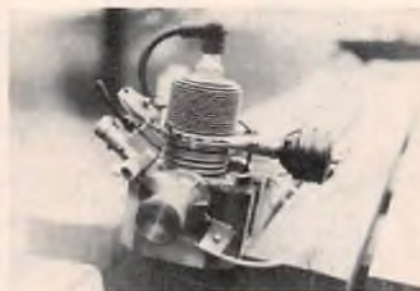
O & R engine converted to Model power. Engine is beam mounted, throttles down to 1100 rpm from a peak of 5200 with 18/6 prop.
