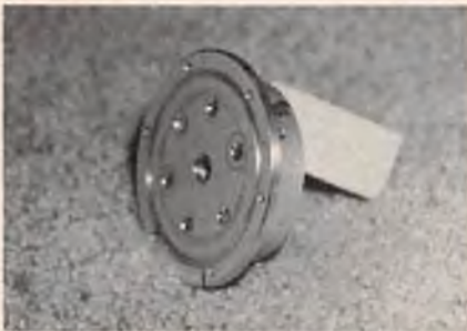
(L) Disc will be attached to other side of housing. Thick alum. collar already bolted to it. Collar will act as mount for 3/4" steel winch hub end and be used to mount 6" hub flanges. 3 set screws are mounted in collar and will set into holes in winch drum. (C) Previous assembly but hub flange attached. Flange is 1/8" thick alum. plate and held in place with 3 countersunk screws. Groove machined in face of disc will mount on clutch housing. Groove holds assembly concentric with engine crankshaft. (R) Disc assemblies are clamped to clutch housing using 6-32 machine screws. Screws have their tension adjusted slightly to align winch drum shaft with crankshaft. Assembly must be completed at this point on engine with clutch housing held in place with clutch shoe assembly.
