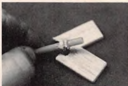
The balsa broke when we tried to remove the NyRod. Note that the adhesive did not separate from the NyRod.
