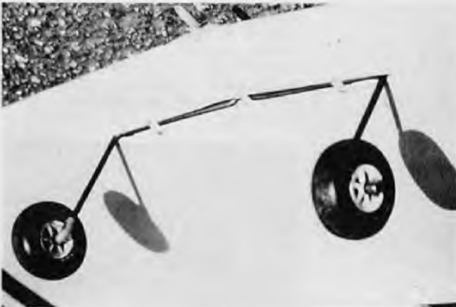
Conventional mounting on fixed main gear. A set of retracts would be fantastic.
