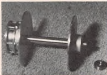
(L) 3/4" steel winch drum hub in place and held with set screws. The far end of the shaft is machined smaller to fit the support bearing used at that end. (C) Other flange is attached to 3/4" steel hub. Flange has a thick alum. collar attached with 3 countersunk screws and collar is held firmly on shaft with 3 set screws placed into depressions drilled in shaft. If depressions are not used, fine forces will squeeze the flanges from the hub. (R) Exploded view of all the parts and their relative positions to engine. All that remains now is final assembly and a base so far bearing can be aligned with engine.
