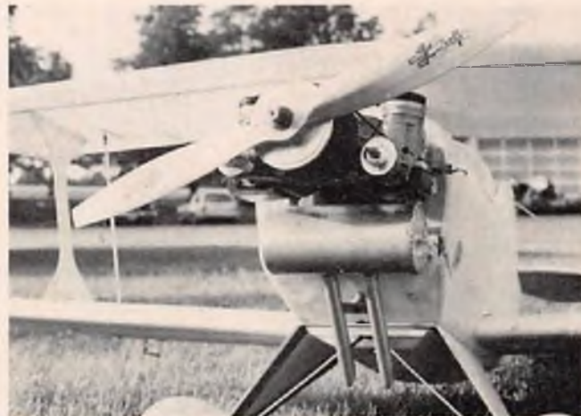
Two engines piped into special muffler making it difficult to tell when both are lit up. Note pressure lines for each fuel tank and support of exhaust pipes.
