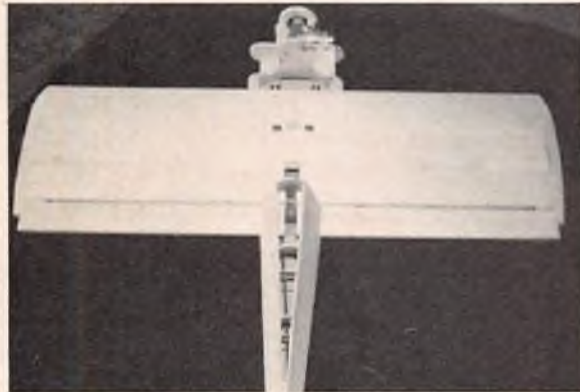
19) Here we see the side sheeting of the turtle deck being fitted to the fuselage and around the trailing edge of the wing.
