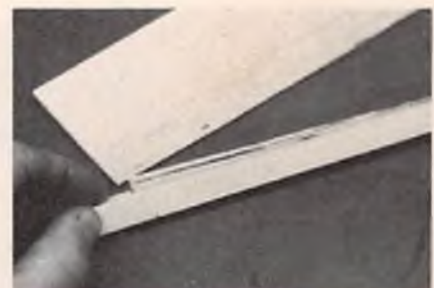
A bead of Super Jet applied down length of edge of sheeting, then pressed to 1/2 x 1/2. When we tried to separate the two, the balsa failed.
