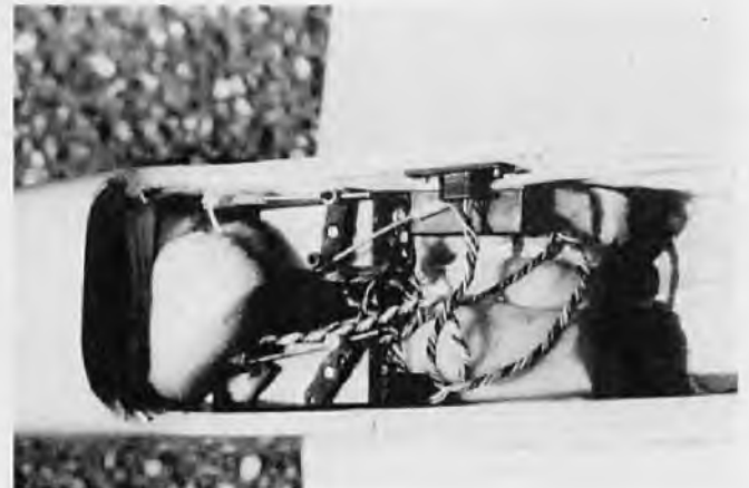
Inside fuselage showing nose wheel and throttle servo. Note linkage going to rudder which was tried on one or two prototypes.
