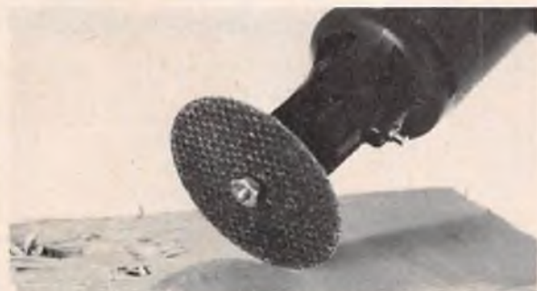
A valuable feature of the Tuf-Grind is its ability to withstand side load shock. We seem to break more solid abrasive wheels by bumping them on the work bench than any other way.
