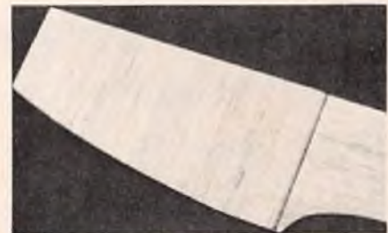
Doubler glued in place.
