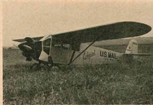
Fairchild FC-2; scratch-built by George Clapp, Syracuse, N.Y. --- Wingspan, 88" --- weight 11 lbs. --- powered by an O.S..60F SR.
