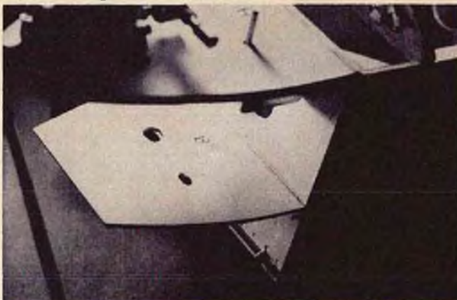
Former "B" is base for battery pack and receiver. Note fuel tank vent and filler tubes thru former "A".
