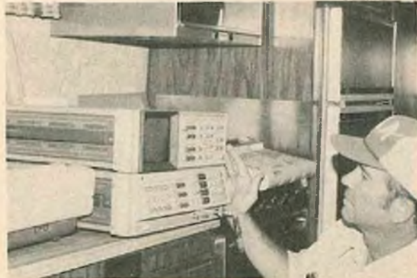
Transmitter frequencies were monitored with HP 8566 Spectrum Analyzer, with plotter and desk top computer.
