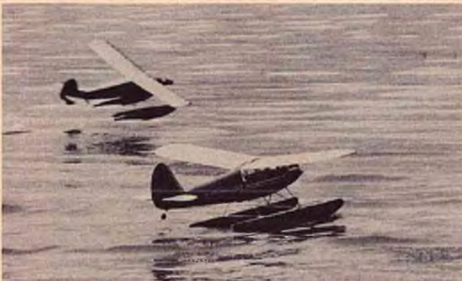
Jim Drever built and flew this TD-Coupe originally published in Model Airplane News in 1936. Jim's model was built from Model Builder plans weighing in at 5½ lbs. with an O.S. .30.
