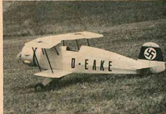
Bucker Jungmeister, built from a Platt kit by Al Pollicano, Erie, PA --- Kraft Radio --- Powered by a Maximizer geared 4-cycle O.S. 60. Al is a pilot for USAir.
