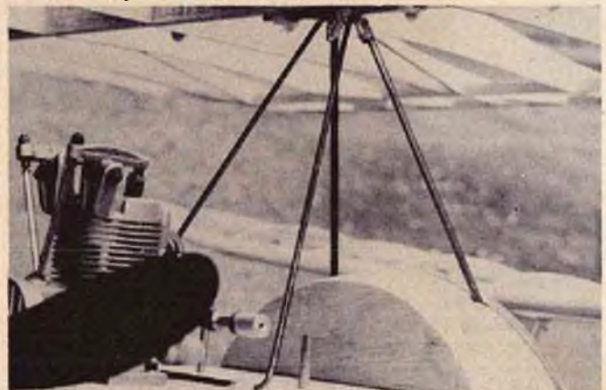
Close-up of cabane struts showing the pivot attachment to the wing. This system works very well.
