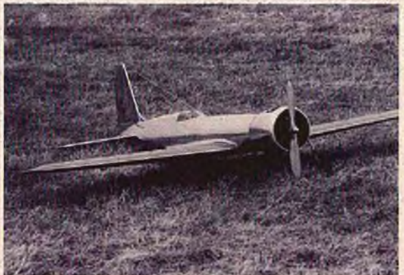
Hughes H-1 --- scratch-built by Bruce Knox, East Aurora, N.Y. --- weight 5½ lbs. --- powered by ST .60 Saturn --- swings 12 x 6 prop --- Kraft radio.
