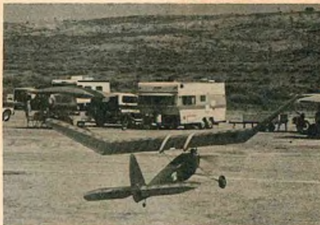
Contest Manager Al Hellman's Lanzo Record Breaker was a Texaco entry. Powered by an O.S. .60 4 cycle. Red, white, and blue silk covering.
