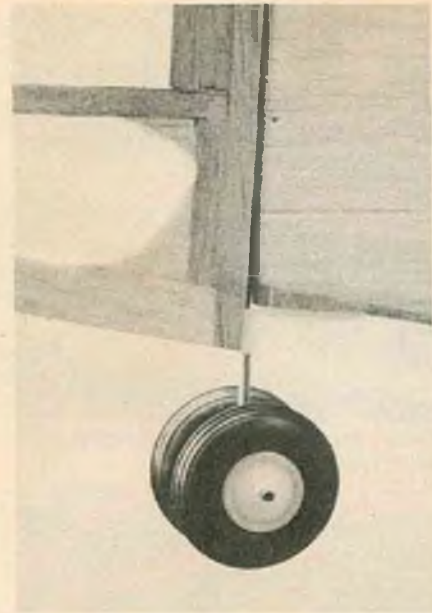
Rudder and tail wheel assembly installed to fuselage.
