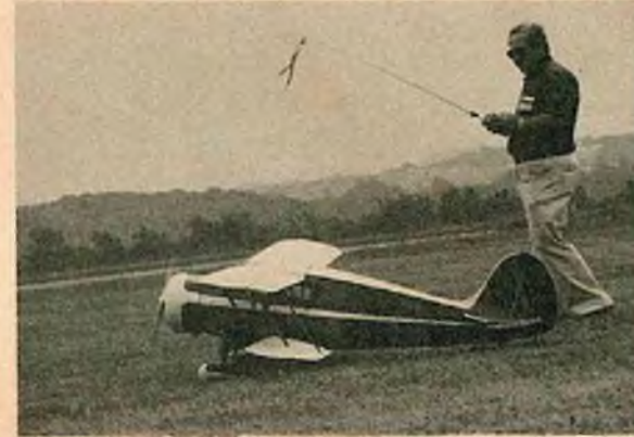
Norm Rosenstock, Plainview, N.Y., with his scratch-built Waco HKS-7 Cabln Bipe --- weight is 33 lbs. --- Powered by a Kawasaki 3.5 engine.
