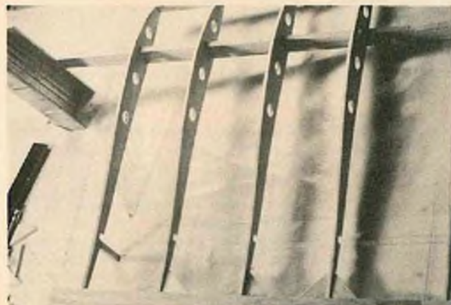
Tip panel is completed, making sure T/E stock is straight and true.
