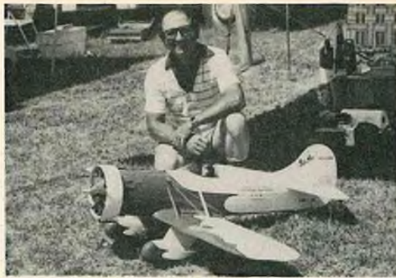
Tom Weems from Hereford, Texas, with his beautiful 10 1/2 lb. 1/4 Scale GeeBee Model-E. Scratch-built from photos with Webra .91 turning a Top Flite 14/6 prop.
