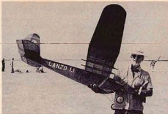
Dave Bruner scaled up the Lanzo Record Breaker 10% to make it SAM-legal for a .60 size engine. A nice flying airplane.
