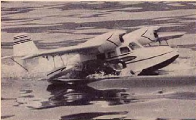
A magnificent "Mr. G's" Widgeon built by Al Mayer. Powered by (2) K & B .61's. It weighed in at 13½ lbs.
