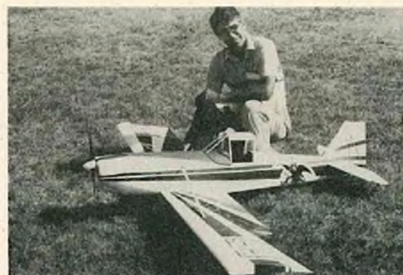
Wendell Roberts' and Randall Snow's 15 lb. Quadra-powered Piper Pawnee. Foam-board fuse with conventional built-up wing. Dynathrust 20/8 prop cut down to 18/8.
