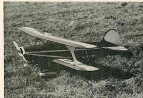
George Paris from Garland, Texas, and his Skybolt from a Dively kit. Powered by Super Hustler MK II, at 30 lbs. (5 lbs. nose ballast.)
