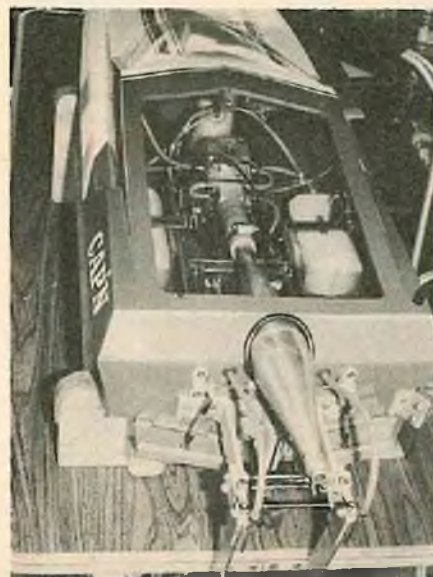
This OPS 90 Deep Vee uses 4 channel radio for throttle, needle valve, rudder and trim plates.
