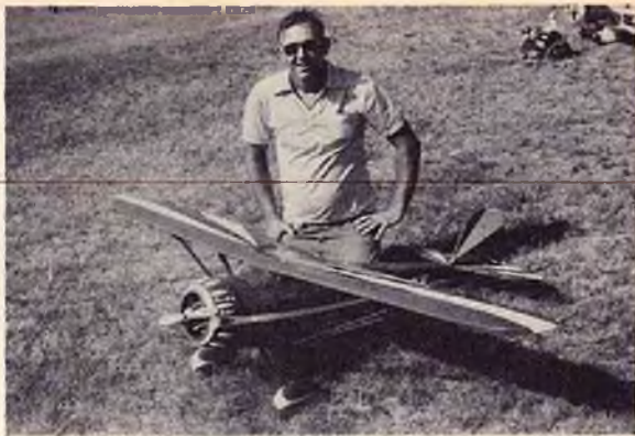
Another Little Rock, Arkansas, entry was Jim Hess' scratch-built Monocoupe. Scaled up from M.A.N. plans, this beauty weighed 13½ lbs. with an O.S. .90 14/5.
