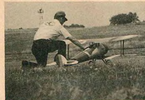
Ralph Jackson, Endicott, N.Y., with his Proctor Nieuport 28 --- weight is 18 lbs., wingspan 80" --- Power is a Quadra.
