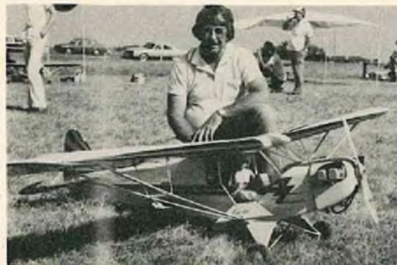
Wendell Roberts' modified (15" off of each wing) Nosen Cub. Quadra powered, 18/6 Dynathrust prop, at 16 lbs.
