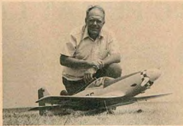
Mahlon Hirsch, Erie, PA, with his scratch-built P-51 --- weight is 10.5 lbs. --- powered by a geared ST-40 --- swings a 15 x 10 prop.
