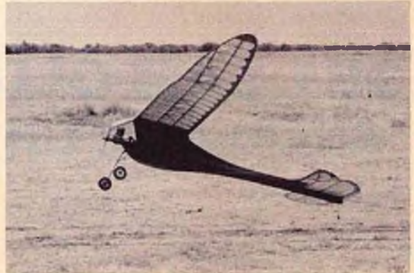
Pete Samuelson flew his 86" span Fotte Westerner in Class B with an Enya .29 and in Class C with an Ignition Super Cyclone.
