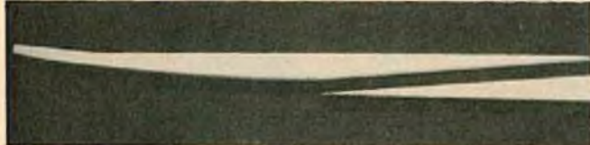
Wing spar should be cut very accurate before final gluing. Check angle against plan layout.
