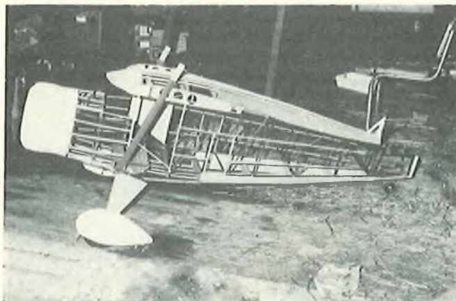
The doctor's 1/4 Scale Stinson Reliant has a welded steel tube basic structure.
