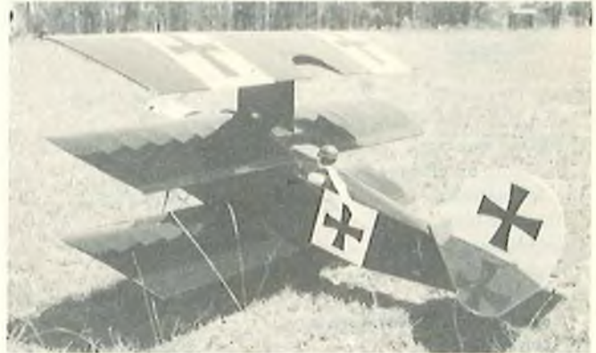
Photo shows a reworked RCM "Basic Bipe" (RCM Plan No. 679) built by N.H. Foote of New South Wales, Australia. Having built several Basic Bipes and ending up with extra wings, Norm put together this Fokker Triplane. Powered by an O.S. .40, it flies very well but could use some additional aileron area.
