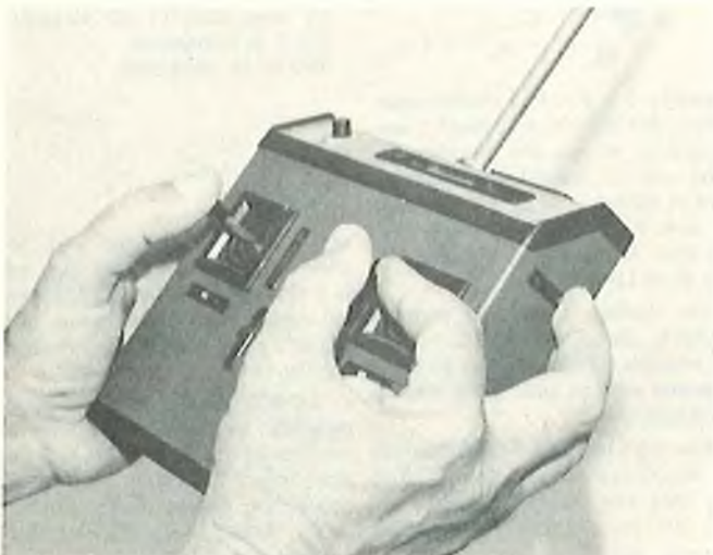
Heathkit eight channel transmitter has two controls on side. Best location for operation without shifting grip. Two lower mounted controls are in awkward position.
