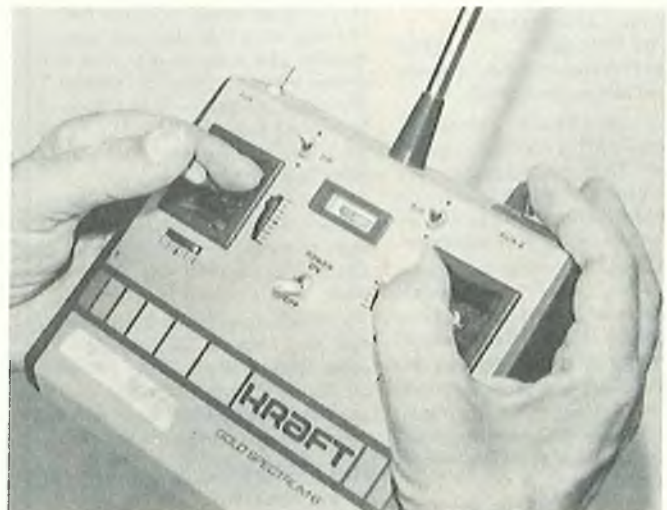
Grip on transmitter must be shifted to operate long throw of aux 2 control on Kraft Spectrum 6.
