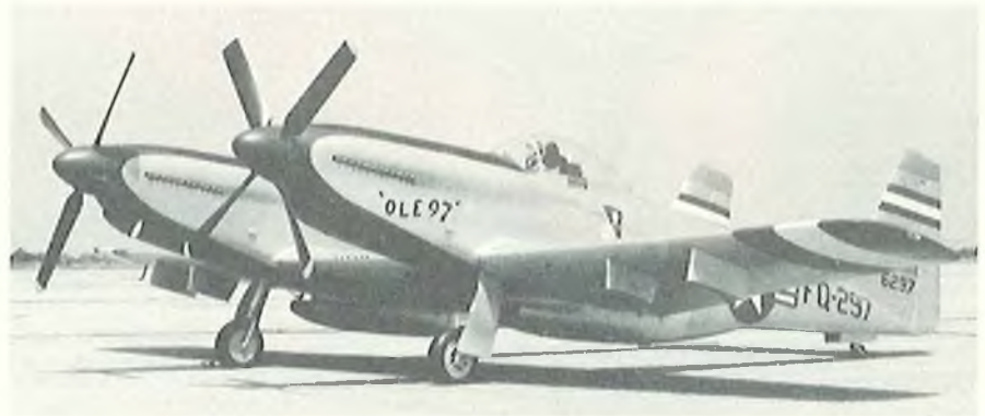
Models of complex aircraft need multi-function R/C transmitters. Art's 1982 National Champion F-82 model requires eight channels with drop tanks.
