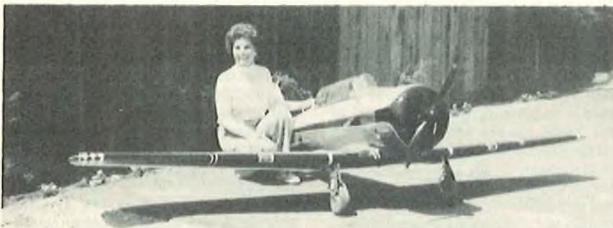
Chuck Fuller of Seaside California, produced this Quarter Scale AT-6 Texan. Will have a few fuselages available. Nice glass work with a built-up wing. The Ziroil T-6 is 1/5 Scale, so Chuck's is noticeably larger. BIG airplane, Kawasaki powered. Mrs. Fuller shows just how big the Texan is at Quarter Scale.
