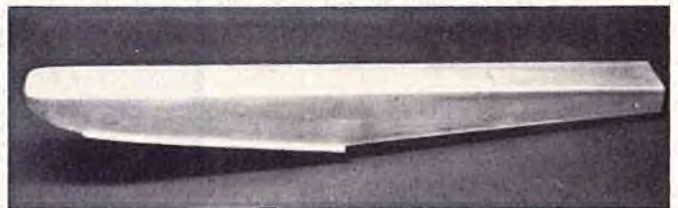
PHOTO 6: Add balsa noseblock and 1/8" plywood transom. Cover floats with 3/4 ounce glass cloth and resin. Glue on 1/4" square balsa spray rail and 1/4" plywood top mounting rail.
