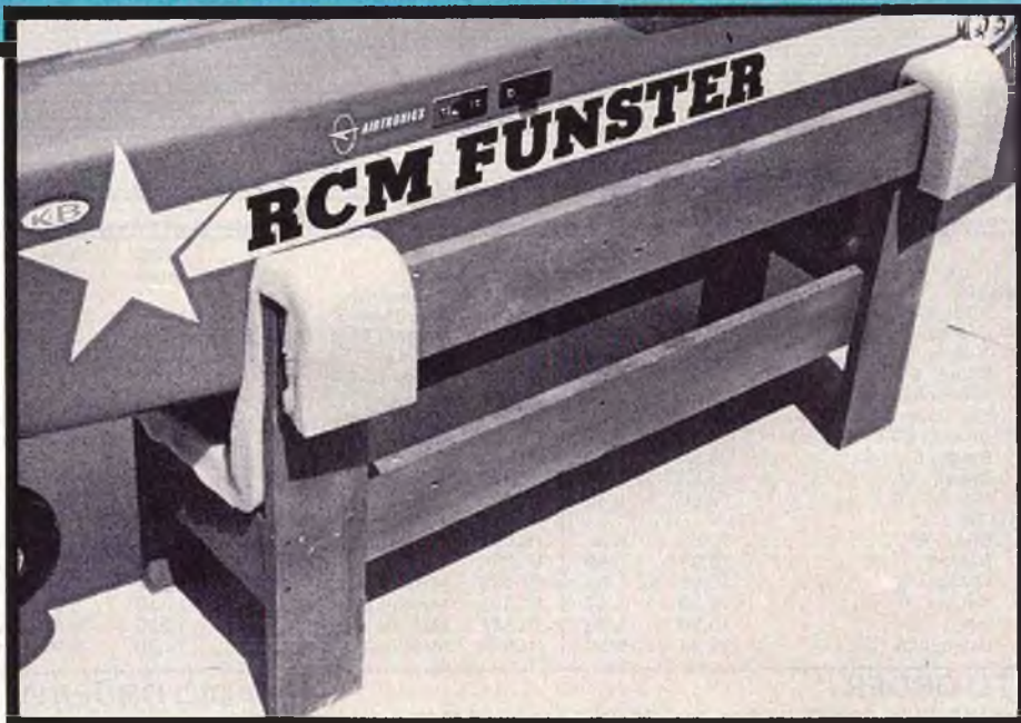
This stand can also be used to allow access to radio from bottom of fuselage. Common poly foam 3/4" thick was glued on for padding.
