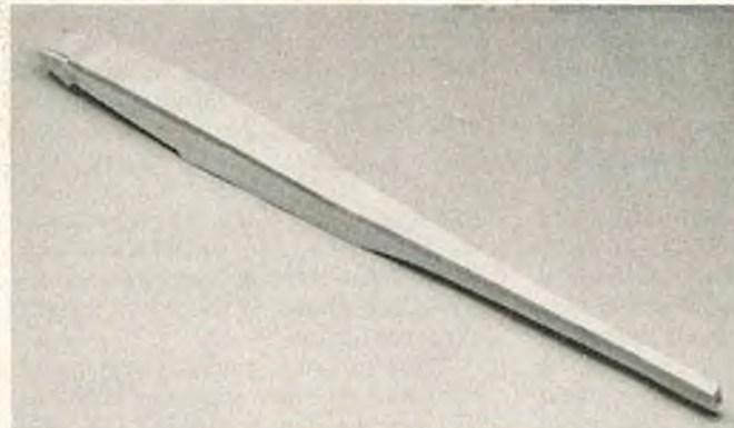
Bottom of fuselage fully sheeted and sanded flush.
