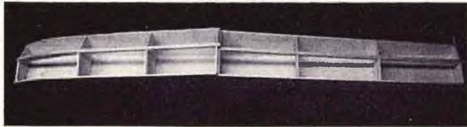
PHOTO 3: Glue on 1/8" balsa float sides and add 1/4" balsa keel.
