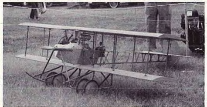
Canadian Colin Wilson's breathtaking pre-WWI Avro biplane. Only three channels (no ailerons!), model is flown by Rudy Mayer when there's absolutely no wind! Quadra powered, Colin used a second Quadra cylinder to provide nose weight and simulate the engine on the "real" Avro.
