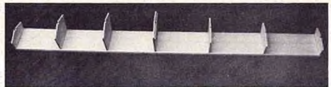
PHOTO 2: Glue bulkheads to 1/4" x 3" balsa top.
