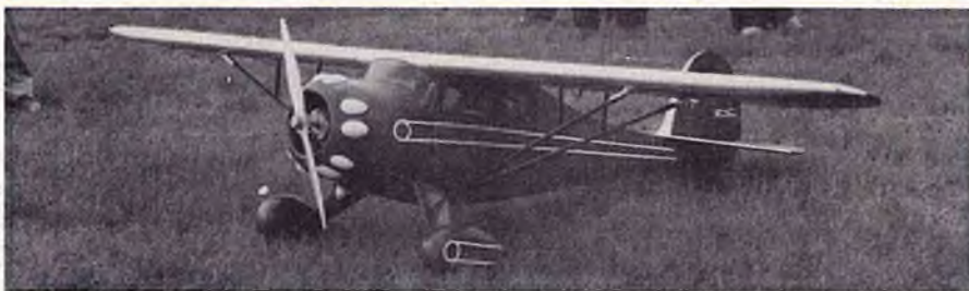
STAR's club member, Bob Dunn's original design 30% Monocoupe 110. Model has piped Quadra for power. In flight, its sound and maneuverability duplicates the prototype, exactly.
