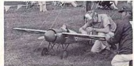
Ray Hinds, of Connecticut, drew his own plans for this 1/3 Scale French Morane Saulnier WW I "pursuit." Dead-on scale, model had prototype's "all flying" stabilizer; Quadra power. Wings warp, too!
