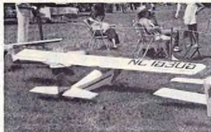
Norm Orcutt's E-2 Cub --- 50% enlargement of RCM drawings, for a Quadra. E-2 was predecessor of much better known J-3.
