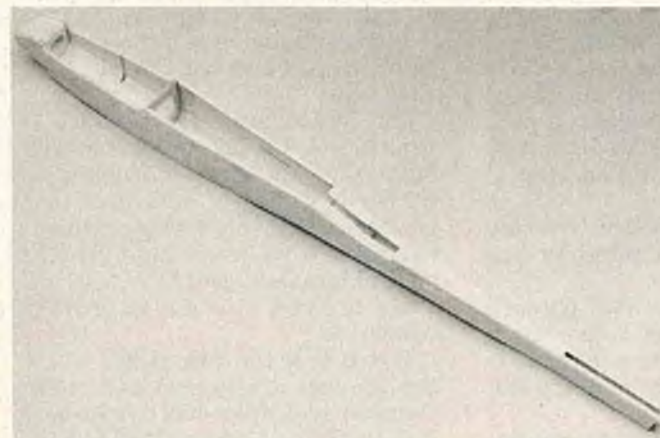
Tail boom top installed and pre-shaped. Be sure to use tail fin to insure correct alignment of slot.
