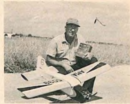
Ben Harr of San Antonio, and the 48" version of his well-known Separator series. 5 1/4 lbs., 380 sq. in., 32 ounce wing loading!
