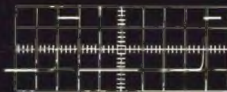
Collector of Q11. 200 us/div. 2 volts/div.
