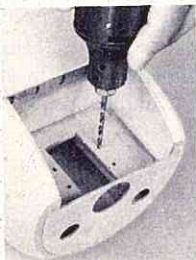
Drill holes for mounting motor and equipment
