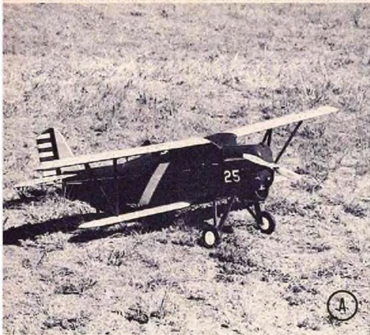
(A) Big, old Enya .60 hangs down into the cooling breeze. Half throttle is more than enough for flight but there ain't no such thing as too much power on a scale ship!
