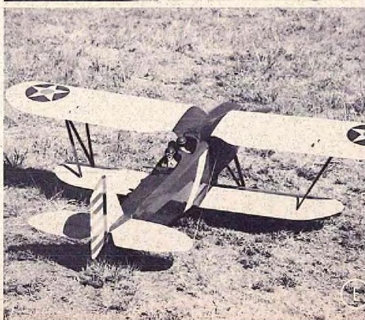
besides, the bird flies OK without a steerable tail skid. The cockpit cut-outs are made in the top fuselage planking and the flexible machine gun mounting block glued in place. After grooving the cowling for the fixed gun troughs (only the barrels protrude), the fuselage is basically completed.
