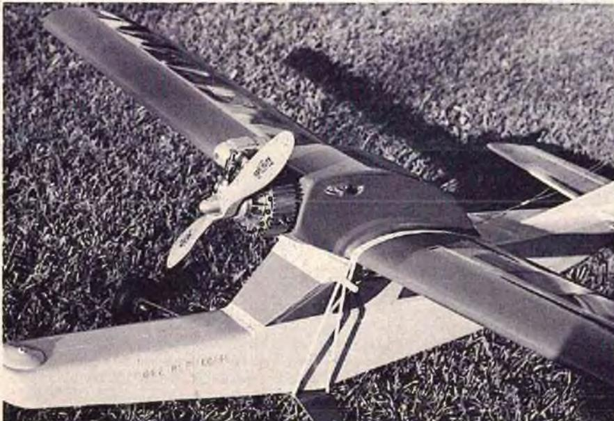
The Mallard is a general sport amphibian produced by the Gee Bee Line, 143 East Main Street, Chicopee, Mass. 01002. Somewhat unusual in construction, the superstructure is conventional balsa and hardwood built on a polyethylene hull which is actually a float. The wing is conventional and built-up of balsa and spruce while the tail surfaces are 1/4" sheet balsa. (Be sure to check the specification and impression charts on page 55 for more detailed information.)
