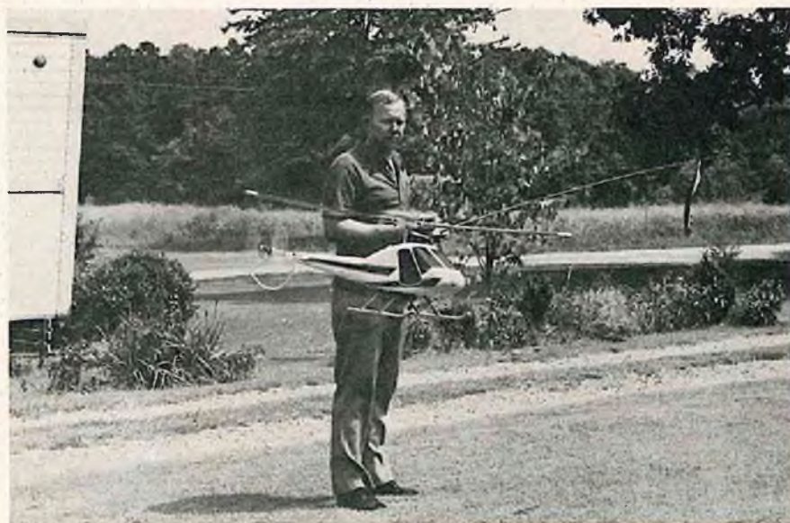
BELOW: The Enstrom configuration requires 2 oz. additional weight in the nose. All flying photos taken within 30 minutes from the first bare Tri-Star shot.
