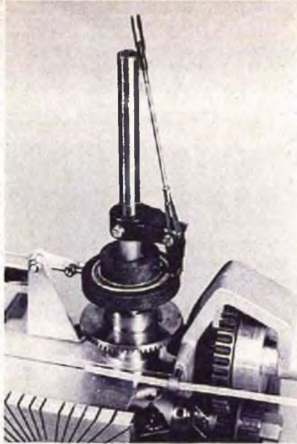
LEFT: The swashplate and scissors installed. Make sure there is no binding in latter. ABOVE: 1/32" ply tail fin added to aid in weather-vaning. ABOVE, RIGHT: Tail rotor gear box and blades installed. RIGHT: Basic head assembly with all bearings in place.
