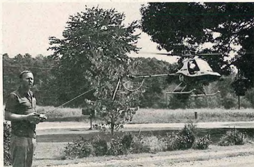
BELOW: The Enstrom configuration requires 2 oz. additional weight in the nose. All flying photos taken within 30 minutes from the first bare Tri-Star shot.
