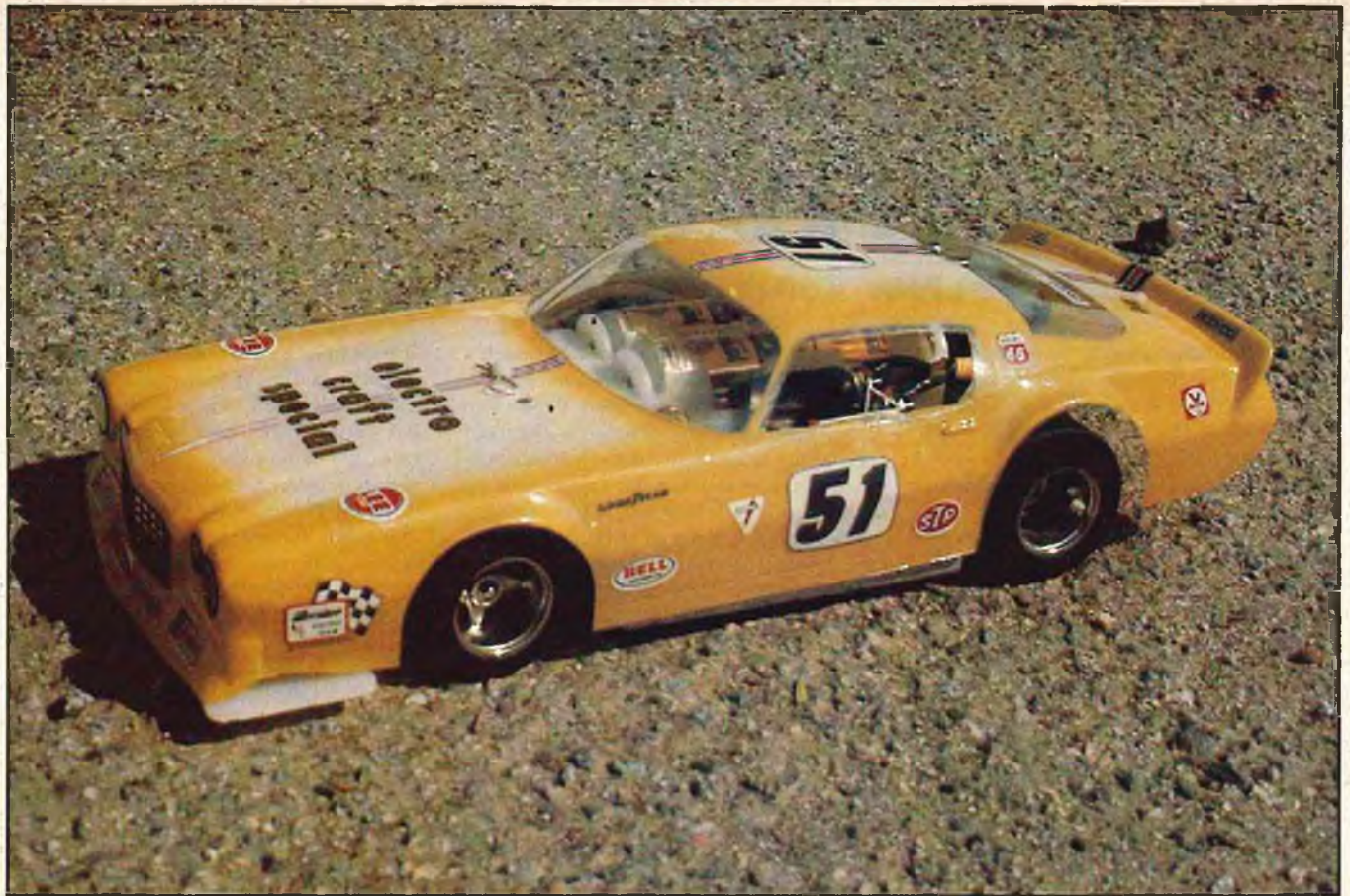
The author's electric conversion of the Jerobee-based car is competitive against 1/12th scale gas cars.
