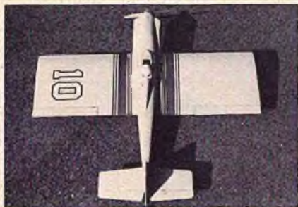
'Flying Dutchman' Cassutt QM racer by Fred Reese. Design was encouraging at first, but proved disappointing with increased engine performance of the Rossi.
