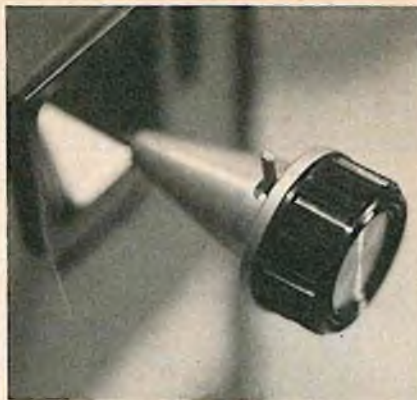
Trim lever installed on Heath GDA-1057.
