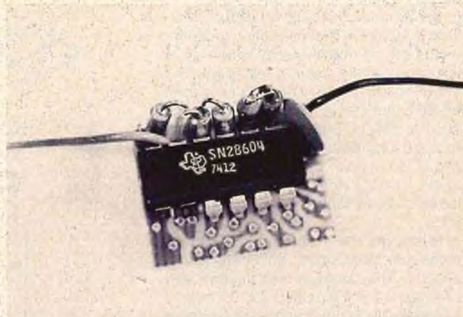
Completing Figure 1 of the instructions, partially filled board shows neat and orderly layout. Installing components in order of sequence is a must.
