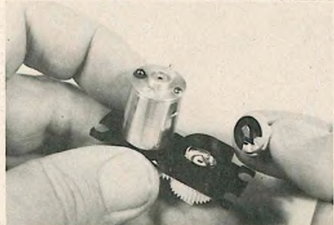
Pot element is lubricated with a special lube available from Royal. Pure Vaseline can also be used. Apply sparingly.
