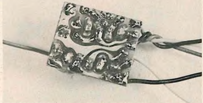
Carefully inspect track side of board to make sure there are no solder bridges or foreign matter between lands. Solder flux is easily cleaned off with dope thinner.
