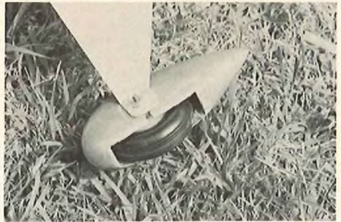
Easy removal of wheel pants for rough field flying.
