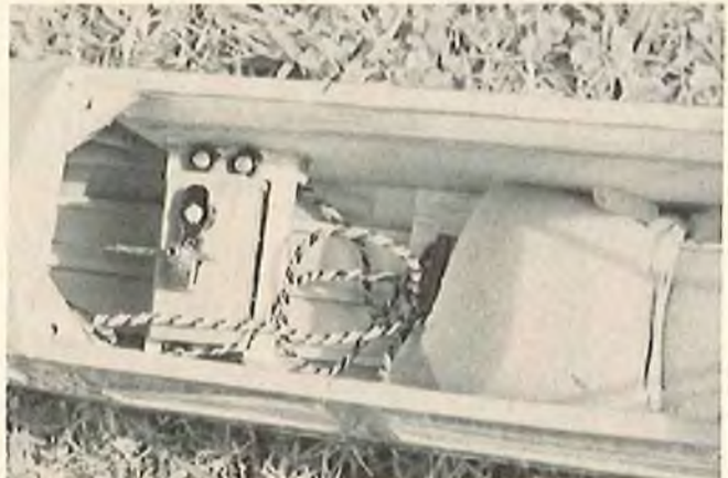
Elevator adjustment made at servo using either Du-Bro or Goldberg pushrod connectors.
