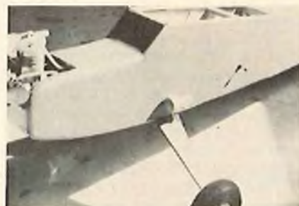
Horn is mounted facing aft to keep engine crud from collecting inside of bell.
