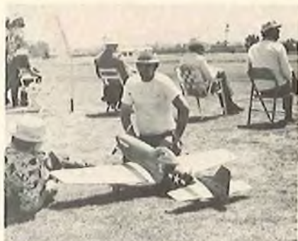
P-51 by Paul Cremins of San Jose, Calif. A Flite Glass fuselage with a scratch-built wing. The model uses a Kraft radio and an OS Max .60 motor.
