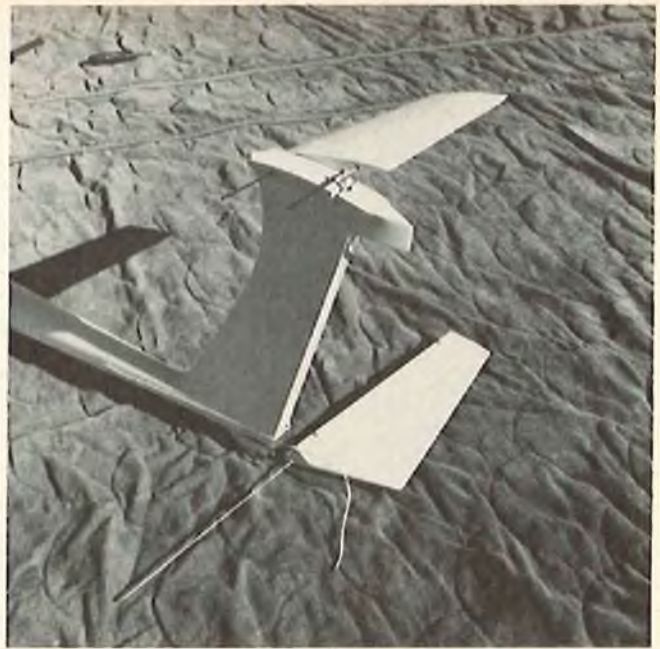
Tail Assembly. Rudder is removed by withdrawing 1/16" O.D. aluminum hinge pin from the base. "Missing Link" couples drag pin on the flying stab to the elevator pushrod.
