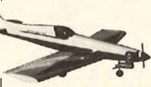
SUPER LUCKY FLY SUPREME New Fibreglas Fuselage-Wings covered with 1/64" plywood
