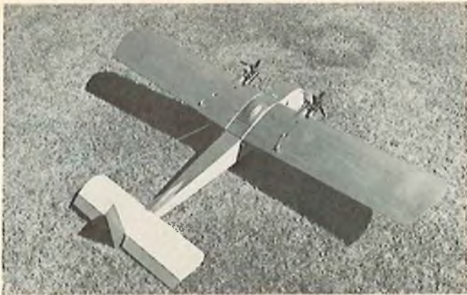
Wings separate just outboard of engines. Note offset couplings from aileron torque rods to ailerons on outer wing panels. Bump on top of wing center section contains throttle and aileron servos.
