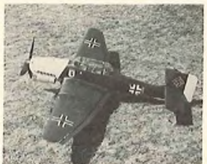
Junkers JU 87b-2 "Stuka" by Gene Ageno of Sunnyvale, Calif. The model uses an RS radio and an OS Max motor. The model dropped bombs.
