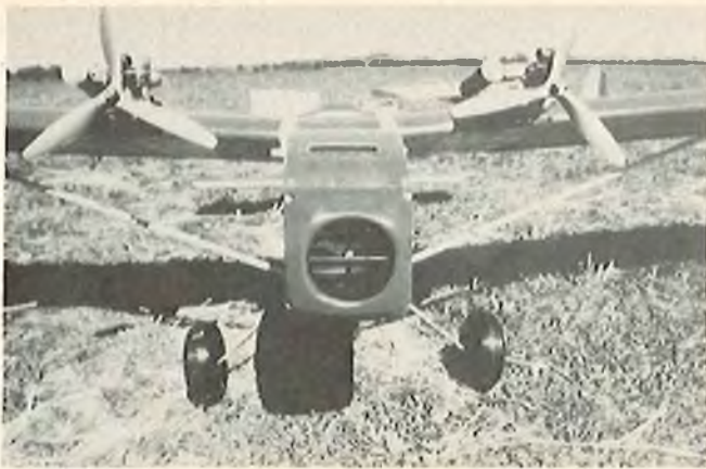
Front view of twin showing air intake and air volume counter. Contra-rotating props evident.
