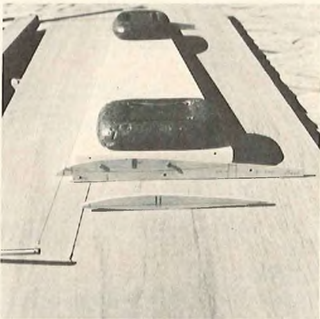
Cut the foam cores from 2 lb. density blue syntrofoam. Weight the blanks flat to the cutting board to insure against a twisted core.
