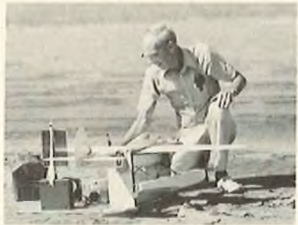
Art Snyder's Form I Shoestring Racer had a wing loading of 35 oz./sq. ft. and flew at about 100 mph. K & B .40 power.
