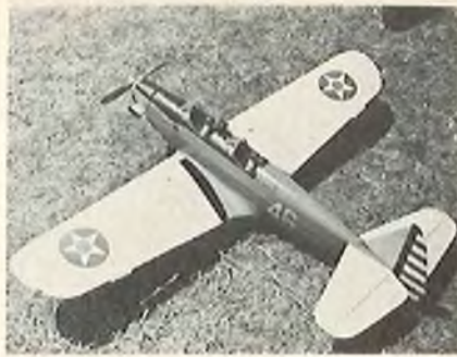
PT 19 by Lee Horn of Anahelm, Calif. A Jemco kit that was built in 12 days with about 50 hours of work. Power is a K & B .40 and control is a 7 channel Kraft.
