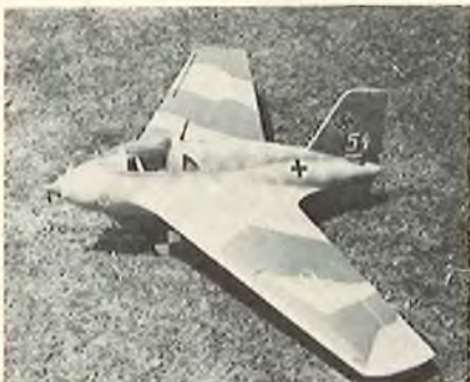
ME 163b Rocket plane by Pat White of Lauderdale Lakes, Florida. Powered by a Super Tigre .60 and controlled by a World Engines radio. It was 18 months in the works.
