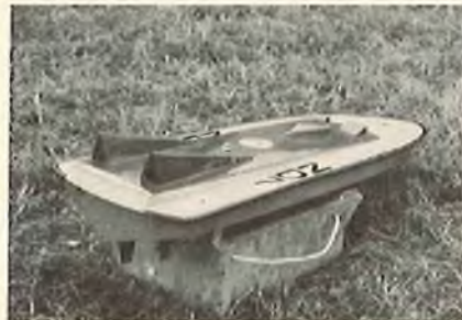
Same boat, this time showing air outlets.
