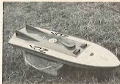
Front view of Deep V Racing hull showing close-fitting hatch and air intakes.
