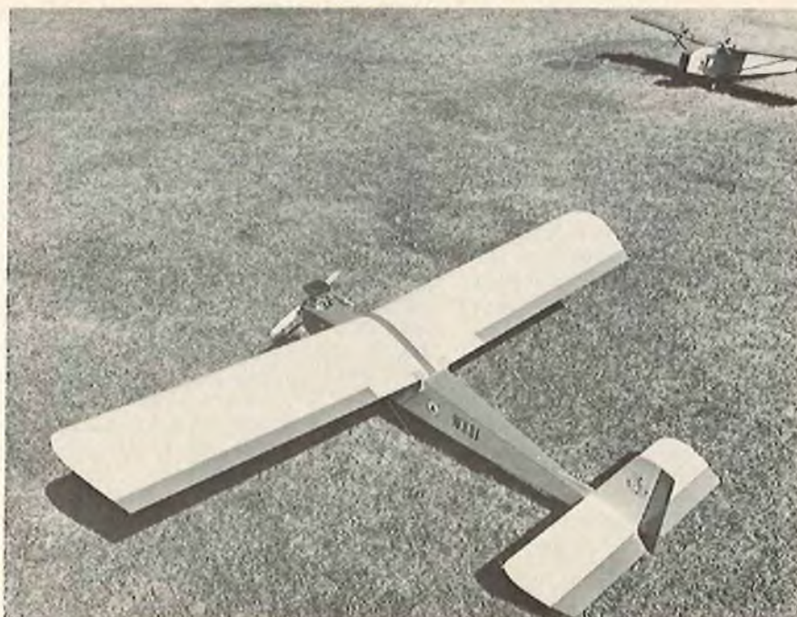
Standard Sr. Telemaster. I built it myself at home to get interest and prove the idea for scientific use. It holds camera. Shoots out left side through window under wing.
