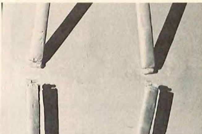
Wing attachments for struts using Robert hinge flats cut in half.
