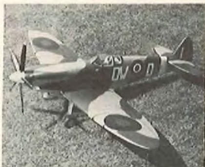
Spitfire Mk. 14 by Denny De Weese of Orange County, Calif. A Royal kit powered by an OS Max .60 and controlled by an Orbit radio. 300 hours of labor.
