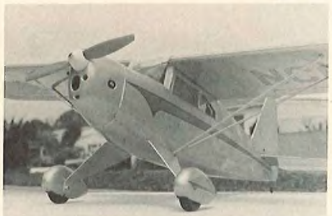
Note small wire protruding from cowl bottom for glow plug clip.
