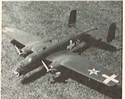
B-25 Mitchell by Pat Ray of Los Gatos, Calif. The only twin engine model at the meet, it is a Royal kit with K & B .40's and an EK radio.
