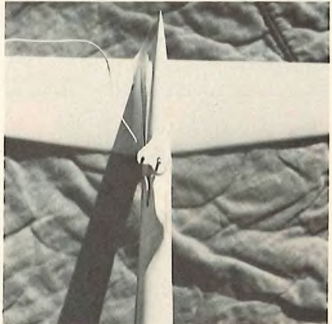
Access to the hinge pin is from the base of the rudder. Keep the gaps here as tight as possible.
