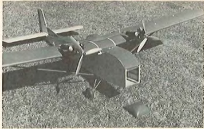
Twin with nose block removed. 4 x 4 inch, 16 inches deep payload compartment. Air Sampler will have 3 inch aperture, faired intake scoop. Air exits through "dust bin" type door in bottom. Doors operated by Sonic Systems air cylinders.
