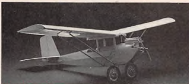
PIETENPOL SKY SCOUT (1/2-A 'PETE') • Span 42 in. • Area 284 sq. in. • Length 26 in. • Weight 22-27 oz. • Engine QRC .049 • Wing loading 11-14 oz./sq. ft. 26.95
