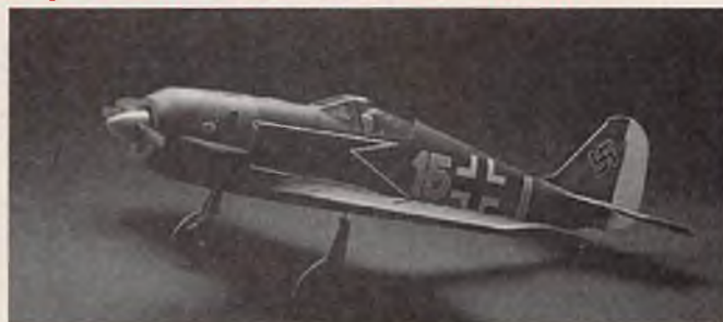
FOCKE-WULF FW 190-A3 • Span 36 in. • Area 216 sq. in. • Length 28.5 in. • Weight 22-28 oz. • Engine TD .049 • Wing loading 14.6-18.6 oz./sq. ft. 34.95
