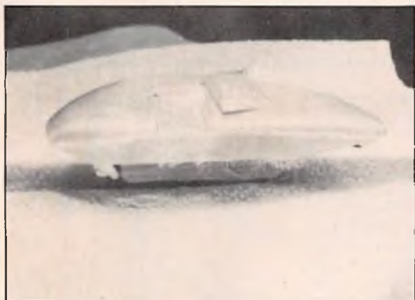
9.) Glass in place ready for resin.
