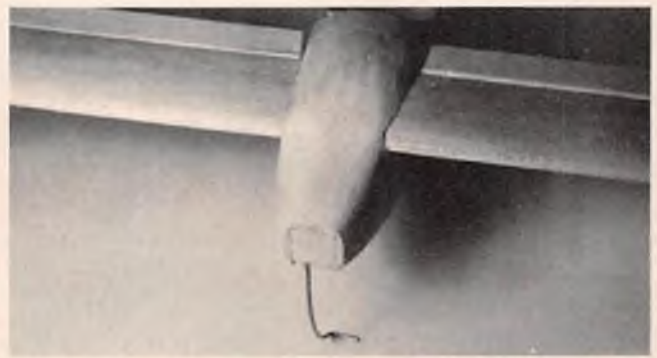
Nose blocks rough carved. Needs additional tip block and final filling and sanding.
