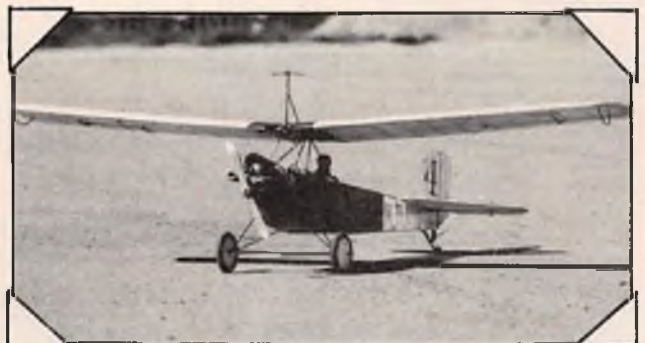
Prototype Parasol Antic, with upright engine and Williams Brothers wheels. Wide well placed gear makes ground handling easy.
