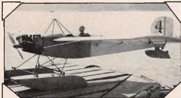
The Antic on floats — also available as a Proctor kit. This one has oak stained fuselage front end and floats.
