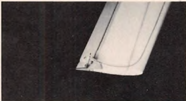
Rudder "kick-out" linkage shown with aileron cable hooked up.
