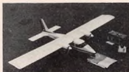
John Scrary's P-68 from Astro Flight kit. 5 channel, rudder, elevator, aileron, motor and flaps.
