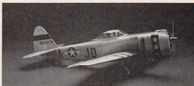
P-47 THUNDERBOLT • Span 36 in. • Area 216 sq. in. • Length 28.5 in. • Weight 22-28 oz. • Engine TD .049 • Wing loading 14.6-18.6 oz./sq. ft. 34.95
