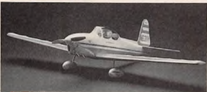
CHIPMUNK • Span 36 in. • Area 216 sq. in. • Length 28.5 in. • Weight 22-28 oz. • Engine TD .049 • Wing loading 14.6-18.6 oz./sq. ft. 34.95
