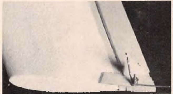
Aileron horn and rudder "kick-out" linkage. Linkage on both tips on bottom side.
