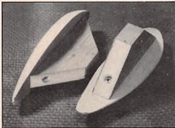
7.) Holding blocks attached. Note shape.
