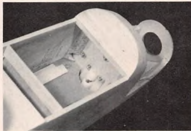
Tank compartment showing Goldberg nylon bearing block and groove to clear steering arm.
