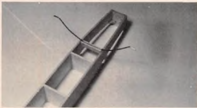
Landing gear sandwiched between two pieces of plywood.
