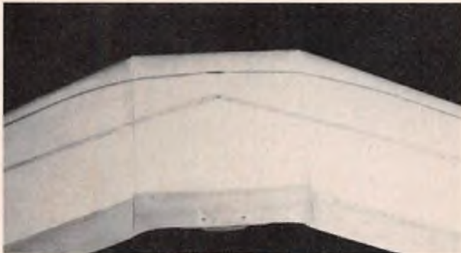
Six inch center section of Ace constant chord wing shows spar, trailing edge and Sullivan Gold'N-Rod and cable installed.
