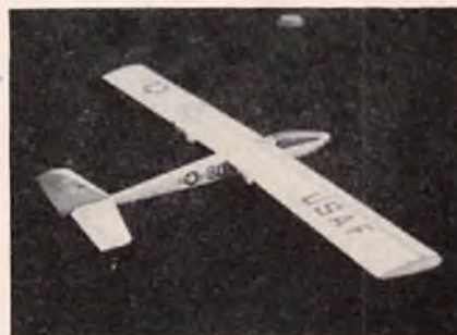
Jim Zaremski's Sweepstake twin 05. 54 oz., 74" wingspan, 580 sq. inches of wing area. A Floater.
