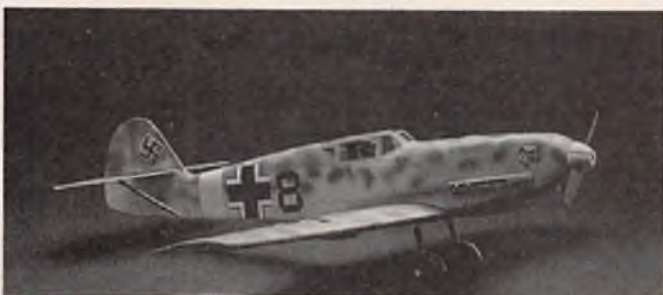
ME-109E • Span 36 in. • Area 216 sq. in. • Length 28.5 in. • Weight 22-28 oz. • Engine TD .049 • Wing loading 14.6-18.6 oz./sq. ft. 34.95
