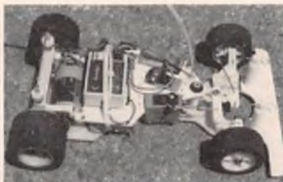
Curtis' Associated RC12E Production car featured the lightweight conversion parts and the new super fast Bantam Midget servos from Novac Electronics.
