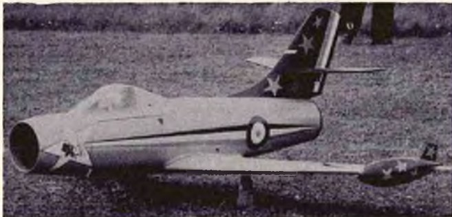
Marcus Norman's O/D Ouragan. DIY fan/duct, Rhomairs. Unflown due to engine snags. Looks pretty. Balsa/ply structure.
