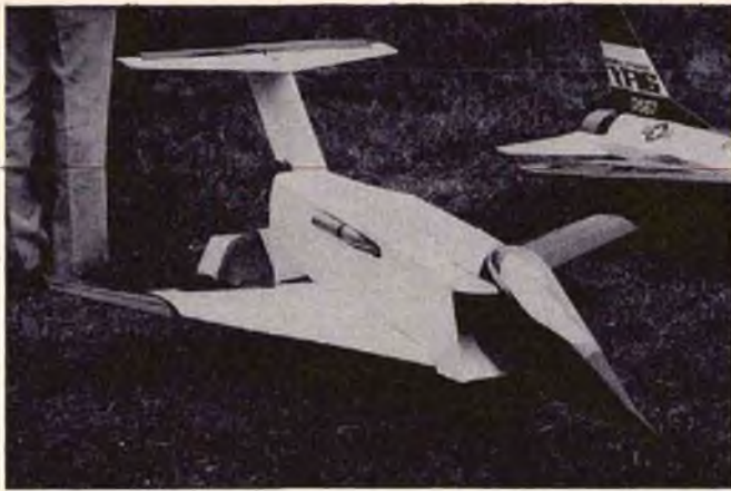
Ducted Fantasia in the shape of Adrian Hayward's Captain Scarlet Interdictor. Axiflo 40. Not finished. Balsa/ply/solarfilm.
