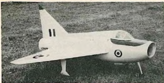
Flt. Lt. Harry French's Boulton Paul P111 research Delta. All foam/veneer construction. Engine snags prevented flying. DIY fan/duct, KB SRII.
