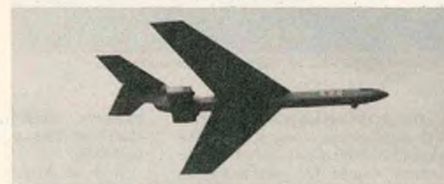
Ken Stokes' Twin-Jet. DIY fan/duct, 2 x OPS 15. Entertaining performer, balsa/ply structure.
