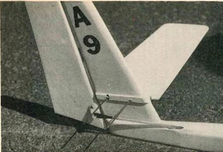
Aft fuselage view showing rudder controls and flying stab control details.
