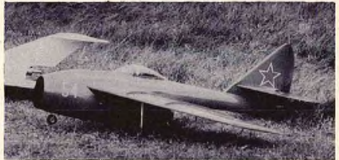
LA 160 by Ken Stokes. DIY fan, O/D model, 6' take-off run into endless vertical climb. KB SR11 on mini-pipe. Shattering performer in all respects. Fiberglass fuz, foam/veneer wings.
