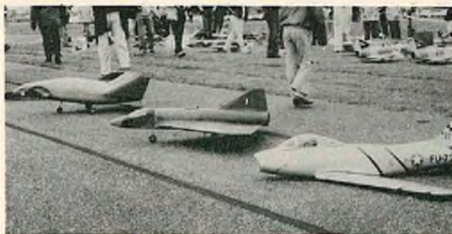
Graham Dennett's freelance Axiflo 20 powered Delta 1000 parked between unflown Dyna Soar and F86. Graham's 5½ lb., KB 21 — powered model equalled most 40-powered jobs in performance.
