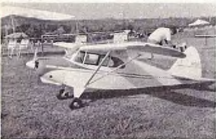
Piper Pacer, 1/3 scale, built by Dale Martin, Columbia Station, Ohio. Tartan twin ignition, flaps, 31 lbs., finished with Coverite and dope. Super flier.
