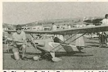
C. Cheeks, Buffalo, Texas, and his 50% Pober Pixy. 70cc Hornet for power swinging a 24" x 10" prop. Flew exceptionally well.
