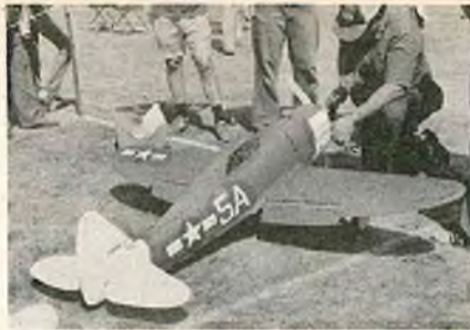
Prototype of Byron Originals' new P-47D. Fiberglass fuselage and foam wings and tail. To be released soon.
