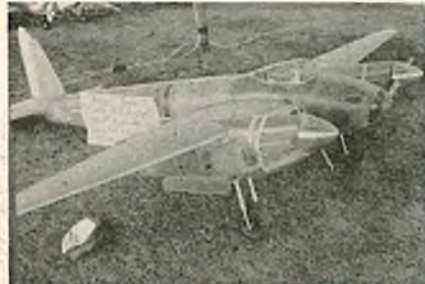
Partly finished Mosquito Bomber 1/5 scale — 40 lbs. with two geared Webra .61's. By Larry Scott, Kirkman, Iowa.
