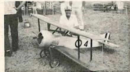
Rusty Allen, Logo Vista, Texas, with his Balsa USA Sopwith Pup. With a 108" span, a Kioritz up front, it weighs 28 lbs. Rusty uses a Futaba radio.
