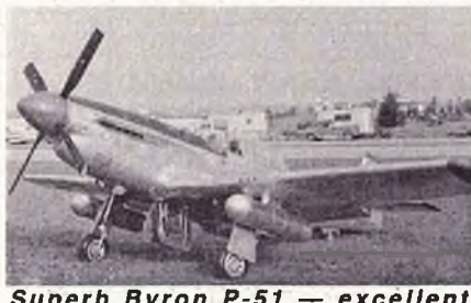
Superb Byron P-51 — excellent workmanship. Built by Rick Quinlan and owned by Steve Wood of Decater, Illinois. Fuel tanks on wings are actually air tanks for the retracts.
