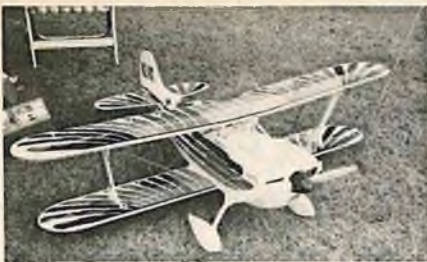
Ed Sochor, Ft. Worth, Texas, built this Christen Eagle. Spans 65", weighs 18 lbs., powered by Tartan Twin and uses a Futaba radio.
