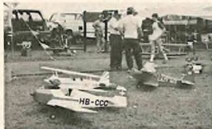
Chuck Cunningham, Ft. Worth, Texas, showing his 84" Turbulent at 11 lbs. with O.S. .90 and JR radio. In background is Lazy Ace, 76" span, Webra 90 at 11½ lbs. with EK radio.
