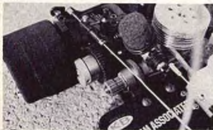
Because of the long straightaway, Associated developed an automatic 2 speed transmission for the team. The transmission shifts for 6 to 1 to 5 to 1 at about 25,000 rpm.
