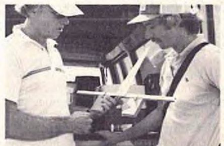
Chuck Shade (left) and home-made wing incidence meter. Extremely accurate using "plumb bob" angle measurement.
