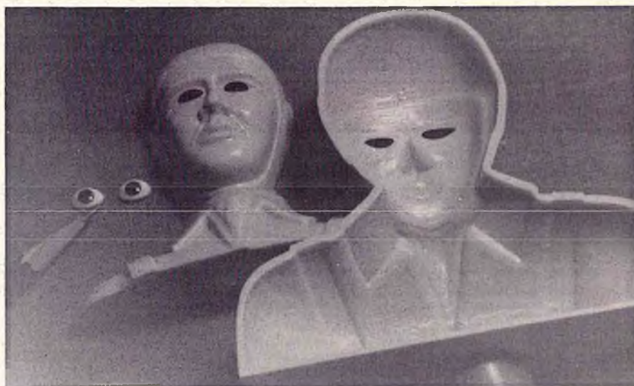
Both "pilots" with their plastic eyes "opened." Pencil points to 8 mm doll's eyes to be used in the quarter-scale pilot. Note how the plastic has been scraped away in the larger casting --- to provide realistic eyelid thickness.
