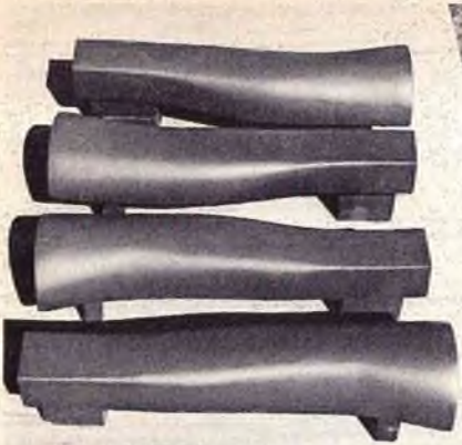
Inlet duct plugs after waxing.
