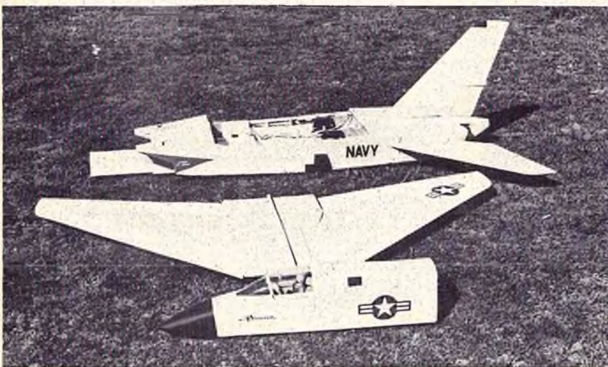
Major components disassembled for transportation.
