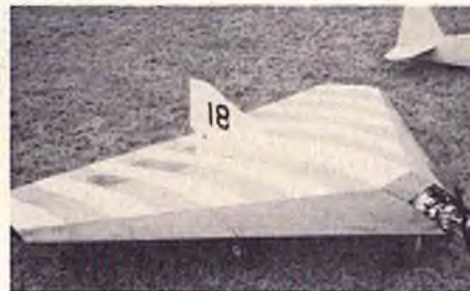
Bob Brooks, Houston, Texas, had this Quadra powered Delta with 86" span, 18 lbs. and Kraft radio.
