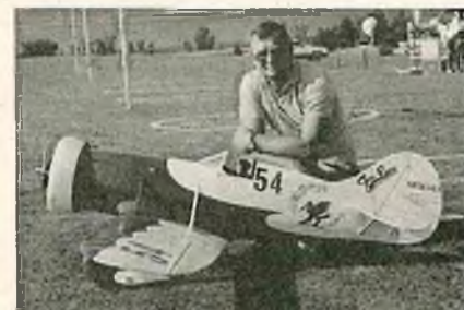
Bill Hunchis, Minneapolis, Minnesota, and Gee Bee Sportster Model Y — scratch-built, 17 lbs., O.S. .90, 16/6 prop.
