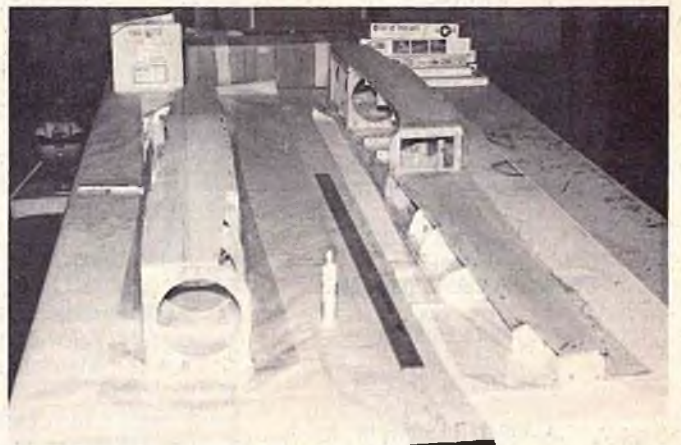
Fuselage halves after side skin has been added.
