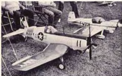
Kerry Hunt, Lake Jackson, Texas, brought two. A 92" span Corsair at 32 lbs. with Quadra on prop drive. Also his CAP 21 with 80" span at 16½ lbs. with Quadra. Both had Kraft radios.
