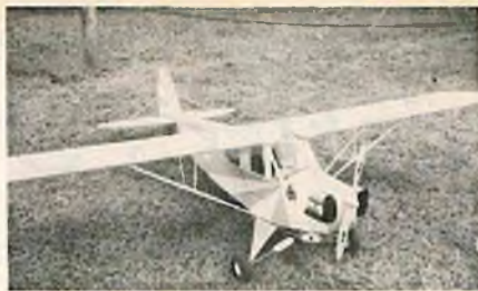
Larry Jensen, Ft. Worth, Texas, displayed his Clipped Wing Cub. Wingspan 86½" with a Webra 90 and weighing 12½ lbs. Larry used Kraft equipment.
