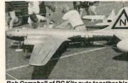
Bob Campbell of RC Kits puts together his giant B-29 Superfort. 17 ft. wingspan, 145 lbs., (4) 2.4 cu. in. Kiorlitz engines. It crashed later in the week.
