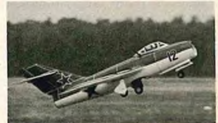
An OPS 65 hauls Kenneth Shufelt's MIG 15 up at a good angle. From the Byron kit, the model was one of five ducted fan models of jet aircraft flying in the Sportsman Sportscale event.
