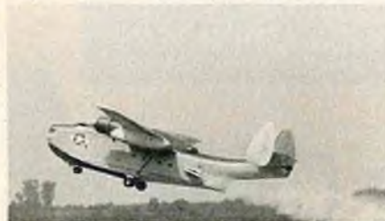
John Nicolai attached wheels to his PBM-3 seaplane and made some spectacular take-offs using Estes rockets for a realistic Jato assist. Powered by two ST 71 engines, the PBM-3 was one of the largest models and the only multi-engined model to fly in Giant Scale.
