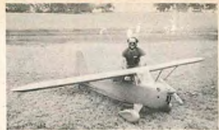
Mike Pugh, Orange, Texas, with his 144" Rearwin Speedster at 38 lbs. and using a 3.5 Kawasaki. Mike uses a Kraft radio.
