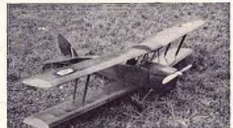
Warren Garoutte, Randolph AFB, San Antonio, Texas, brought his 66" span Tiger Moth. Powered by O.S. .60 4-stroke at 7½ lbs., is guided by a Futaba radio.
