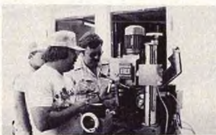
A very busy part of the pit area was this lathe/mill which was used to make parts and also true tires as Rich Lee, Rich Potempa and Rick Davis are doing.
