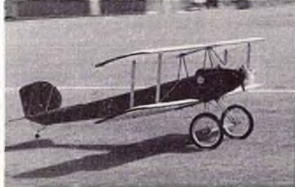
Two times size Antic bipe on take-off. 12" bicycle wheels with Heath parasol landing gear. Phil Kling, Oxnard, California.
