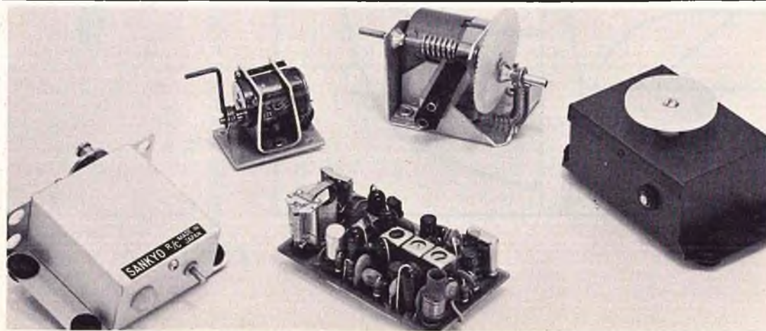
Relay single channel version of RCM's convertible Superhet along with several motorized actuators. L to R: Sanyo compound servo; Tomoser proportional rudder actuator; new S.E.P. Go-Ac for Galloping Ghost; Royal compound servo.
