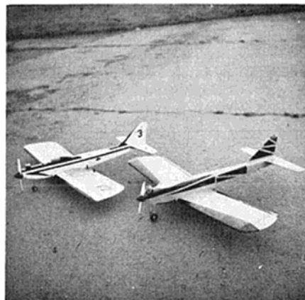
Two speed machines—Geff and Maurice Franklin's Pylon Dusters. Bird in foreground uses Oliver Tiger 15. Orbit gear in both.
