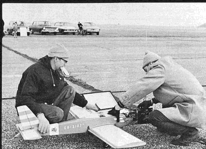
Right: Geoff Pike gives his latest model a quizzical look before starting up. Taurus wing, original fibreglass fuselage and neat "Plane Jane" insignia on the fin. Note silencer on the Super Tigre. F and M proportional gear.
