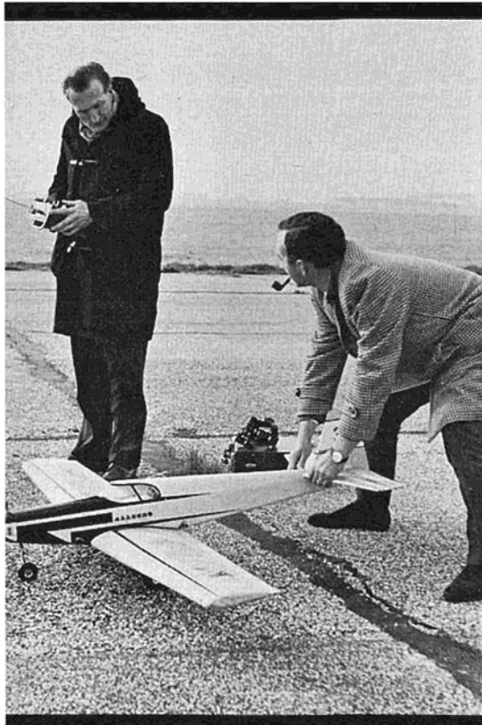
Right: Geoff Pike gives his latest model a quizzical look before starting up. Taurus wing, original fibreglass fuselage and neat "Plane Jane" insignia on the fin. Note silencer on the Super Tigre. F and M proportional gear.
