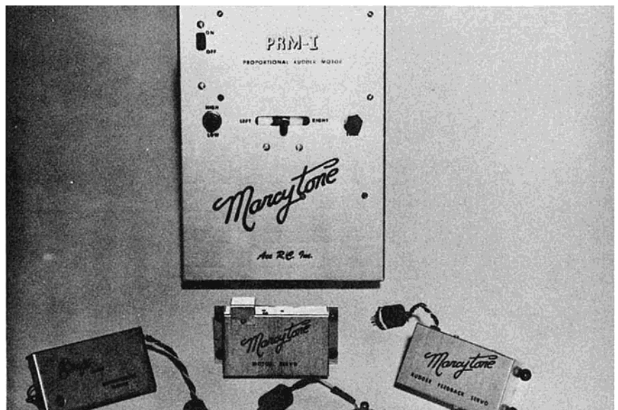
Marcy PRM-1 proportional system with Kraft superhet receiver.
