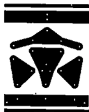
Printed circuit board for Marcy superhet conversion. Actual size.
