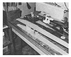
Join sides together with bulkheads.
