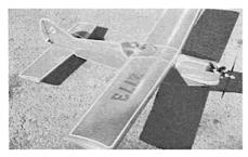
Fearless Leader's TD .049 powered Midwest-RCM Goodyear racer. This modified Owen Kampen design uses Airtrol's RE-1 on rudder-elevator.
