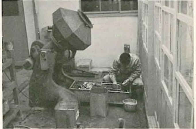
Here, engine parts are polished in a giant tumbler.
