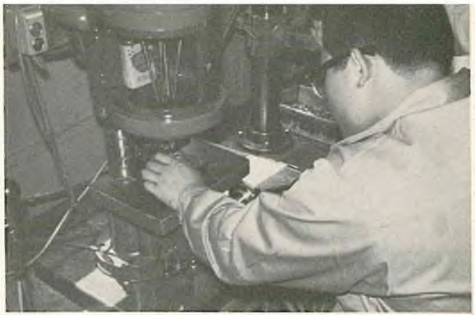
All the rear crankcase holes are drilled and tapped simultaneously for the O.S. .50 on this specially designed machine.
