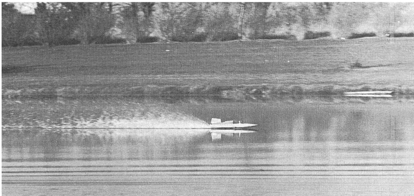
Ron Buck's Rossi-powered White Heat 60 during a test run at Lombard, Illinois. Boat features a surface prop and proportional R/C for steering and throttle. Ron is testing a new hull, new proportional system, new props, and new fin placement. Maybe a record in the making?
