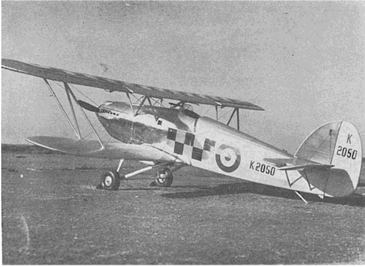
Top honors this month goes to D. F. Bryant of London's Bromley R/C Club for his 54" Hawker Fury. This eight and a half pound scale ship uses a Merco 61 for power. F&M radio equipment with Bonner servos. Front part of the fuselage is of fibreglass with chrome vacuum plating. Markings are from R.A.F. Squadron No. 43. A magnificent ship.
