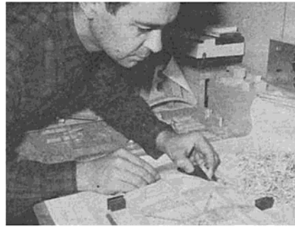
Block plane used to finish wing tip to cross section.
